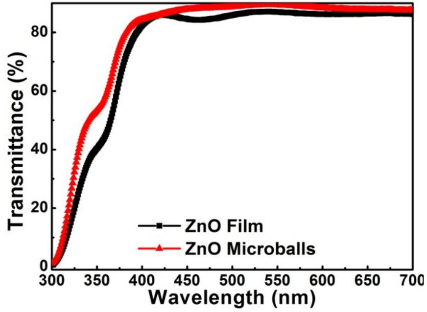
**Figure S11** The transmittance of ZnO film and micro-balls on FTO substrate.
