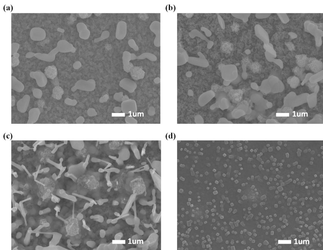
**Figure S3** The top view of SEM images of all-inorganic perovskite CsPbBr<sub>3</sub> prepared from different concentration of PbBr<sub>2</sub> film: (a) 0.5M, (b) 0.75M, (c) 1.25M, and (d) 1.5M.
