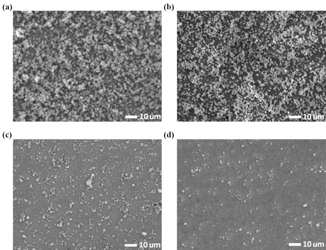
**Figure S1** The top view of SEM images of ZnO microspheres with different times dilution: (a) 5 times, (b) 6 times, (c) 7 times, (d) 8 times.
