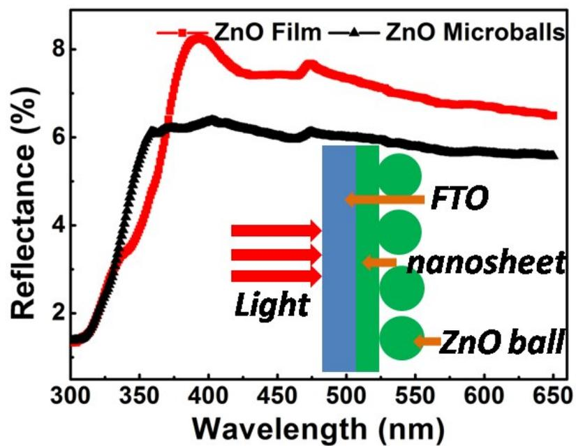
**Figure S10** The reflectance of ZnO film and micro-balls on FTO substrate. Insert: light transmission for testing illustration.
