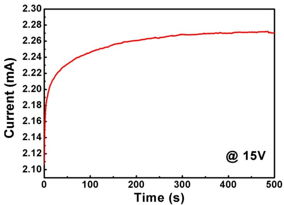
**Figure S9** The stability of ZnO/CsPbBr<sub>3</sub>/GaN structure devices under the forward voltage at 15 V for 5 min.
