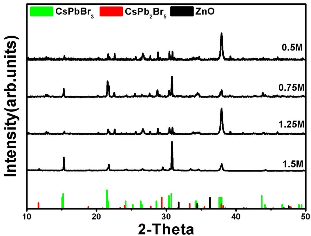
**Figure S4** The XRD pattern of all-inorganic perovskite CsPbBr<sub>3</sub> prepared from various concentration of PbBr<sub>2</sub> film.
