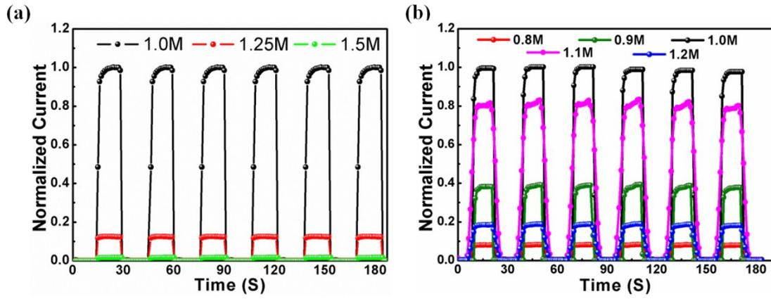
**Figure S6** The light response characteristic of ZnO/CsPbBr<sub>3</sub>/GaN structure devices, where CsPbBr<sub>3</sub> films were prepared from different concentration of PbBr<sub>2</sub> film: (a) 1.0M, 1.25M, 1.5M and (b) 0.8M, 0.9M, 1.0M, 1.1M, 1.2M.
