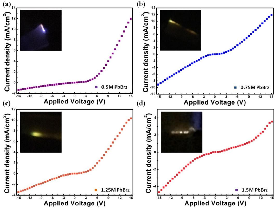
**Figure 7** I-V characteristics of the LED device based on the heterojunction ZnO/CsPbBr<sub>3</sub>/Ga<sub>N</sub>, where CsPbBr<sub>3</sub> films were prepared from different concentration of PbBr<sub>2</sub> film: (a) 0.5M, (b) 0.75M, (c) 1.25M and (d) 1.5M. The Insert is the photo taken from the corresponding device under a forward bias voltage of 15 V.
