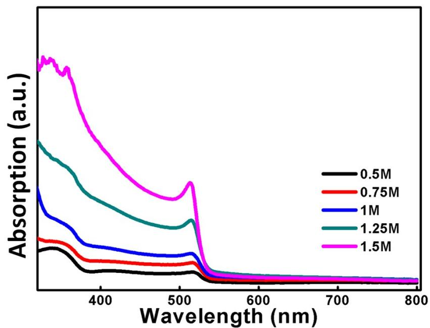
**Figure S5** The absorption spectra of all-inorganic perovskite CsPbBr<sub>3</sub> prepared from various concentration of PbBr<sub>2</sub> film.
