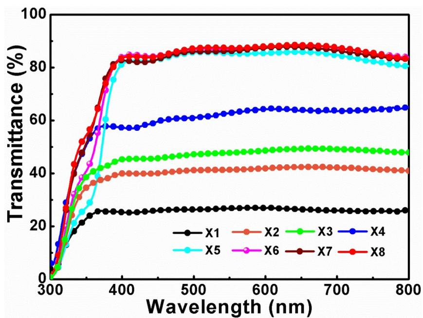
**Figure S2** Transmittance of the ZnO microspheres with different times dilution.
