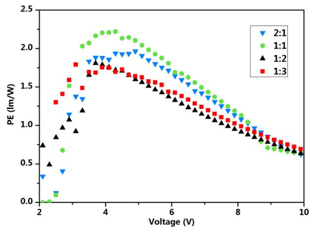
Figure S5. PE-voltage characteristics of OLEDs based on hybrid HILs with different volume ratios of  $\text{WO}_3$  to PANI: PSS (2:1, 1:1, 1:2, 1:3).
