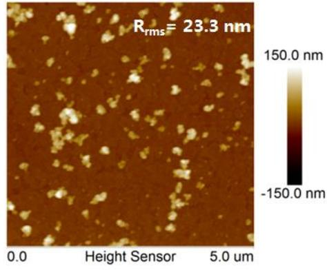
Figure S3. AFM height image of ITO/ $\text{WO}_3$  layer.
