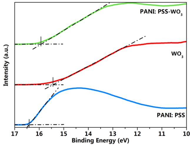
Figure S4. UPS spectra showing high-binding energy secondary electron cut off of  $\text{WO}_3$ , PANI: PSS, PANI: PSS- $\text{WO}_3$ .
