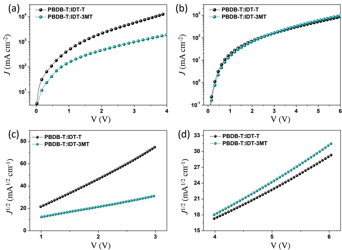
**Fig. S5** Space-charge-limited current  $J$ - $V$  characteristics and corresponding  $J^{1/2}$ - $V$  plots of the blend films under dark conditions for (a), (c) hole-only devices and (b), (d) electron-only devices.
