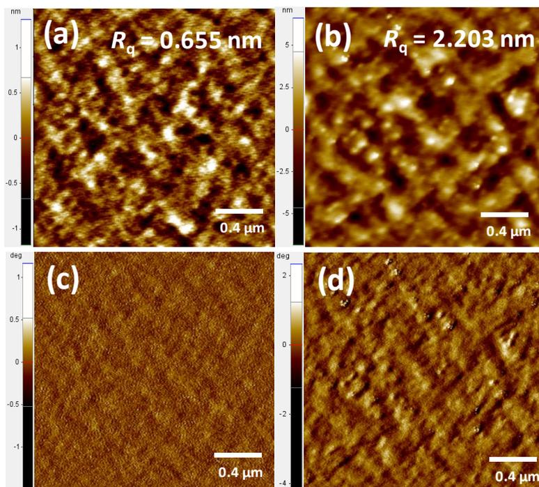
**Fig. S6** AFM (a,b) height images and (c,d) phase images ( $2\ \mu\text{m} \times 2\ \mu\text{m}$ ) of the optimized PBDB-T:IDT-3MT blend films (1:1 w/w) prepared in chlorobenzene. (a,c) PBDB-T:IDT-3MT without additive and (b,d) PBDB-T:IDT-3MT with 1 vol% DIO.
