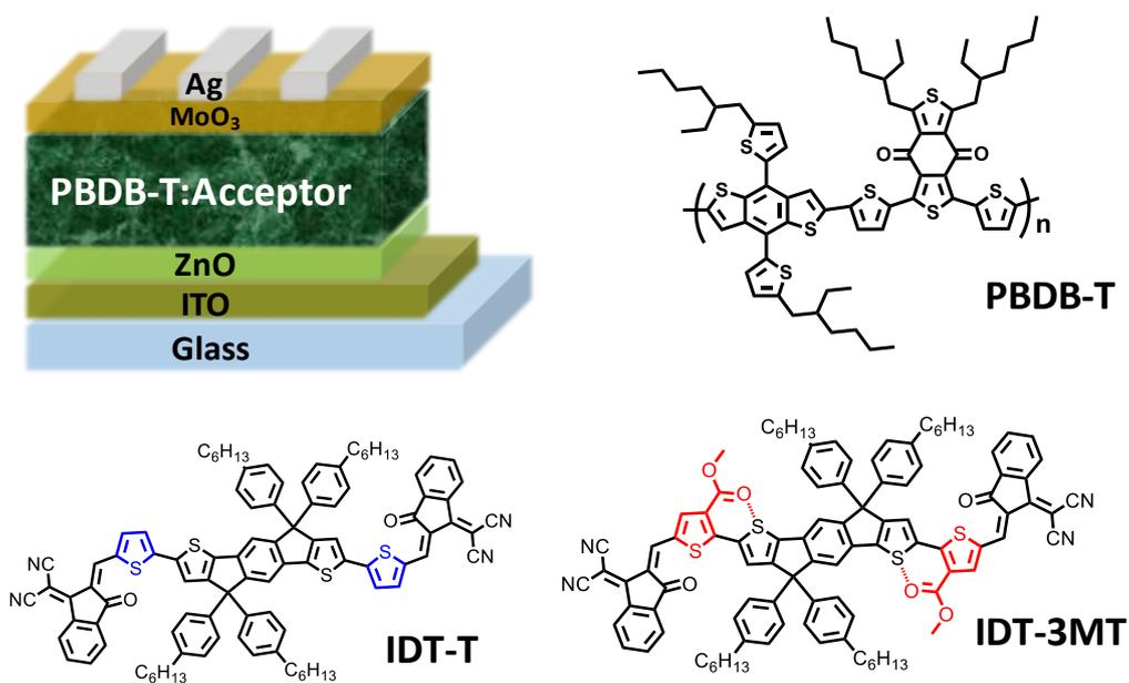
**Fig. S3** Chemical structures of the donor polymer and acceptors. Device configuration of the inverted structure PSCs.
