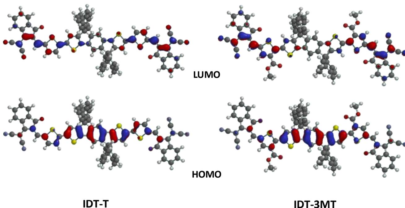
**Fig. S1** Optimized molecular geometries and frontier molecular orbitals of **IDT-T** and **IDT-3MT** by DFT calculations.
