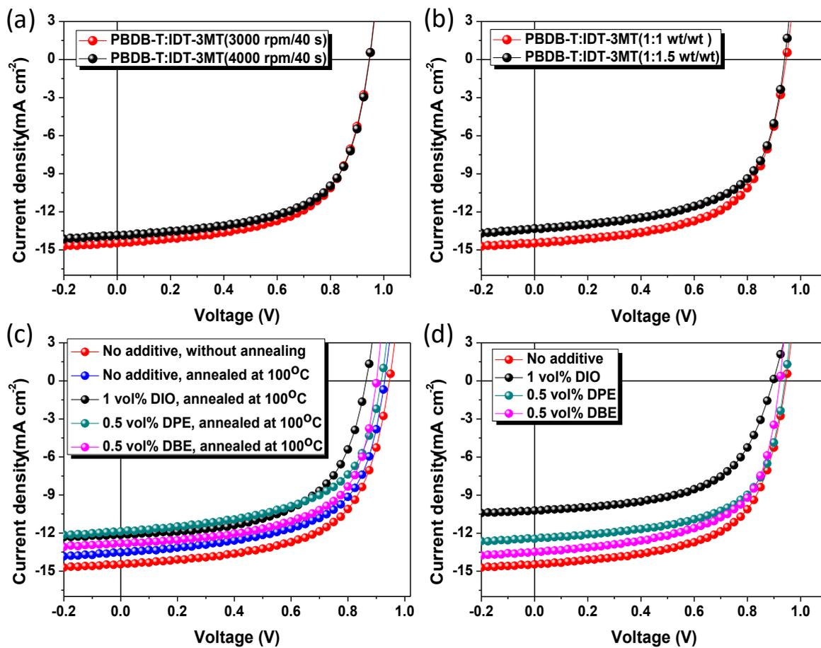
**Fig. S4**  $J$ - $V$  characteristics of IDT-3MT-based PSC devices under various conditions: (a) effect of thickness, (b) effect of ratio, (c) effect of solvent additive with annealing and (d) effect of solvent additive without annealing. (DIO : 1,8-diiodooctane, CB : chlorobenzene, DPE : diphenyl ether, DBE : dibenzyl ether).
