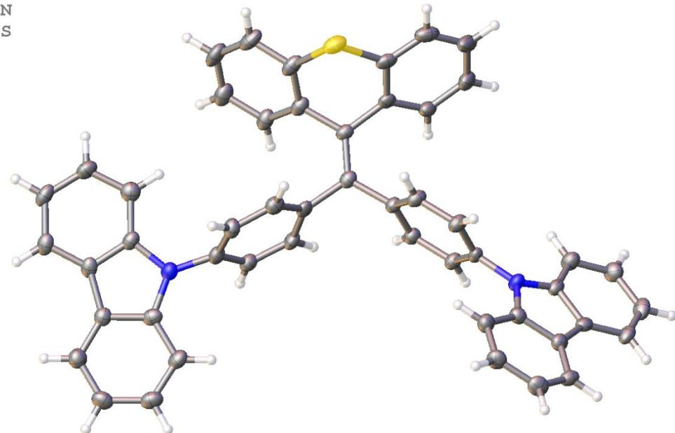
**Figure S13.** Thermal ellipsoids drawing of sulfur-bridged TPE derivative **1**.
