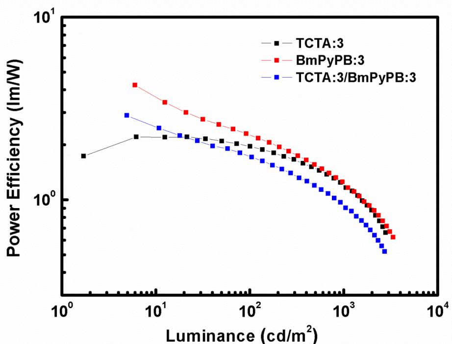
**Figure S18.** Power efficiency *versus* luminance curves of the doped OLEDs based on sulfur-bridged tetraphenylethylene derivative **3** as dopant, device configuration: ITO/MoO<sub>3</sub> (10nm)/NPB (40nm)/TCTA (10nm)/EML (10nm)/BmPyPB (40nm)/LiF (1nm)/Al.
