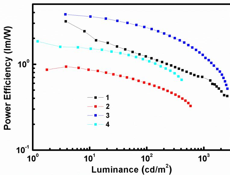
**Figure S17.** Power efficiency *versus* luminance curves of the non-doped OLEDs based on sulfur-bridged tetraphenylethylene derivatives **1-4** as emitters, device configuration: ITO/MoO<sub>3</sub> (10nm)/NPB (40nm)/TCTA (10nm)/EML (10nm)/BmPyPB (40nm)/LiF (1nm)/Al.
