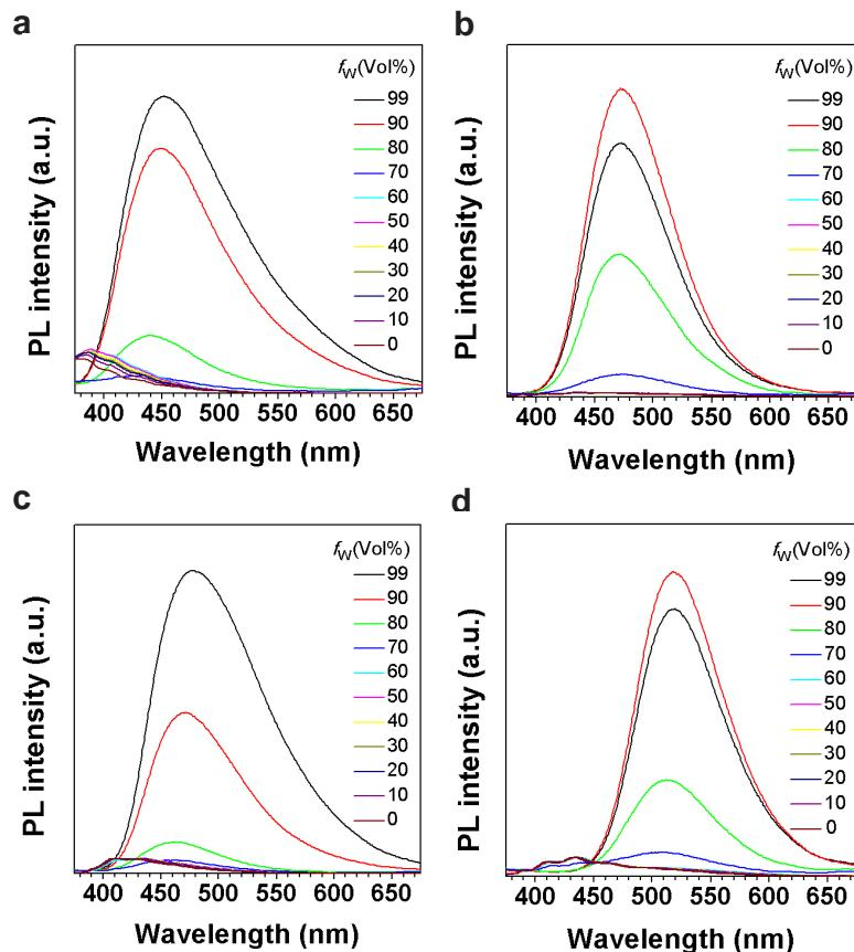
**Figure S16.** (a) **1**, (b) **2**, (c) **3**, (d) **4** AIE curves of sulfur-bridged tetraphenylethylene derivatives **1-4** in THF/H<sub>2</sub>O mixtures ( $10^{-5}$  M) with different water fractions ( $f_w$ ).
