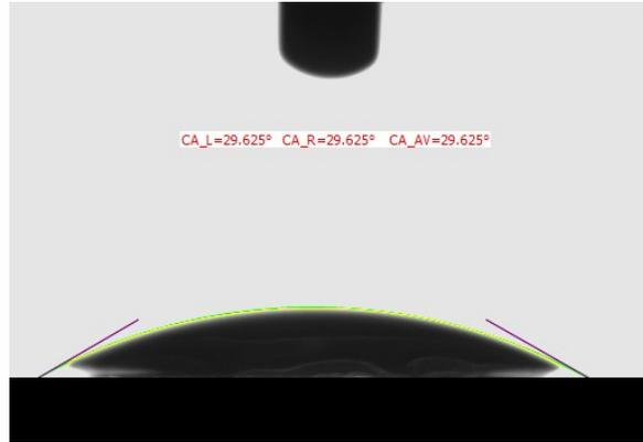
**Fig. S7** Viscosity and contact angle of Cuf-PDA.
