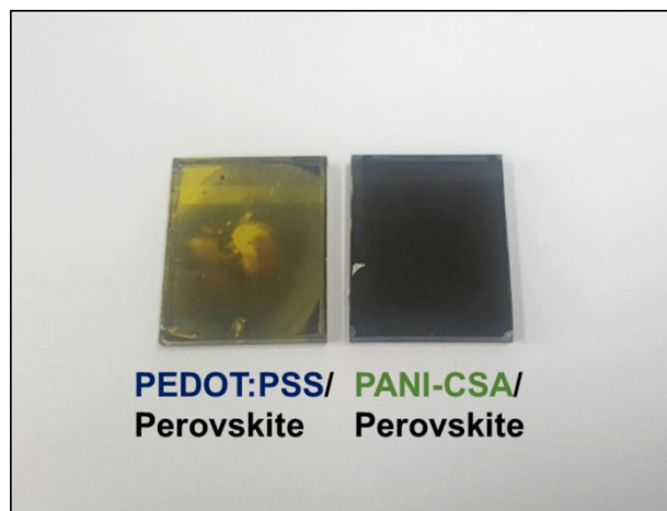
Figure S12. Digital photograph of perovskite films deposited on PEDOT:PSS and PANI-CSA which are stored for 7 days in ambient air (temperature = 25 °C, relative humidity = 50%). Photograph was taken from the glass side of the sample (glass/FTO/PEDOT:PSS or PANI-CSA/perovskite).
