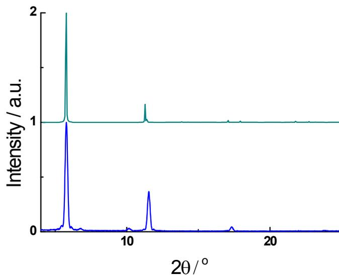
**Figure S9.** Experimental (blue line) and theoretical with preferential orientation along the  $\langle 100 \rangle$  direction (green line) X-ray diffractograms of the  $\text{AF}_2\text{PbBr}_4$  structure in the thin films.
