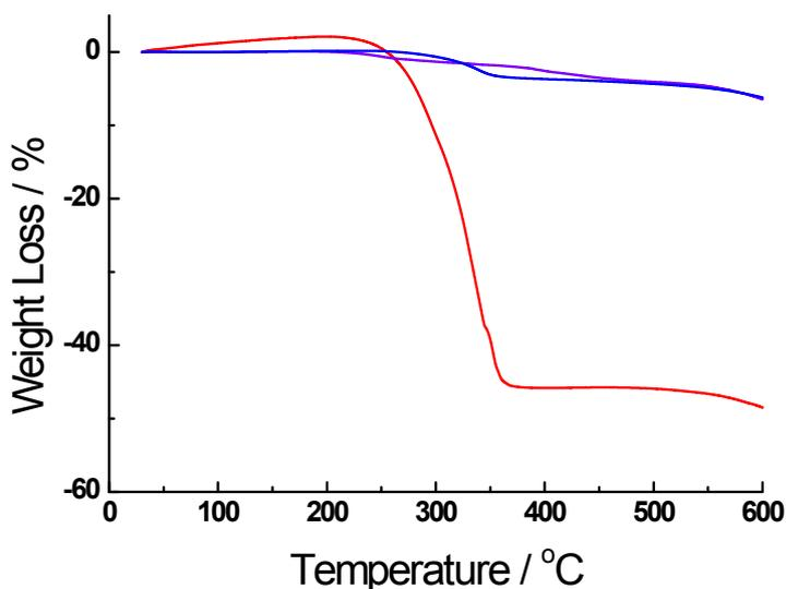
**Figure S1.** Thermogravimetric analysis (TGA) curves of the synthesized powders with AF (red line), AA (violet line) and DAF (blue line).
