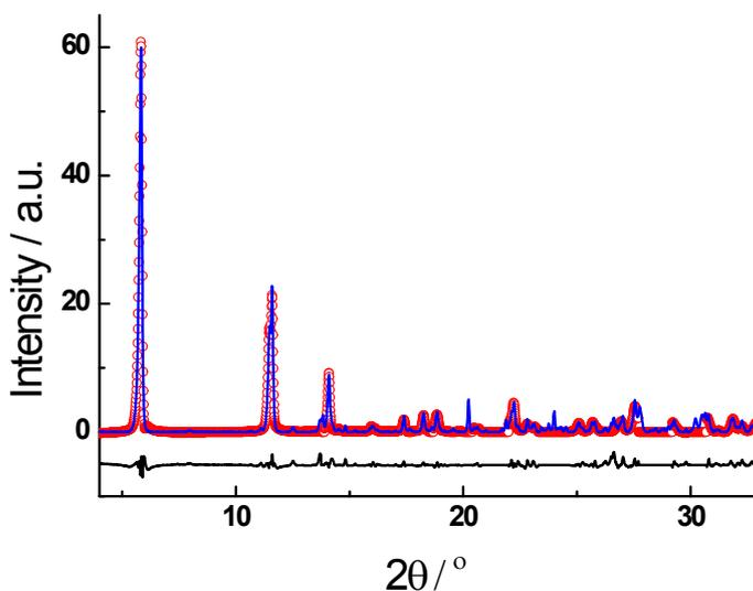
**Figure S2.** Rietveld refinement of the XRD pattern of  $(\text{AF})_2\text{PbBr}_4$ .
