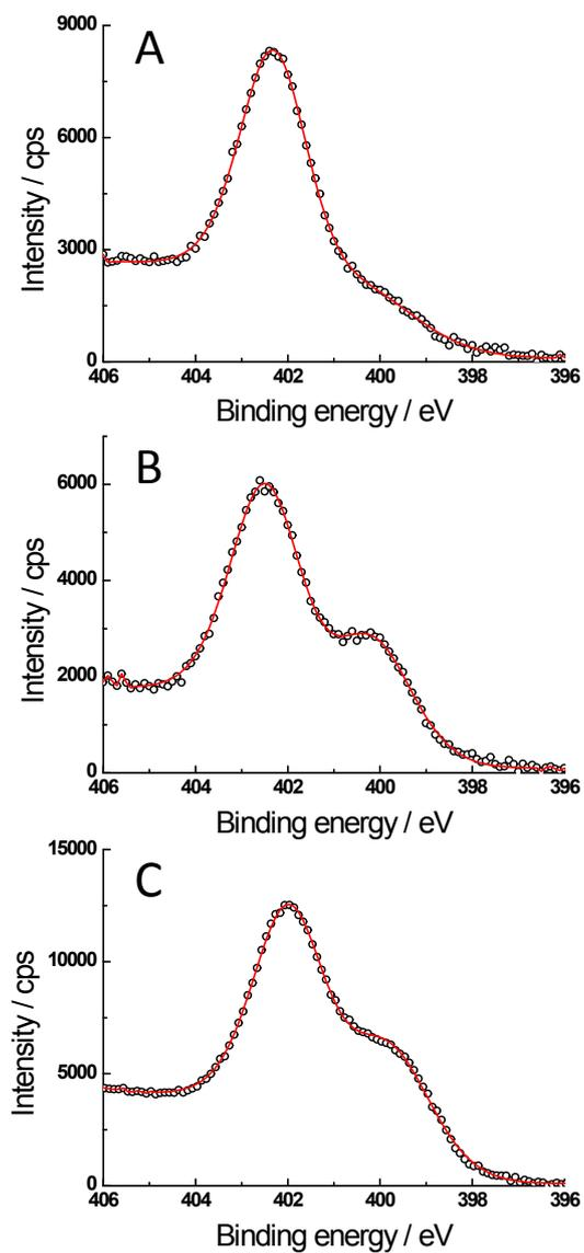
**Figure S4.** XPS spectra of N 1s of the synthesized powders with 2-ammonium fluorene (A), 2-ammonium anthracene (B), and 2,7-diammonium fluorene (C) cations.
