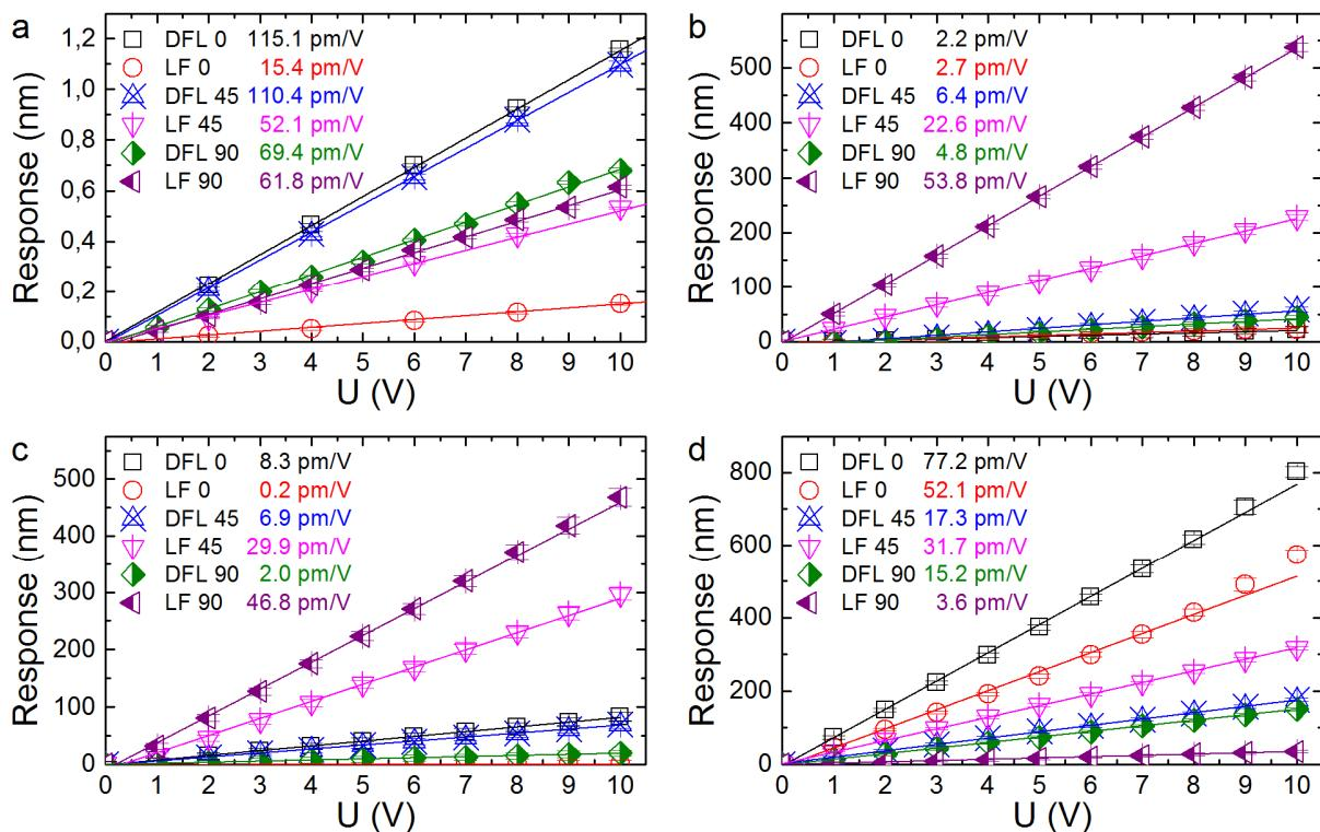
**Figure S26.** Voltage dependencies of piezoelectric response of (a) ( $S, S_P$ )-3a crystals, (b) ( $S, S_P$ )-3b crystals, (c) ( $S, S_P$ )-3d crystals, and (d) ( $S, S_P$ )-3f crystals.
