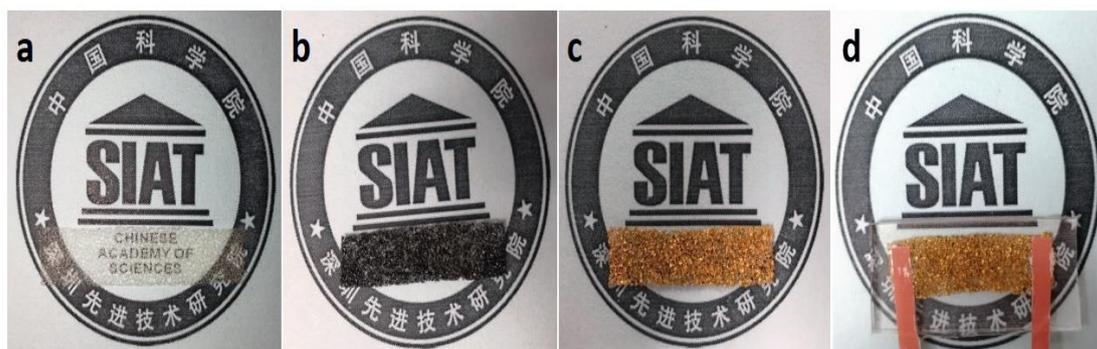
**Fig. S1.** The optical images of the a) as-prepared PUS, b) GPUS, c) Au-Ni@GPUS, d) the flexible conductor, respectively.
