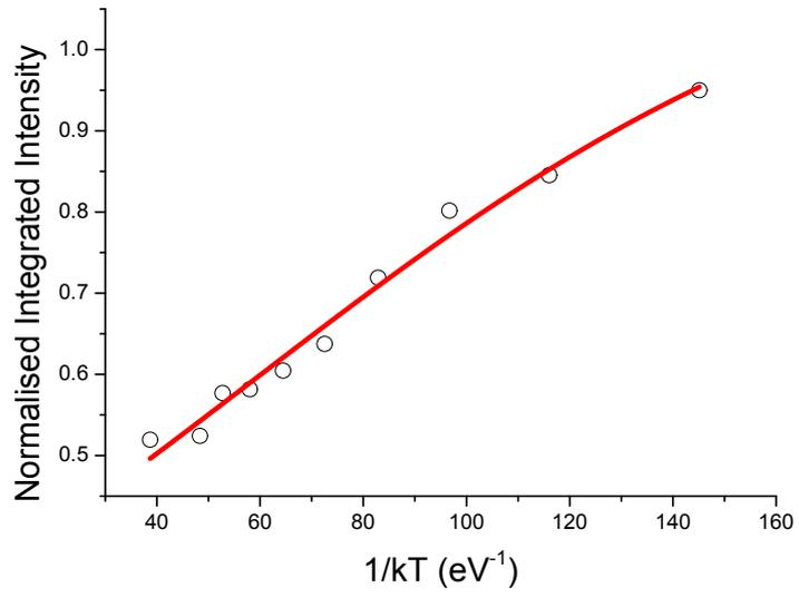
**Figure S14:** Arrhenius plot for the  $\text{Ge}_{1-x}\text{Sn}_x$  nanowires with  $x = 0.09$  at low temperature. The red line represents the Arrhenius fit, which gave an activation energy of  $E_A = 16$  meV.
