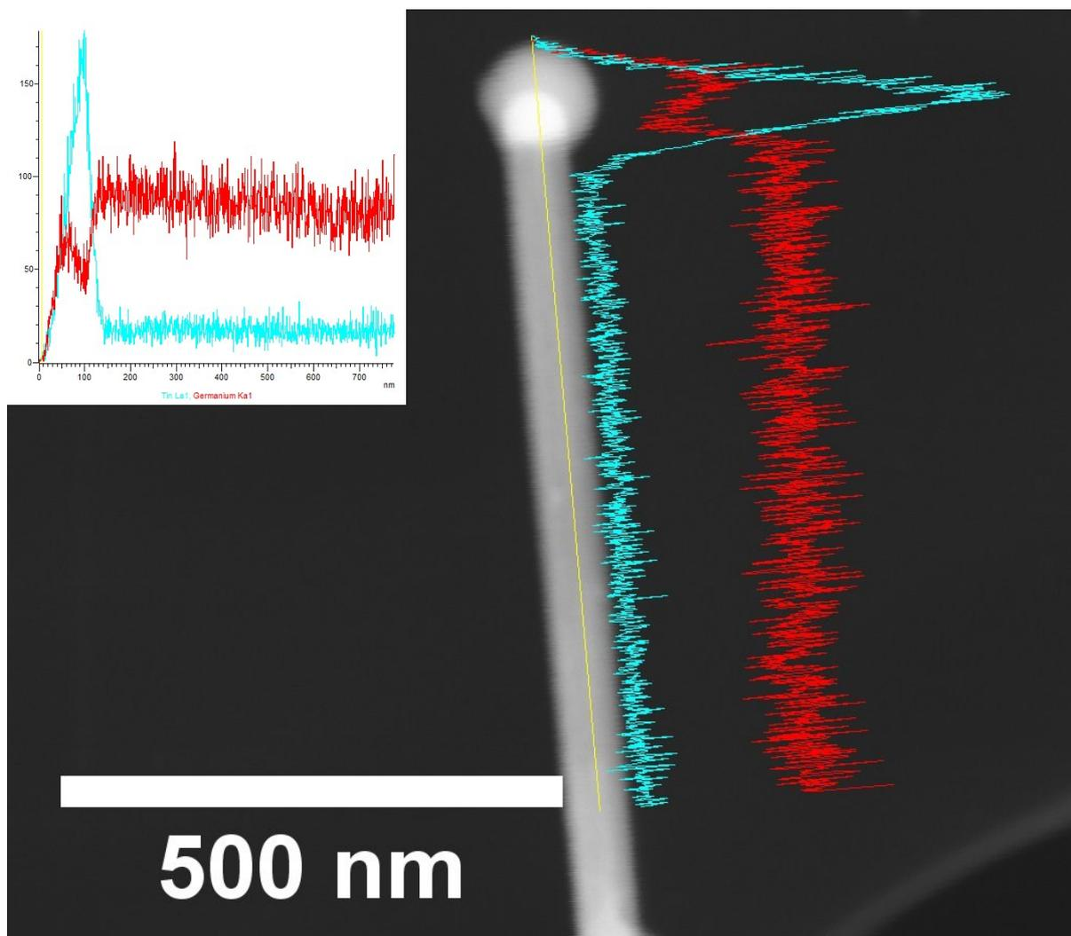
**Figure S5:** Linescan of EDX analysis of  $\text{Ge}_{1-x}\text{Sn}_x$  nanowires with mean Sn content 8.7 at. %. In the linescan Ge is denoted by red and Sn by blue. The Sn rich nature of the seed is clearly apparent.
