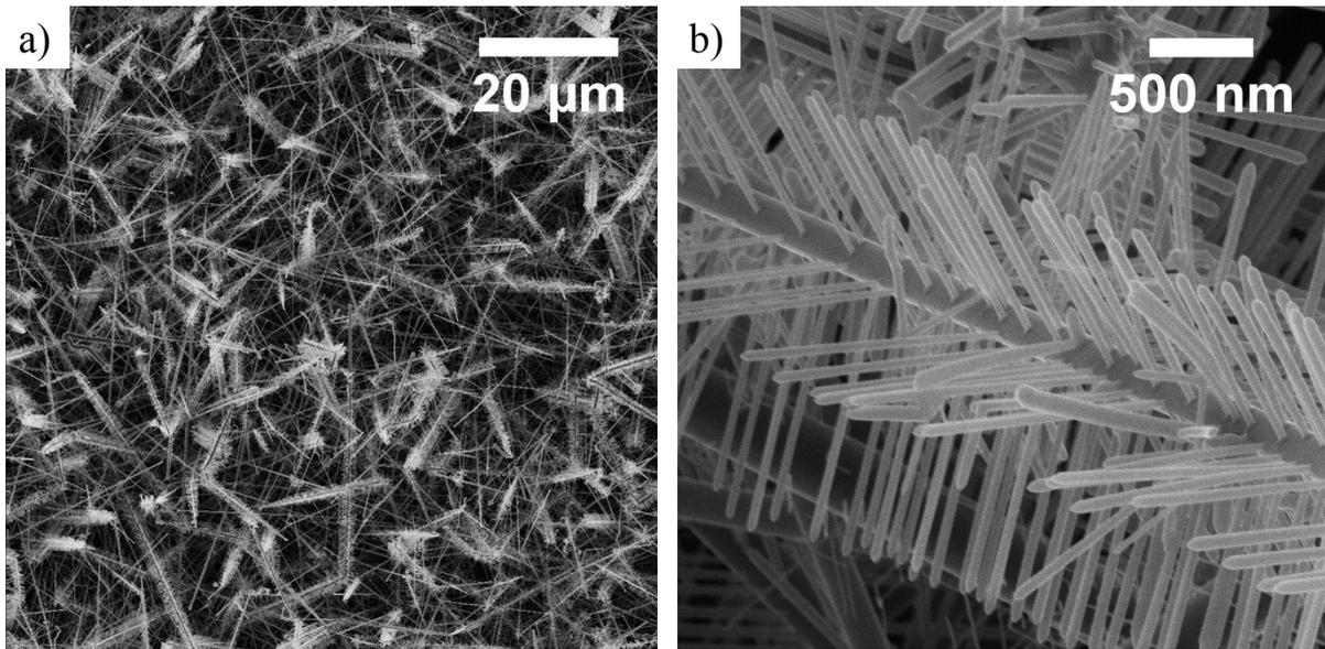
**Figure S4:** SEM images of the branched  $\text{Ge}_{1-x}\text{Sn}_x$  nanowires grown using a specific TET concentration. The density of these branched nanowires across the substrate can be seen in (a), these branched nanowires are relatively high yield compared to the non-branched nanowires. (b) Displays the highly ordered nature of these branches, with the branch nanowires seemingly aligned along the trunk.
