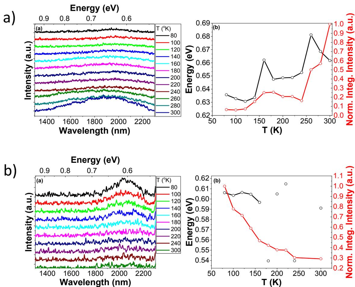
**Figure S13:** Temperature dependent photoluminescence studies in part (a) and (b) convey the different behaviours of the Ge<sub>1-x</sub>Sn<sub>x</sub> nanowires with 7.4 and 9.1 at. % Sn respectively. They also display the shift in energy and integrated intensity as a function of temperature.
