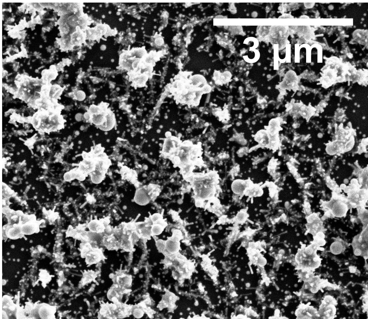
**Figure S6:** SEM (a) of Ge<sub>1-x</sub>Sn<sub>x</sub> nanowires grown with TET as the Sn source at 470 °C. EDX analysis revealed an erratic amount of Sn incorporation from one nanowire to another (*i.e.* 4 – 8 at. % Sn).
