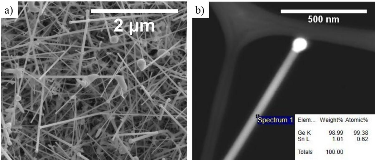
**Figure S2:**  $\text{Ge}_{1-x}\text{Sn}_x$  nanowires grown using tetraallytin (TAT) as a Sn source. (a) depicts Sn segregation and clustering using TAT as the Sn precursor. The  $\text{Ge}_{1-x}\text{Sn}_x$  nanowires grown from TAT also have a very low amount of Sn incorporation (b), with the mean Sn content of approximately 2 at. %.
