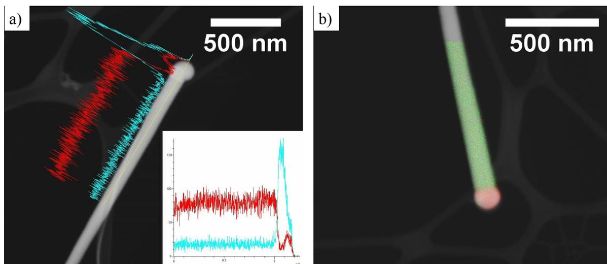
**Figure S8:** EDX analysis of Ge<sub>1-x</sub>Sn<sub>x</sub> nanowires catalysed by Au<sub>0.80</sub>Ag<sub>0.20</sub> nanoparticles with 9.14 at. % Sn. In the linescan (a) Ge is denoted by red and Sn by blue. In the elemental map (b) Ge is denoted by Green and Sn by red. The Sn rich nature of the seed and lack of Sn clustering and segregation is apparent from the linescan in (a) and the elemental map in (b).
