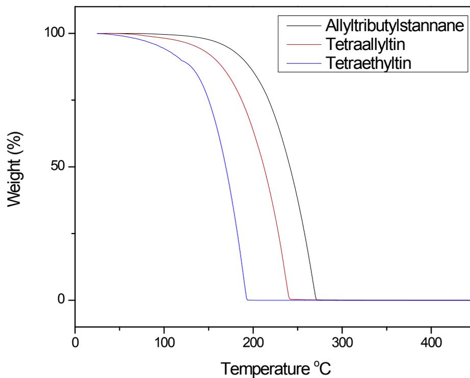
**Figure S3:** Thermogravimetric Analysis (TGA) of the three Sn precursors; allyltributylstanne, tetraallytin and tetraethyltin. The decomposition temperatures of these Sn molecules follows the general trend of their boiling points; ranging from TET with the lowest boiling point (181 °C at atmospheric pressure) to ATBS with the highest (353 °C at atmospheric pressure).
