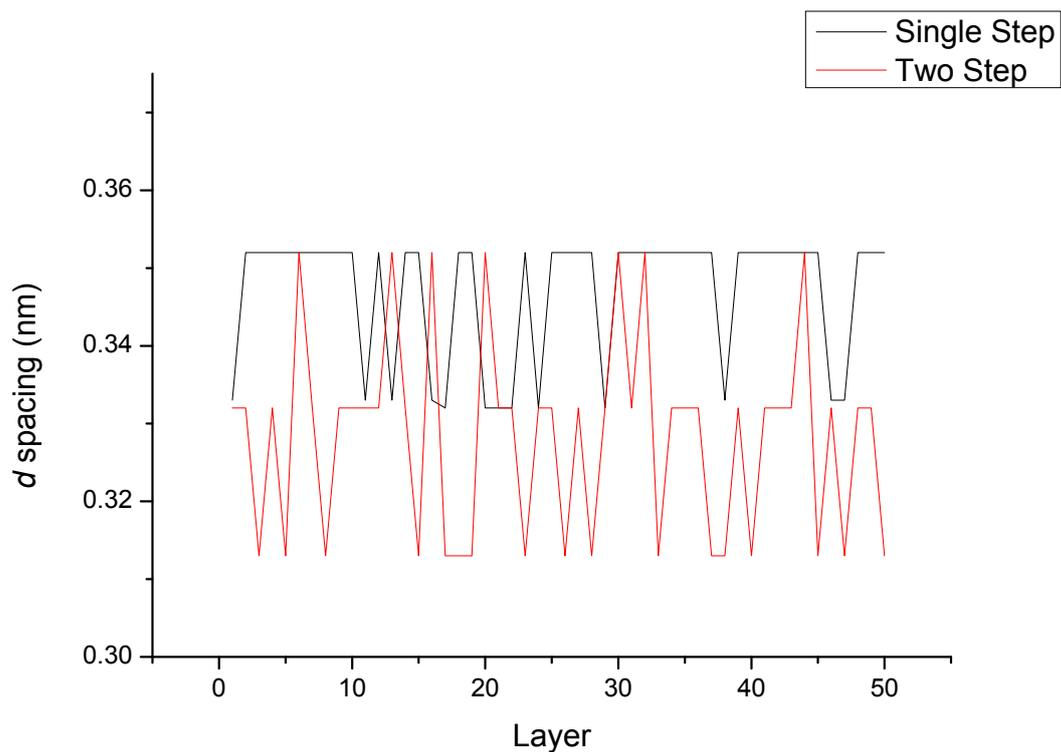
**Figure S10:** Comparison of the interplanar ( $d$ ) spacing of 50 successive layers of  $\text{Ge}_{1-x}\text{Sn}_x$  nanowires. The black line denotes the nanowires fabricated through increased growth kinetics with 9.1 at. % Sn, while the red line represents nanowires grown using a two-step method with 9.2 at. % Sn.
