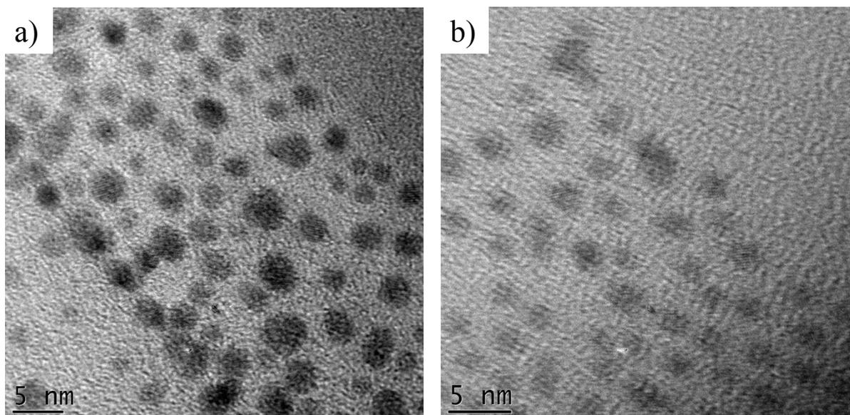
**Figure S1:**  $\text{Au}_{1-x}\text{Ag}_x$  nanoparticles used to catalyse the growth of the  $\text{Ge}_{1-x}\text{Sn}_x$  nanowires. The nanoparticles have increasing Ag content from (a)  $\text{Au}_{0.90}\text{Ag}_{0.10}$  to (b)  $\text{Au}_{0.80}\text{Ag}_{0.20}$  and both have a mean diameter of  $\sim 4\text{-}5$  nm.
