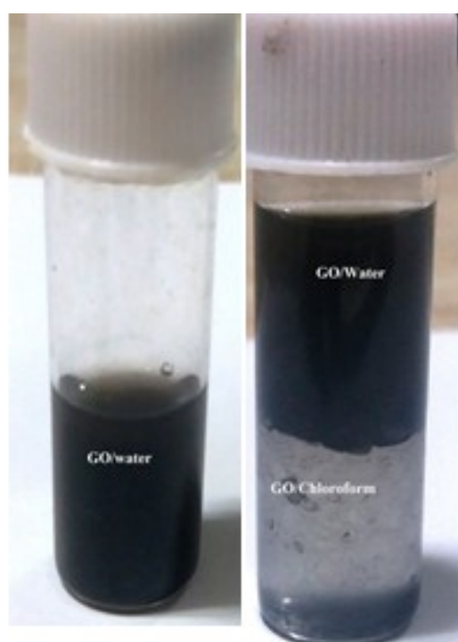
Fig. S1: Picture of GO in water (left) and GO + water/GO+ Chloroform after sonication (right) showing dispersion in two phases.
