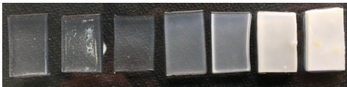
Figure S1. The photography of the hydrogels after dipped in different concentration of Py aqueous solution for 3 min.
