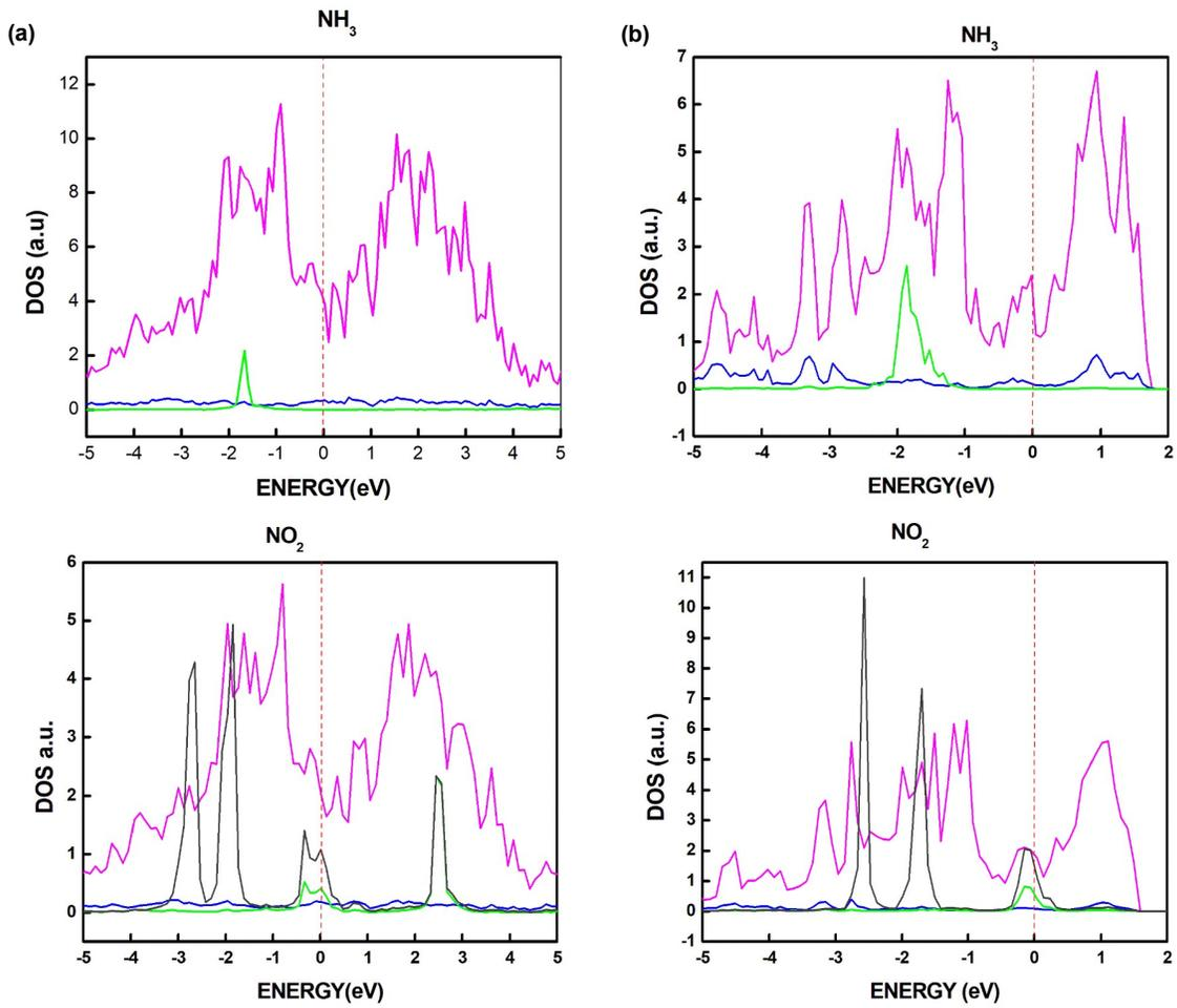
**Figure S5.** Partial Density of States (PDOS) of the MoTe<sub>2</sub> with adsorbed gas molecules in (a) Pt surface and (b) Ti. Note that the Fermi level is fitted at 0 eV. Colour code used for the PDOS is Mo-d (magenta), Te-s (blue), N-p (green) and O-p (Dark grey) respectively.
