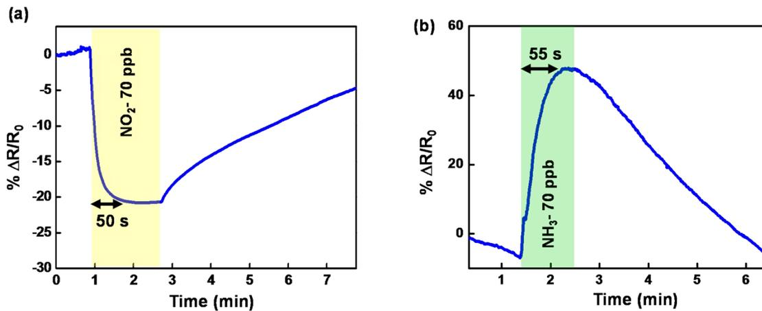
**Figure S4.** Magnified first cycles in (a) Figure 6a and (b) Figure 6b, showing the relative resistance change of the MoTe<sub>2</sub> FET under exposure to 70-ppb NO<sub>2</sub> and 70-ppb NH<sub>3</sub>, respectively.
