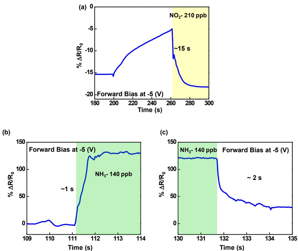
**Figure S1.** (a) Magnified third cycle in Figure 4b, showing the SD responses under exposure to 210-ppb  $\text{NO}_2$ . The response time of  $\text{NO}_2$  was  $\sim 15$  s. A forward-bias voltage of -5 V was applied across the device. (b, c) Magnified second cycle in Figure 4d, showing the response and recovery behaviour of the SD under exposure to 140-ppb  $\text{NH}_3$ . At a forward bias of -5 V, the response time was  $\sim 1$  s and the recovery time was  $\sim 2$  s.
