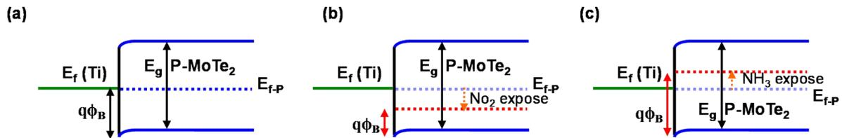
**Figure S2.** Energy-band diagram of the  $\alpha$ -MoTe<sub>2</sub> SD in three different conditions: (a) before gas exposure; (b) under NO<sub>2</sub> gas exposure, showing the reduction of the Fermi level; and (c) under NH<sub>3</sub> gas exposure, indicating the increase of the Schottky-barrier height compared with the pre-exposure condition.
