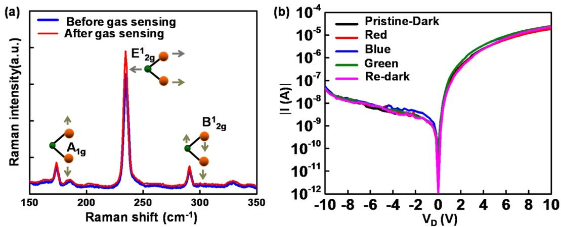
**Figure S3.** (a) Raman spectra of MoTe<sub>2</sub> before (blue) and after (red) gas sensing in NO<sub>2</sub> and NH<sub>3</sub>. The Raman spectra confirms the stability of the MoTe<sub>2</sub> sensors after sensing. (b) The I–V curves of the SD under irradiation from red, green and blue light-emitting diodes (LEDs). The SD is insensitive to the visible light.
