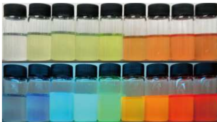
Figure S16. Photographs showing the emission color of the CsPbBr 3 NWs (d=6.5 nm) with different compositions after halide-exchange under day light and UV illumination.
