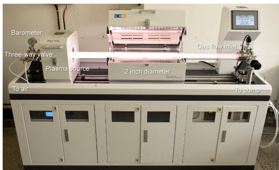
Fig. S2 The photograph of the PACVD system used for growing graphene directly on Si substrate.
