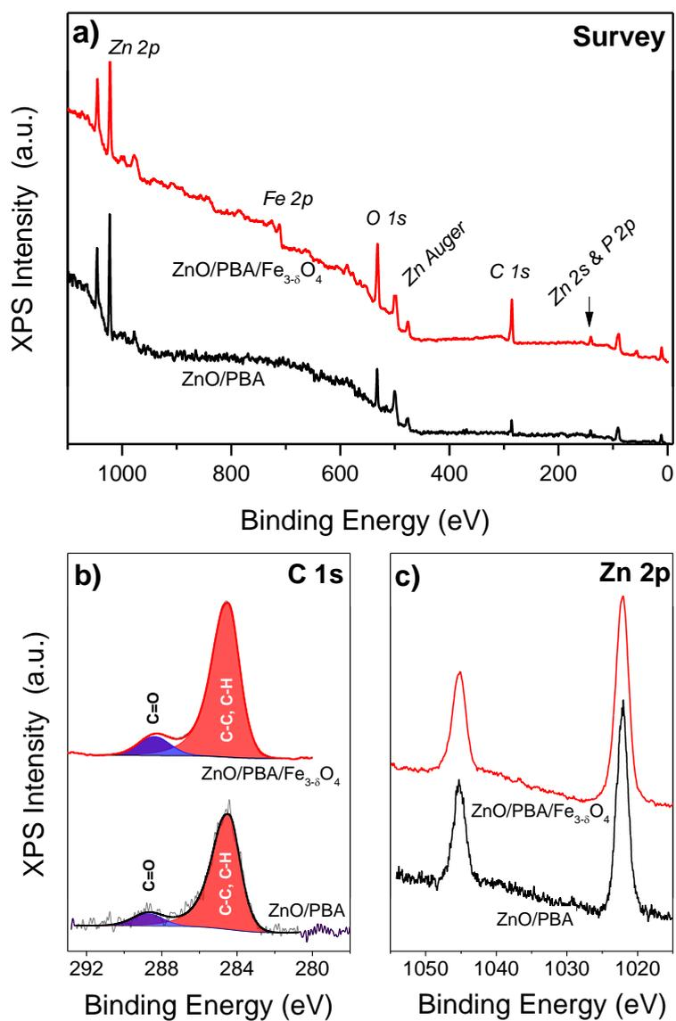
**Figure 6S.** XPS spectra of ZnO nanorod arrays measured after PBA functionalization (ZnO/PBA) and consequent decoration with  $\text{Fe}_{3-\delta}\text{O}_4$  nanoparticles (ZnO/PBA/ $\text{Fe}_{3-\delta}\text{O}_4$ ). a) survey spectra, b) C 1s and c) Zn 2p regions.
