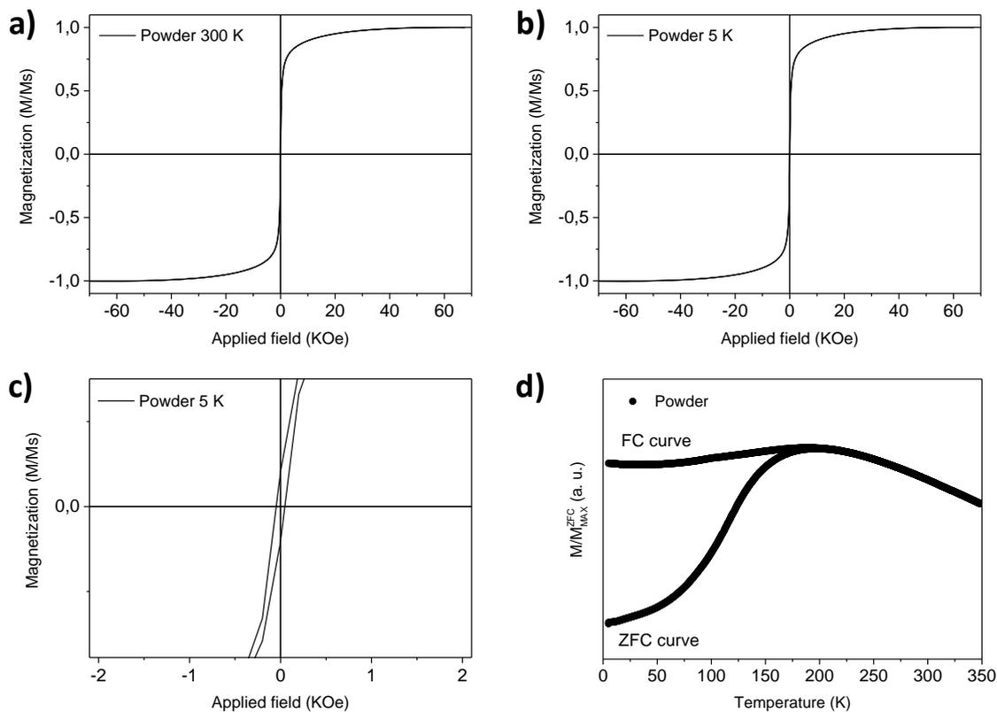
**Figure 11S.** Magnetic measurements of  $\text{Fe}_{3-\delta}\text{O}_4$  nanoparticles in the powder state. a) Magnetization recorded against a magnetic field at a) 300 K and b, c) at 5 K. c) shows the low field region in b). d) Magnetization curve recorded against temperature after cooling down with no magnetic field (ZFC curve) and after cooling down under a 75 Oe magnetic field (FC curve).
