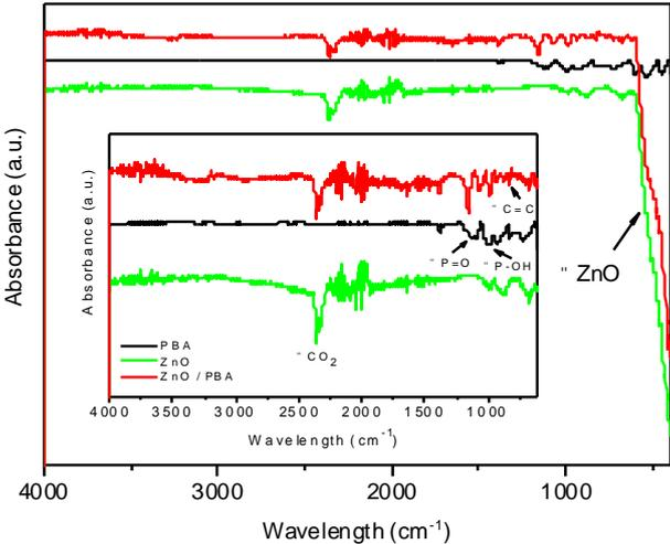
**Figure 4S.** FTIR spectra of zinc oxide nanorod array functionalized by PBA (ZnO/PBA), 1,4-phenylenebis(phosphonic acid) in the solid state (PBA) and zinc oxide nanorod array (ZnO).
