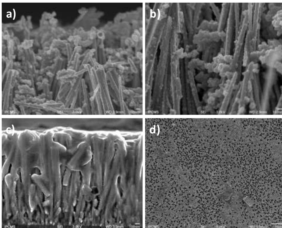
**Figure 8S.** SEM micrographs of ZnO nanorod arrays after dipping in a PBA solution. a, b) 0.5 mg/mL for 7 h. c, d) 2 mg/mL for 10 min. All samples were subsequently dipped in a followed by dipping in  $\text{Fe}_3\text{O}_4$  nanoparticle solution for 2 h. a, b, c) are top views. d) is cross section view.
