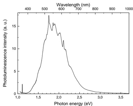
**Figure 12S.** Photoluminescence spectra of  $\text{Fe}_{3-\delta}\text{O}_4$  nanoparticles drop casted on a glass substrate. Spectral fringes are visible here because no filtering of the spectrum could be performed without also removing sharp structures (at 525, 550 and 610 nm) that seems to be characteristic of  $\text{Fe}_{3-\delta}\text{O}_4$ .
