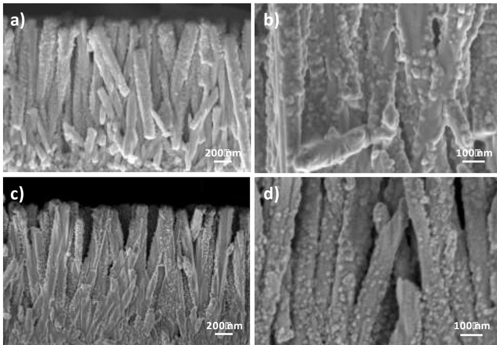
**Figure 7S.** SEM micrographs of PBA functionalized (0.5 mg/mL, 10 min) ZnO nanorod array after dipping in a suspension of  $\text{Fe}_3\text{O}_4$  nanoparticles for a, b) 10 min and c, d) 7 h.
