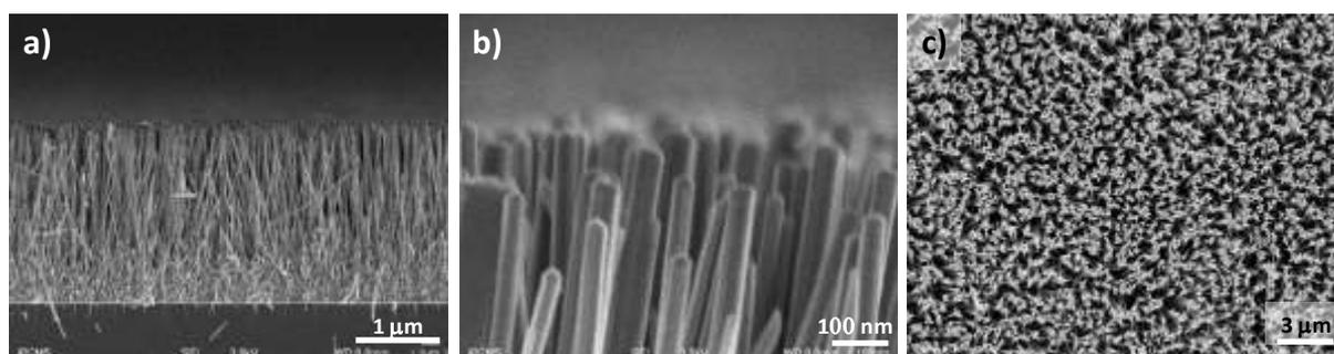
**Figure 1S.** Micrograph of ZnO nanorods before functionalization by PBA and grafting of iron oxide nanoparticles. a, b) Cross section and c) top views corresponding SEM micrographs.
