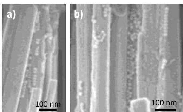
**Figure 10S.** SEM micrograph showing that some nanoparticles spontaneously aligned as single nanoparticle chains thanks to dipolar interactions.
