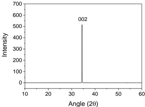
**Figure 3S.** XRD pattern of ZnO nanorod arrays decorated with Fe<sub>3-δ</sub>O<sub>4</sub> nanoparticles.
