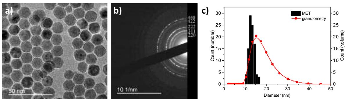
**Figure 2S.** a) TEM micrograph of  $\text{Fe}_{3-\delta}\text{O}_4$  nanoparticles. b) Electron diffraction pattern showing the crystallinity of nanoparticles which can be assigned to the spinelle structure of iron oxide (magnetite  $\text{Fe}_{3-\delta}\text{O}_4$  JCPDS file 19-629 or maghemite  $\gamma\text{-Fe}_2\text{O}_3$  JCPDS file 39-1346 phases). c) Size distribution measured from TEM micrographs and hydrodynamic diameter distribution measured by granulometry
