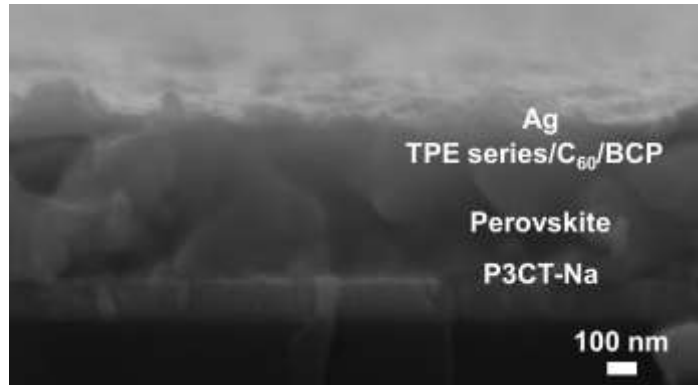
Fig. S4 The cross-sectional scanning electron microscopy (SEM) image of the device.
