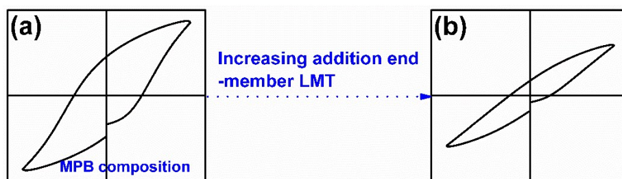
Figure S1 The evolution of P-E loops (a) MPB composition with tetragonal-pseudocubic phase and (b) ergodic phase composition with pseudo-cubic phase for BKT-LMT systems. Both the ceramics exhibits poor energy storage properties by CS.
