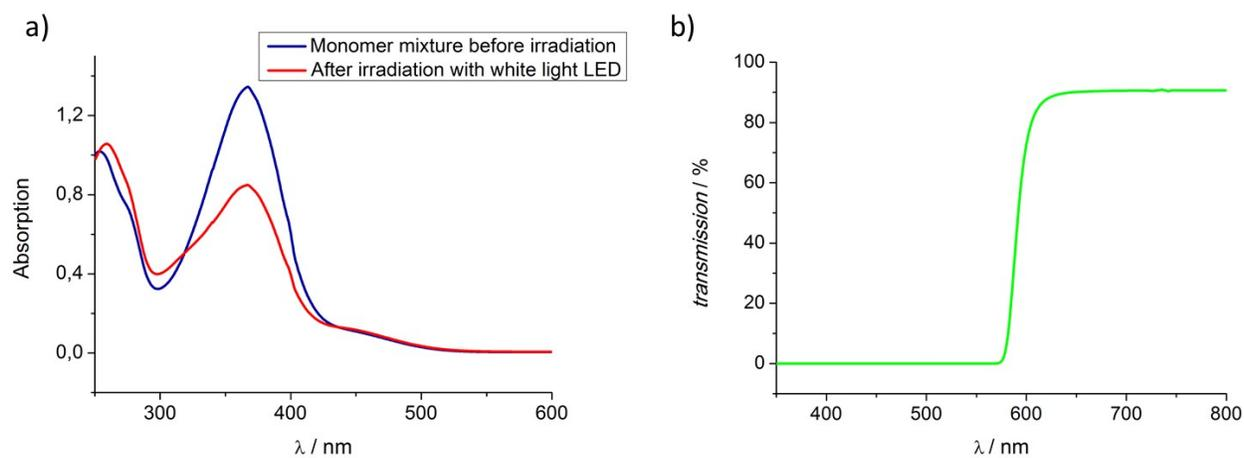
Figure S3. a) UV-vis spectrum of the monomer mixture before and after irradiation with the white light LED which was used to induce photoactuation. b) Transmission spectrum of the red light filter which was used to induce photoresponsive back-deformation.
