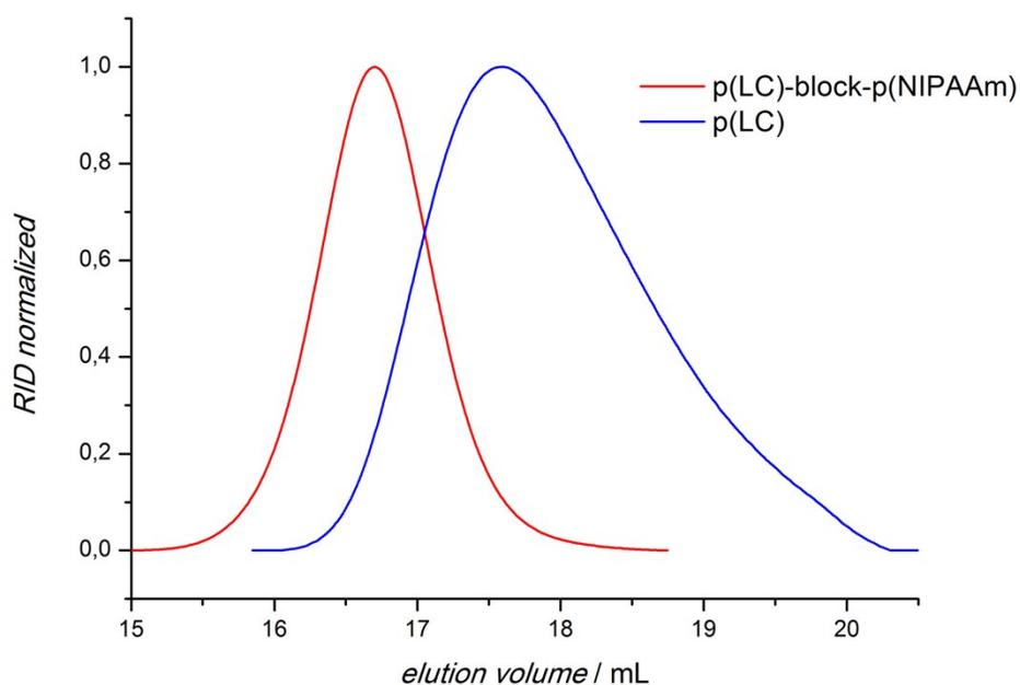
Figure S1. GPC elution curves of *p(LC)* and *p(LC)-block-p(NIPAAm)*.
