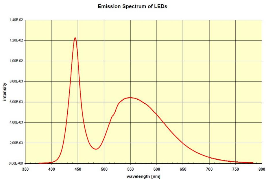
Figure S2. Emission spectrum of the coldlight source that was used to induce photoresponsive actuation. (Kindly provided by Schott AG)
