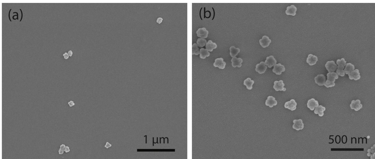
Figure S1: SEM images of 117 nm Au-silica heterostructure centrifuged after a) 1 hour of reaction, b) 1.5 hour of reaction
