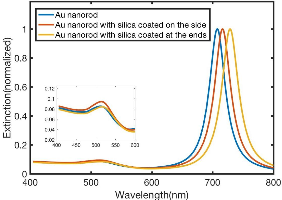
Figure S3: Simulated extinction spectra of Au nanorod (blue), Au nanorod with silica coated on the side (red) and Au nanorod with silica coated at the ends (yellow). The inset figure shows the corresponding simulated extinction spectra of the transverse plasmonic mode only.
