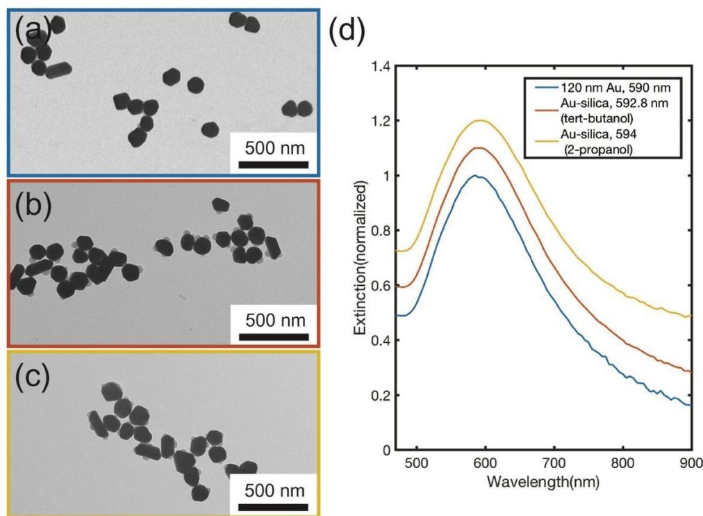
Figure S2: TEM images of a) 120 nm citrate capped Au nanoparticle, 120 nm Au-silica heterostructure synthesized in b) tert-butanol, c) 2-propanol, d) UV-vis spectra of the corresponding structures.
