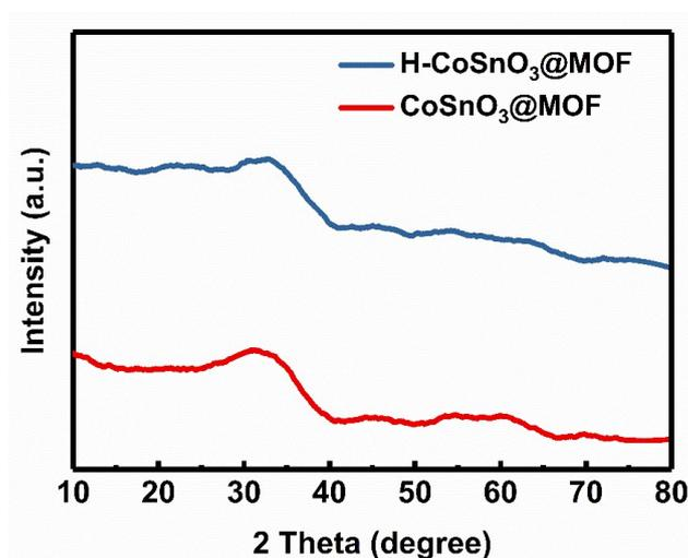
**Figure S2.** XRD pattern of the hollow CoSnO<sub>3</sub>@MOF and H-CoSnO<sub>3</sub>@MOF nanocubes.
