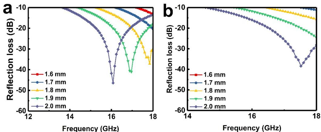
**Figure S6.** Calculated RL curves of  $\text{SnO}_2/\text{Co}_3\text{Sn}_2@\text{C}$  and  $\text{SnO}_2/\text{Co}_3\text{Sn}_2@\text{Air}@\text{C}$  with the thickness of 1.6 -2.0 mm.
