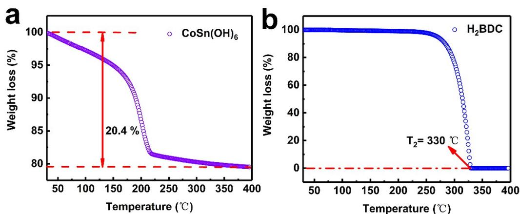
**Figure S1.** TGA curves of CoSn(OH)<sub>6</sub> (a) and H<sub>2</sub>BDC (b) which were tested in air from 50°C to 400°C.
