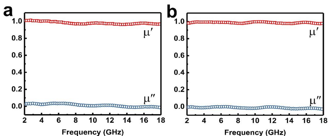
**Figure S4.** Real part ( $\mu'$ ) and imaginary part ( $\mu''$ ) of permeability for  $\text{SnO}_2/\text{Co}_3\text{Sn}_2@\text{C}$ (a) and  $\text{SnO}_2/\text{Co}_3\text{Sn}_2@\text{Air}@\text{C}$ (b)
