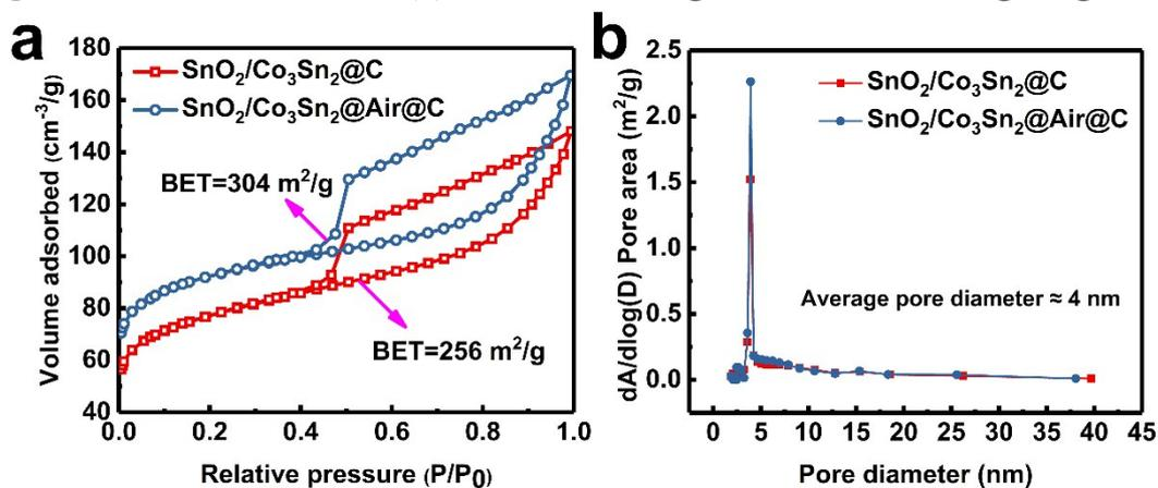
**Figure S8.**  $\text{N}_2$  adsorption-desorption isotherms (a) and pore size distributions (b) of  $\text{SnO}_2/\text{Co}_3\text{Sn}_2@\text{C}$  and  $\text{SnO}_2/\text{Co}_3\text{Sn}_2@\text{Air}@\text{C}$  hybrids.
