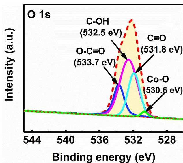
**Figure S5.** XPS survey spectrum of O 1s region of  $\text{SnO}_2/\text{Co}_3\text{Sn}_2@\text{C}$ .
