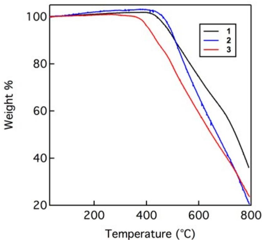
Figure S4. Thermal gravimetric analysis of compounds **1** (black), **2** (blue), and **3** (red).
