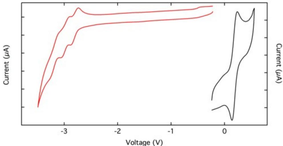
Figure S5. Cyclic voltammograms (first oxidation and reduction) for **1**.
