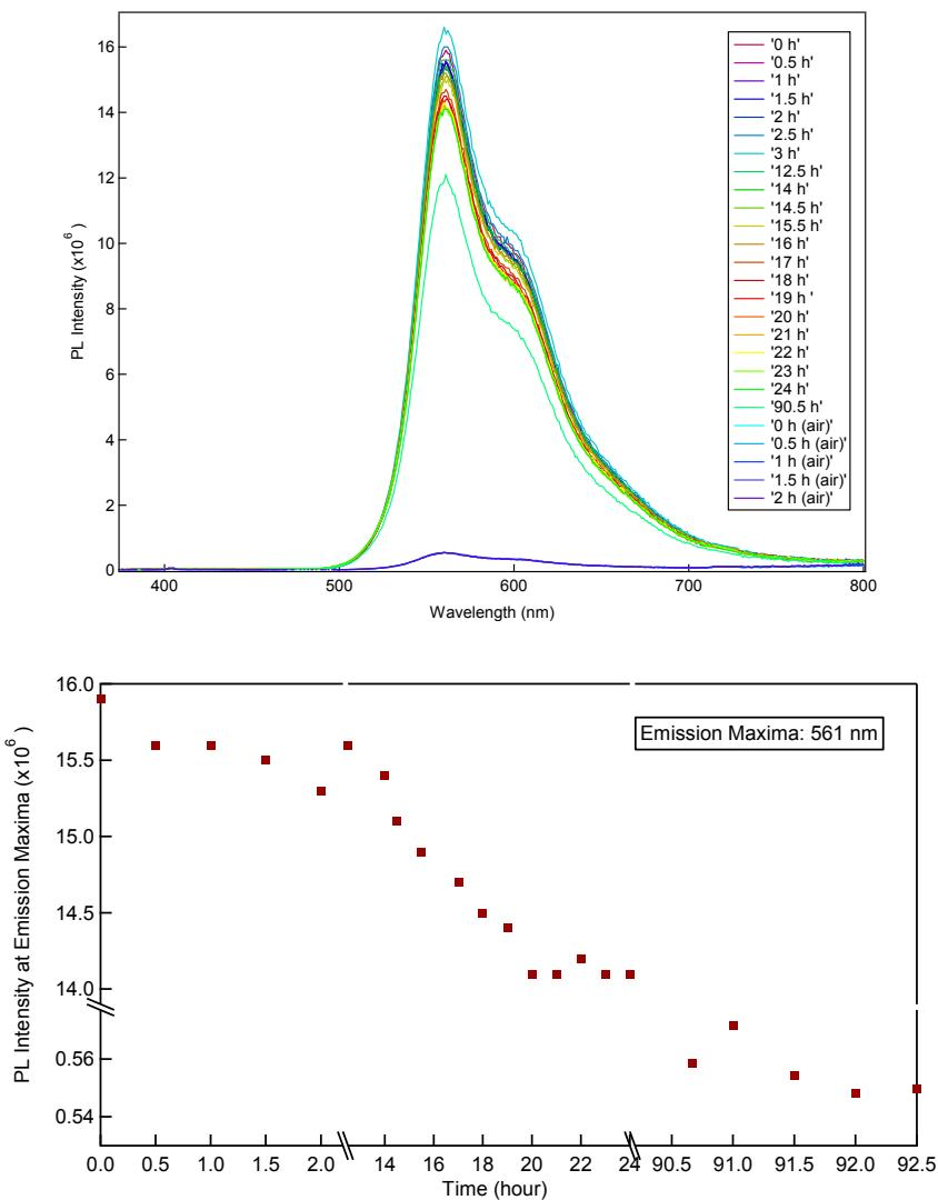
Figure S7. Change in PL intensity of dendrimer **3** over time in deoxygenated and oxygenated toluene. The sample was stored in the light between measurements. a) PL spectra. b) Change in peak maximum over time with each point corresponding to a spectrum in a).
