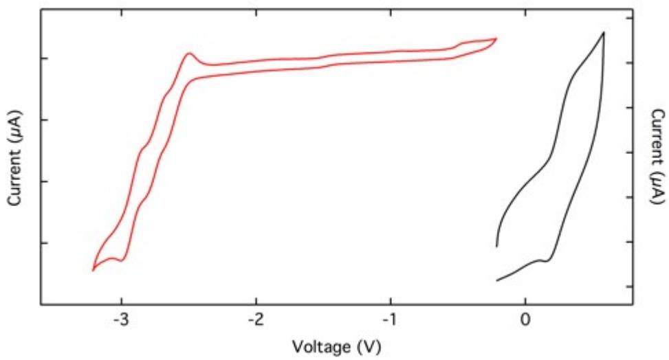
Figure S6. Cyclic voltammograms (first oxidation and reduction) for **2**.
