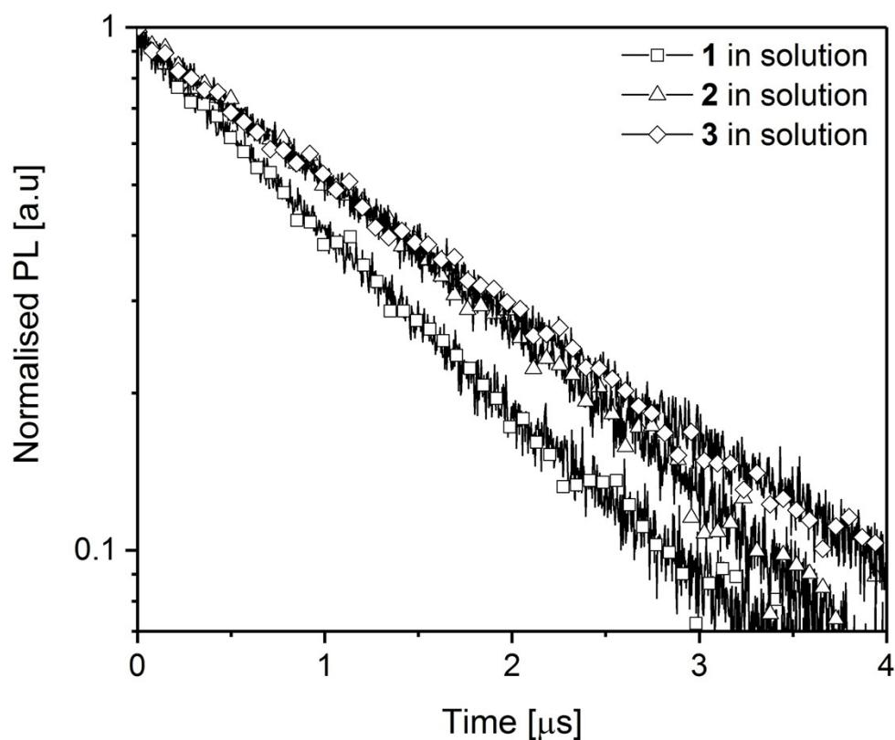
Figure S8. Time resolved photoluminescence data of dendrimers **1**, **2** and **3** in solution.
