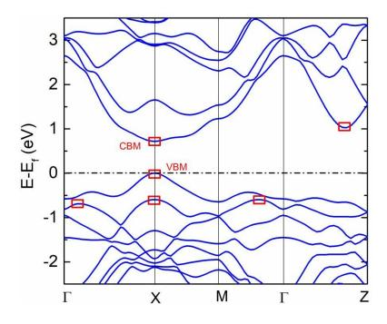
Fig. S2. Calculated band structure of TlGaTe<sub>2</sub>.
