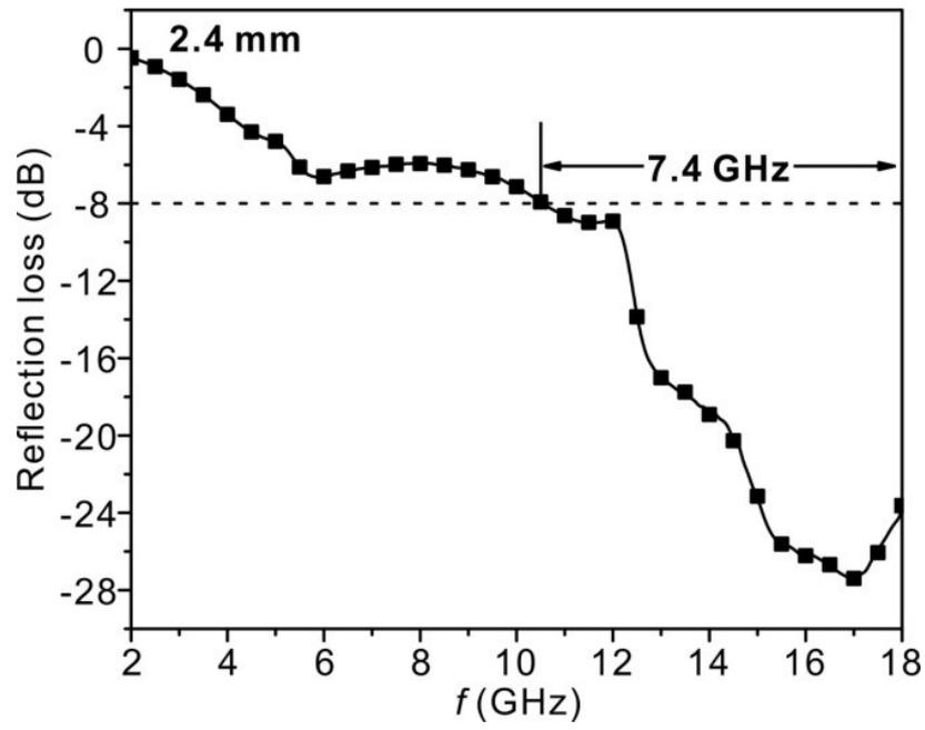
**Fig. S5** *RL* of composites based on the typical GM@AgCPs at  $V = 46\%$ . According to the  $\lambda/4$  thickness equation, thickness of composites is selected as 2.4 mm.
