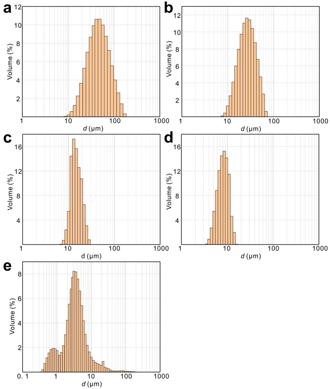
**Fig. S1** The average diameter of various GM: (a)41.0, (b) 27.6, (c) 13.3, (d) 8.1 and
