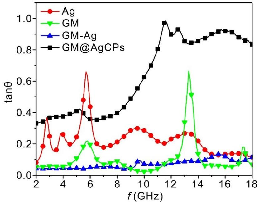
**Fig. S4** The tangent values of dielectric loss of composites based on various fillers of Ag powders at  $V = 19\%$ , GM at  $V = 45\%$ , GM-Ag at  $V = 45\%$  and the typical GM@AgCPs at  $V = 45\%$ .
