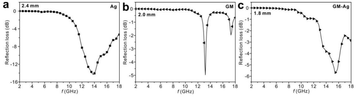
**Fig. S3** *RL* of composites based on various fillers of (a) flaky Ag powders at  $V = 19\%$ , (b) GM at  $V = 45\%$  and (c) GM-Ag at  $V = 45\%$ , other conditions as Fig. 4. According to  $\lambda/4$  matching model, thickness in (a), (b) and (c) for *RL* is 2.4, 2.0 and 1.8 mm, respectively.
