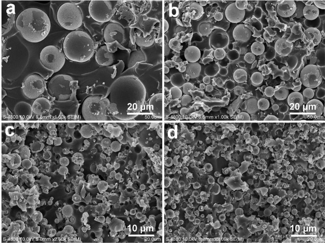
**Fig. S6** SEM images of cross-section samples of composites based on GM@AgCPs with various  $d$  of (a) 27.7  $\mu\text{m}$  at  $V = 45\%$ , (b) 13.4  $\mu\text{m}$  at  $V = 43\%$ , (c) 8.2  $\mu\text{m}$  at  $V = 30\%$  and (d) 3.0  $\mu\text{m}$  at  $V = 27\%$ ,  $d_{\text{Ag}}$  of GM@AgCPs as Fig. 2b, Fig. 6b, 6c, and 6d, respectively.
