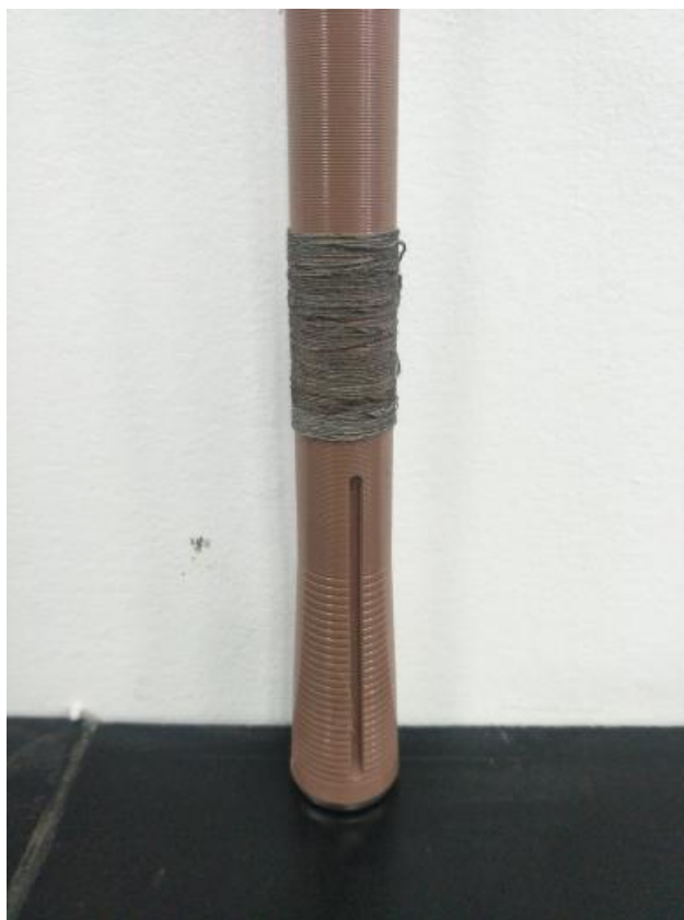
Figure S1 Digital image of the Ni-coated cotton yarns wound on a bobbin.
