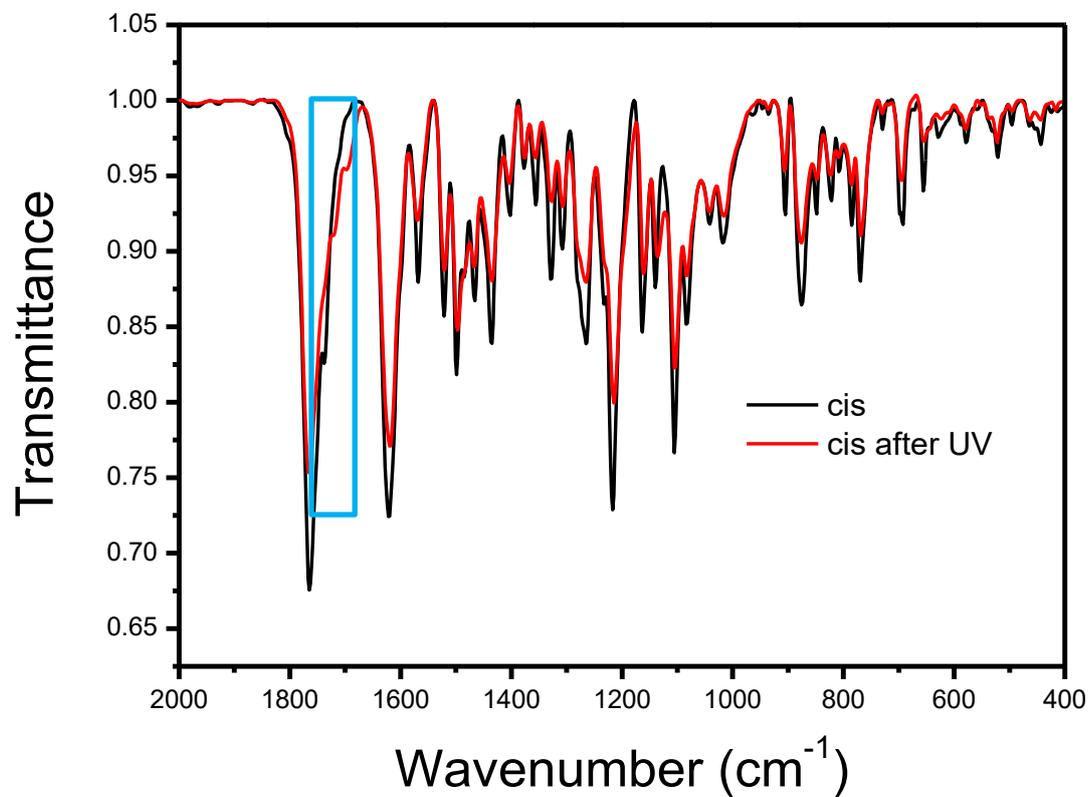
Figure S18. IR spectra of cis-RhRh single crystal before and after UV.
