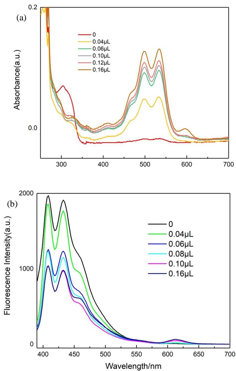
Figure S8. (a) Absorption spectra and (b) fluorescence spectra of trans-RhRh in DCM solution ( $6.7 \mu\text{M}$ ) with the addition of different volume of TFA.
