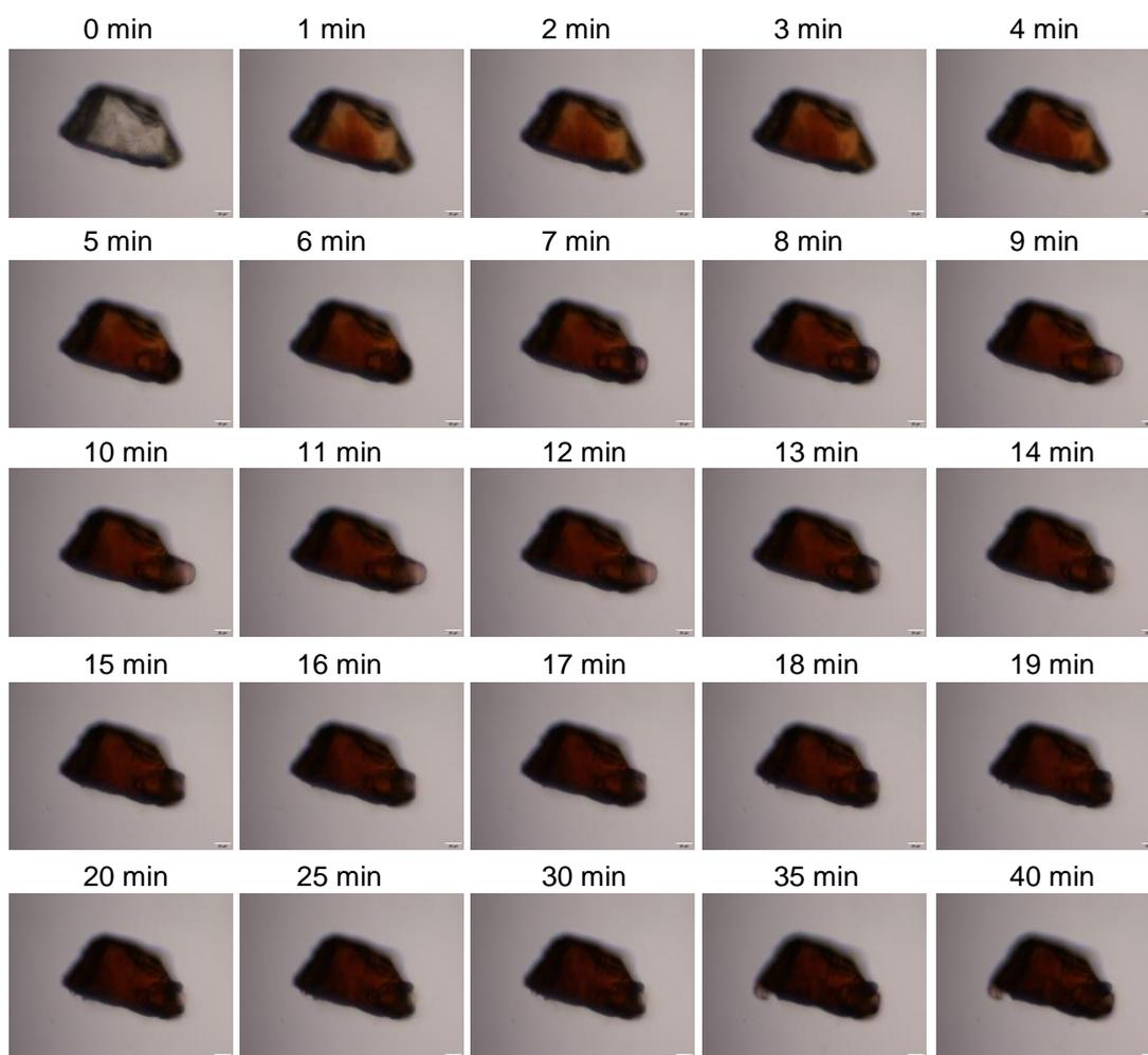
Figure S16. The trans-RhRh single crystal turned from colorless to dark red increasing the irradiation time.
