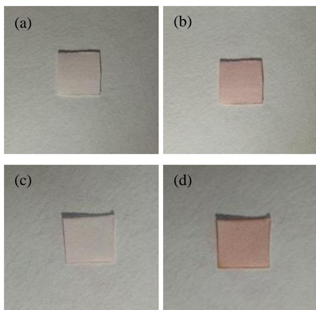
Figure S20. Prepared filter paper by dropping cis/trans-RhRh DCM solution before (a) (c) and after (b) (d) UV. cis-RhRh: (a)(b), trans-RhRh: (c)(d)
