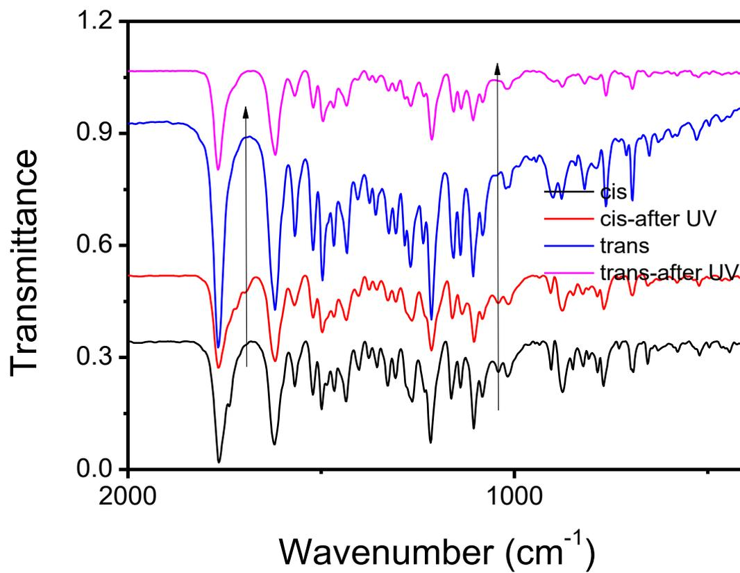
Figure S19. IR spectra of cis- and trans-RhRh single crystal before and after UV.
