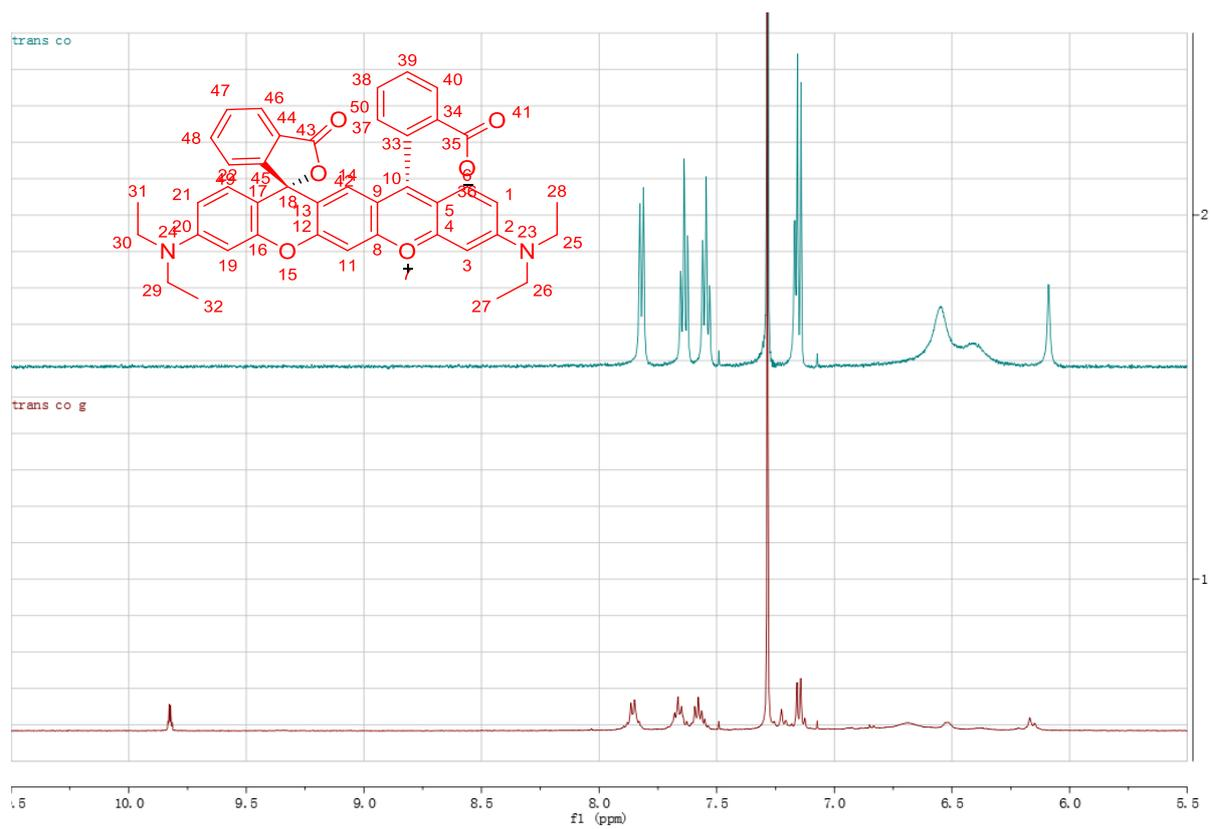
Figure S12. <sup>1</sup>H NMR of trans-RhRh solution in CDCl<sub>3</sub> before (up) and after (bottom) UV irradiation. (The integral of 9.83 peak is 0.25.)
