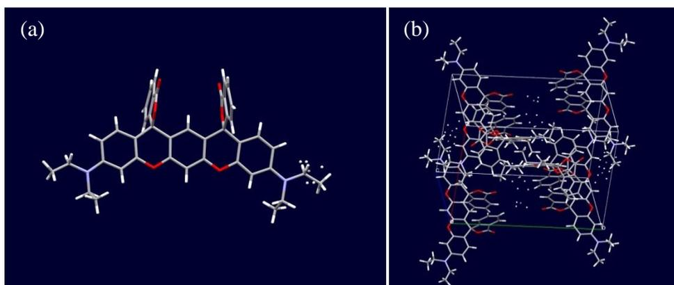
Figure S14. (a) The molecular geometry and (b) the unit cell in the trans-RhRh single crystal.
