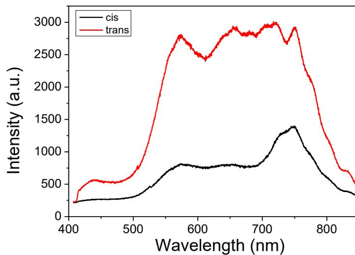
Figure S17. Fluorescence spectra of cis- and trans-RhRh single crystal after UV.
