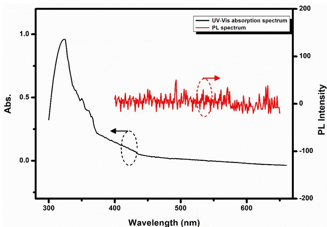
**Figure S2** PL and UV-Visible absorption spectra of the product synthesized at  $C_{PB}:C_{CB} = 0.25$ . No obvious PL signal was obtained, indicating that Cs<sub>4</sub>PbBr<sub>6</sub> can not emit light in the visible wavelength range.
