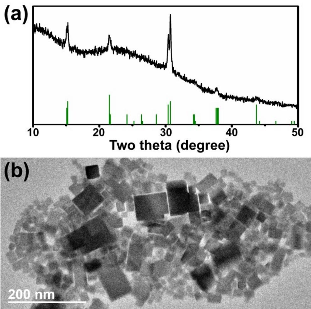
**Figure S5** Pure CsPbBr<sub>3</sub> nanocrystals fabricated by injecting 70  $\mu$ l of DMF composed of an equal amount of PbBr and CsBr at a concentration of 0.04 M into 10 ml of toluene. (a) XRD pattern. Olive lines marked the position of the standard XRD peaks of CsPbBr<sub>3</sub> (PDF No. 180364). (b) TEM image.
