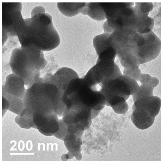
**Figure S1** TEM image of Cs<sub>4</sub>PbBr<sub>6</sub> nanocrystals synthesized at  $C_{PB}:C_{CB} = 0.25$  ( $C_{CB} = 0.04$  M). The size of the Cs<sub>4</sub>PbBr<sub>6</sub> nanocrystals ranges from 80 nm to 350 nm with a poor dispersibility.
