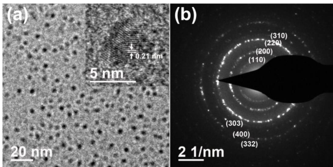
**Figure S4** (a) TEM and (b) SAED characterization of the ultrafine spherical  $CsPb_2Br_5$  nanocrystals. Insert in (a): High-resolution TEM image.
