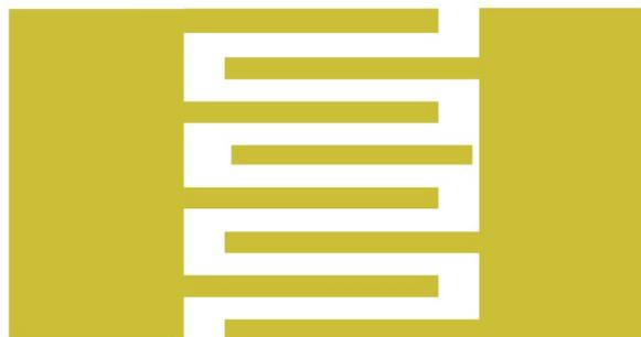
**Fig. S2** Schematic diagram of Au interdigital electrode.
