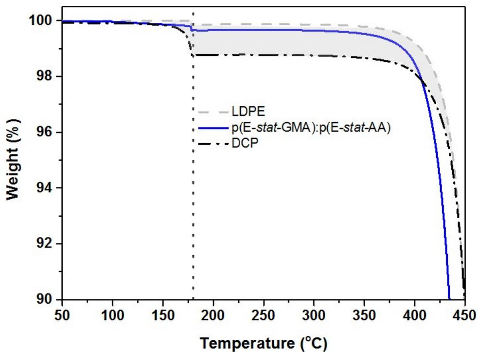
Fig. S3 TGA thermograms of neat LDPE, LDPE crosslinked with 2 % wt dicumyl peroxide (DCP) and p(E-stat-GMA):p(E-stat-AA) blend cured at 180 °C for 15 min. The shaded area highlights the weight loss of volatile byproducts that arise from DCP decomposition.
