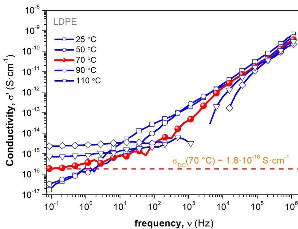
Fig. S7 Conductivity measured at different temperatures, ranging from 30 to 130 °C in 20 °C steps, for reference LDPE.
