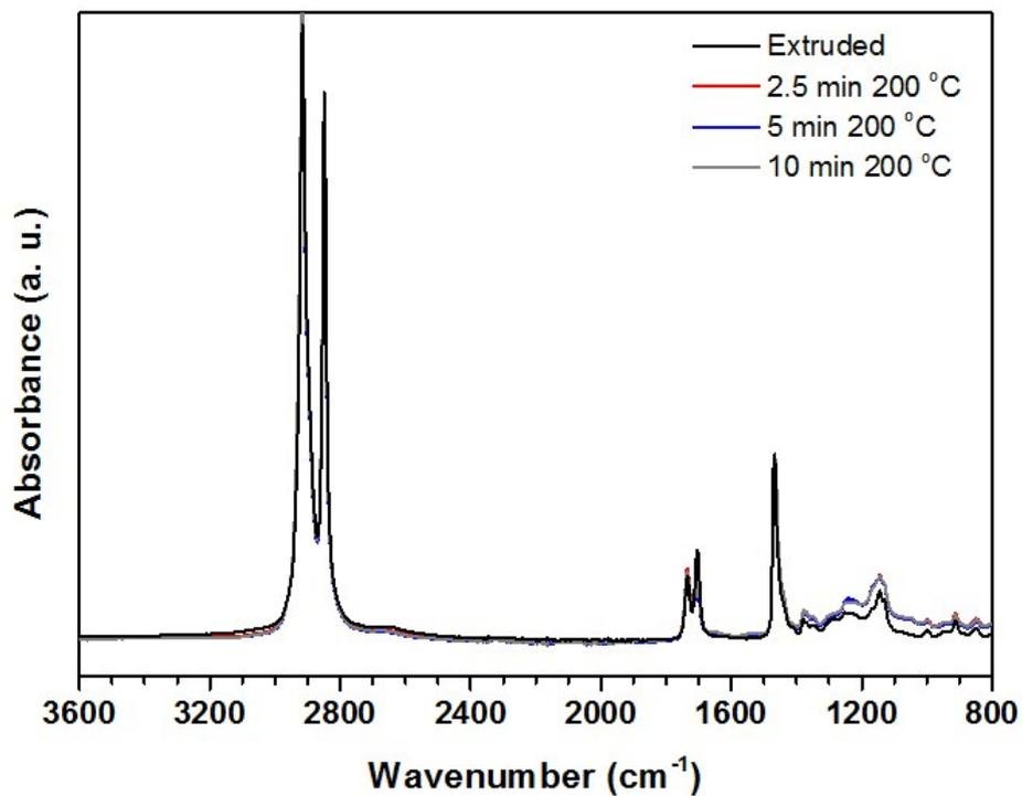
Fig. S2 ATR-FTIR spectrum of p(*E-stat*-GMA):p(*E-stat*-AA) polymer blend at stoichiometric ratios crosslinked at 200 °C for 2.5, 5 and 10 min. Analysis of the spectra indicates that the main side reactions of the hydroxyl group can be ruled out, as evidenced by the absence of water absorption band in the region between 3500-3700 cm<sup>-1</sup>, associated with symmetric and asymmetric stretching of O-H groups.
