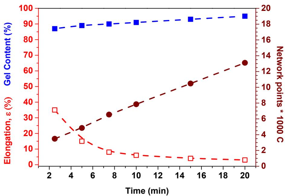
Fig. S6 Effect of time on Hot set Elongation ( $\square$ ), Network point formation\*1000 C atoms ( $\bullet$  from hot set) and Gel content ( $\blacksquare$ ) for a 1.7:1 stoichiometric p(E-stat-GMA):p(E-stat-AA) formulation cross- linked at 200°C.
