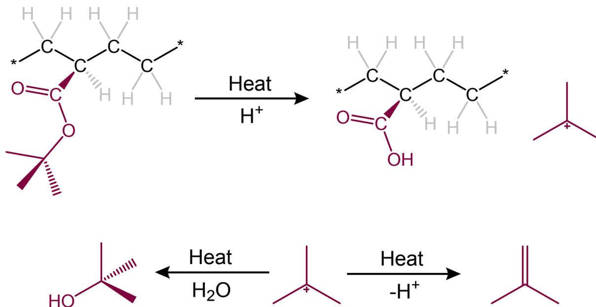
Fig. S10 Deprotection of p(*E-stat*-TBA) at temperature  $T > 200$  °C: tert-butyl acrylate in presence of H<sup>+</sup> released from acrylic acid units releases a tert-butyl cation, which predominantly will react with moisture to give tert-butyl alcohol.
