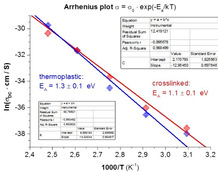
Fig. S8 Arrhenius plot for reference LDPE (top), as well as the thermoplastic and crosslinked copolymer blend (bottom).
