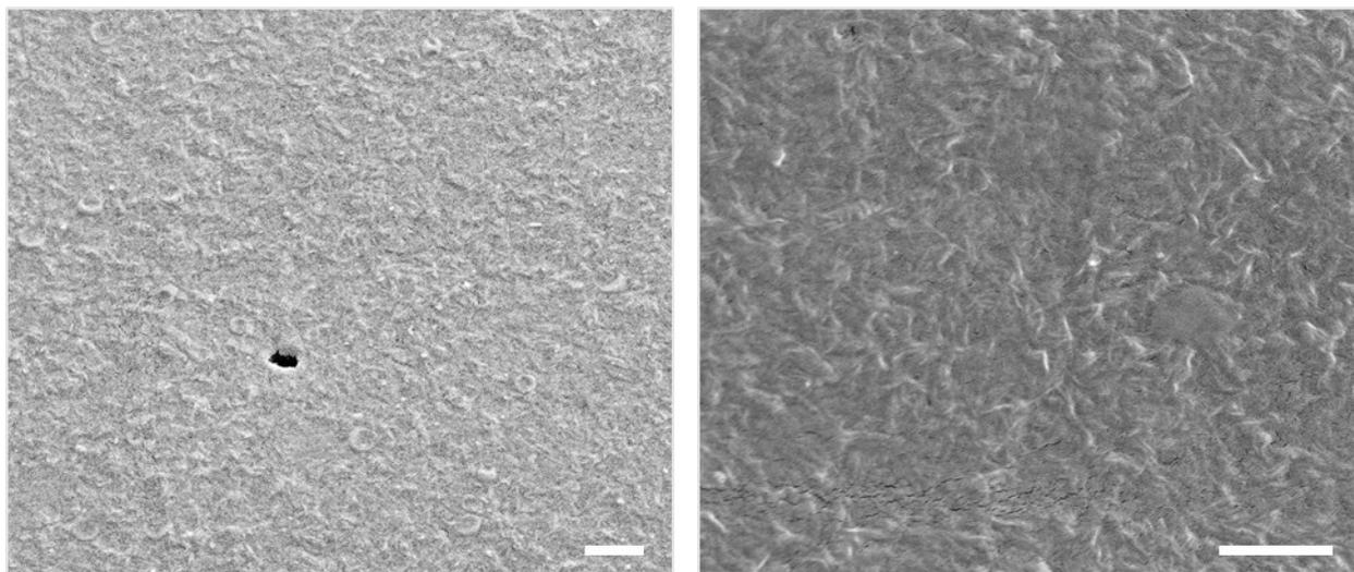
Fig. S5 SEM micrographs of a 1.7:1 stoichiometric p(*E-stat*-GMA):p(*E-stat*-AA)blend. No phase separation of the blend components can be detected. Scale bar equal to 1  $\mu\text{m}$ .
