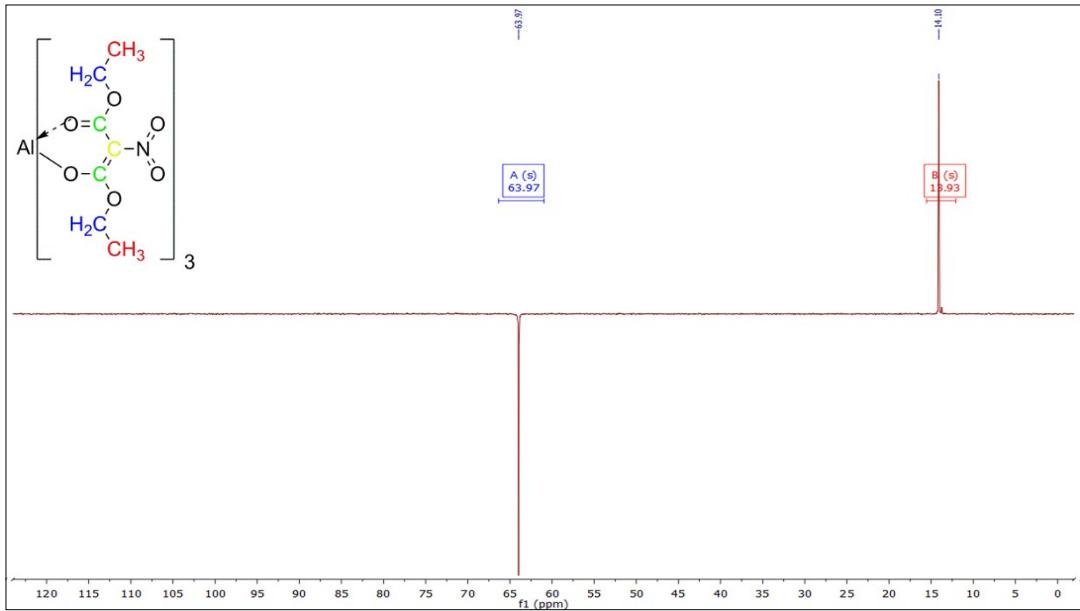
**Fig. S7:** DEPT-spectrum ( $\text{CDCl}_3$ ) of tris[(diethyl-2-nitromalonato)aluminum(III)].
