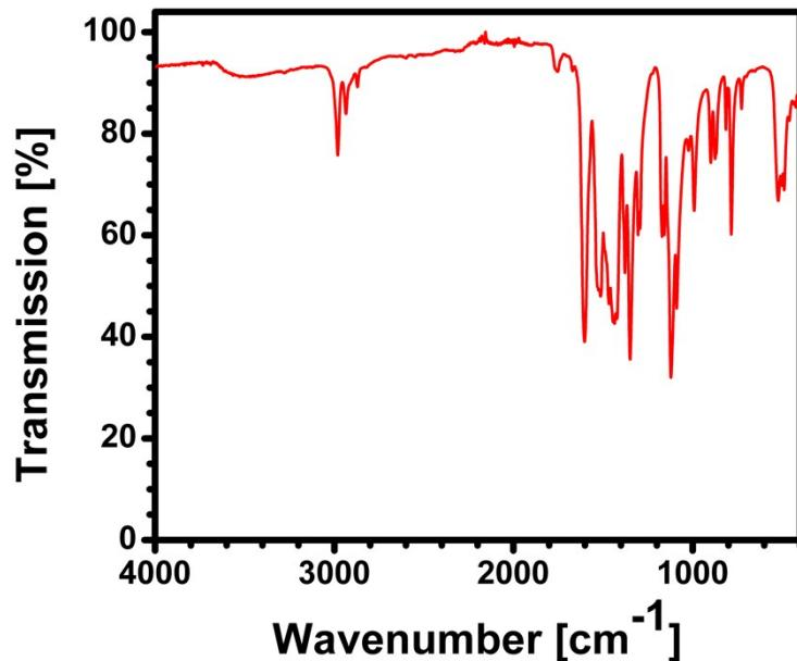
Fig. S9: FTIR-spectrum of tris[(diethyl-2-nitromalonato)aluminum(III)].
