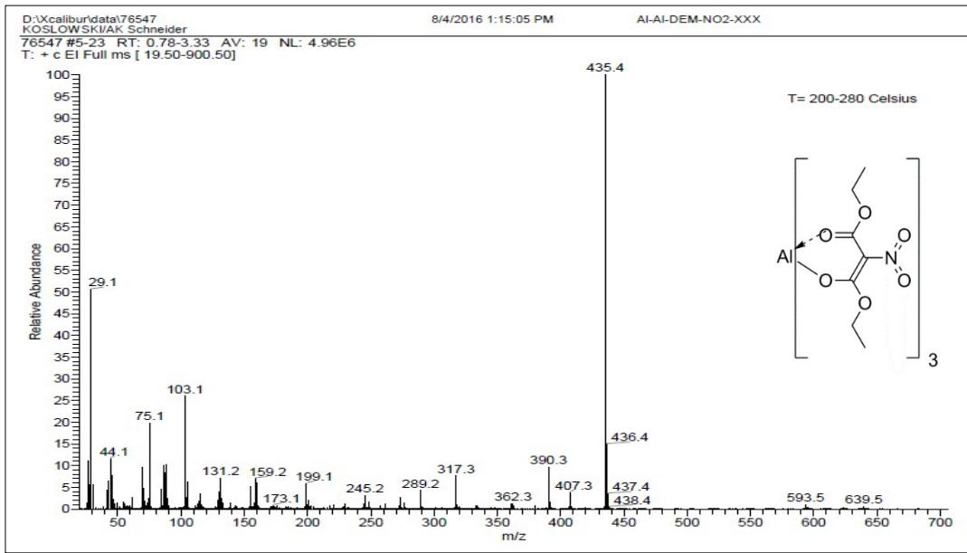
**Fig. S2: Mass spectrum (MS-EI) of tris[(diethyl-2-nitromalonato)]aluminum(III) (overview).**
