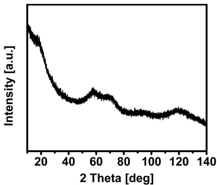
Fig. S10: XRD of empty crucible.
