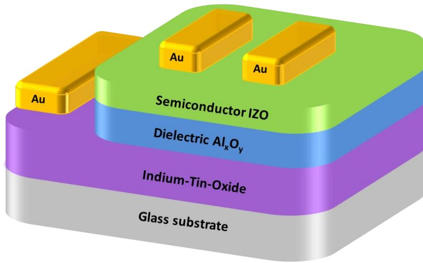
Fig. S14: Schematic representation of the device geometry of the fabricated thin film transistor.
