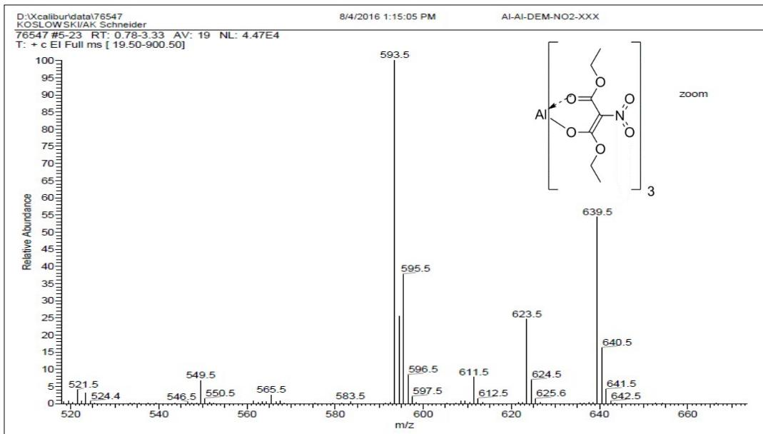
**Fig. S3: Mass spectrum (MS-EI) of tris[(diethyl-2-nitromalonato)]aluminum(III) (zoom-in).**
