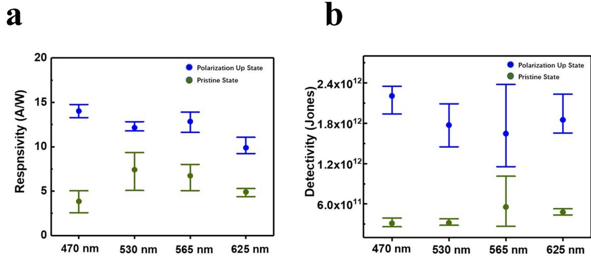
**Figure S3.** a) Responsivity and b) Detectivity of the devices at different wavelengths under pristine and “up” state.
