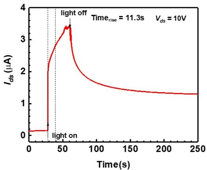
**Figure S4.** Light on-off character of the reference device with  $V_{ds} = 10\text{ V}$ . The photo switching behavior was tested under 470 nm wavelength with intensity  $155\ \mu\text{W cm}^{-2}$ .
