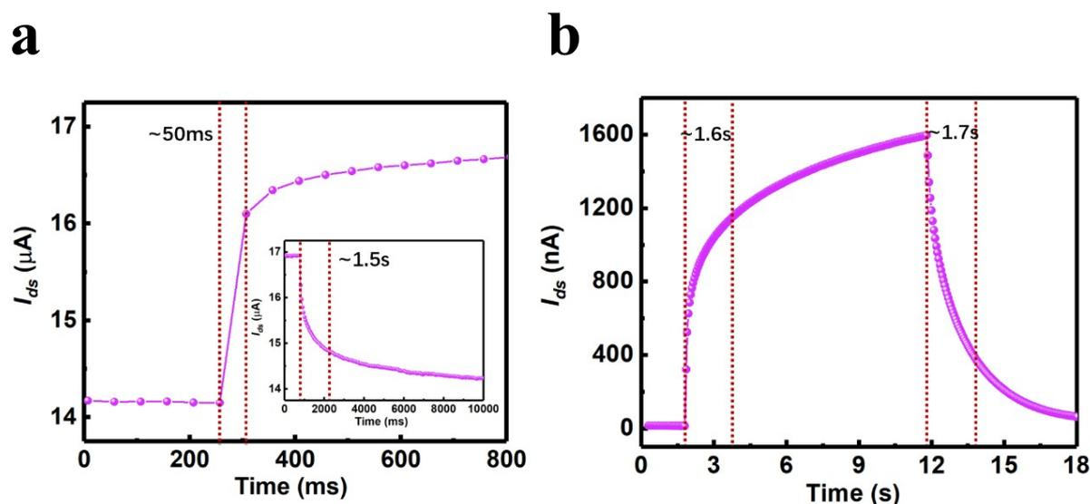
**Figure S5.** a) Enlarge views of the photo-switching behaviors of device under “down” state at intensity  $155 \mu\text{W cm}^{-2}$ . b) An enlarge view of the photo-switching behaviors of device under “up” state at intensity  $155 \mu\text{W cm}^{-2}$ .
