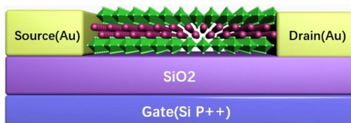
**Figure S1.** Schematic structure of reference devices. The devices own the same parameters as the ferroelectric devices except the dielectric layer changing from P(VDF-TrFE) (250 nm) to SiO<sub>2</sub> (285 nm).
