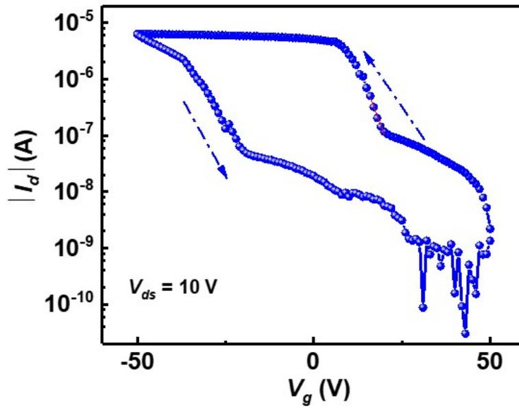
**Figure S2.** Transfer characteristic curves with  $V_{ds} = 10$  V of the reference device under dark condition.
