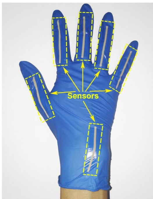
Figure S10. Optical photograph of intelligent glove.
