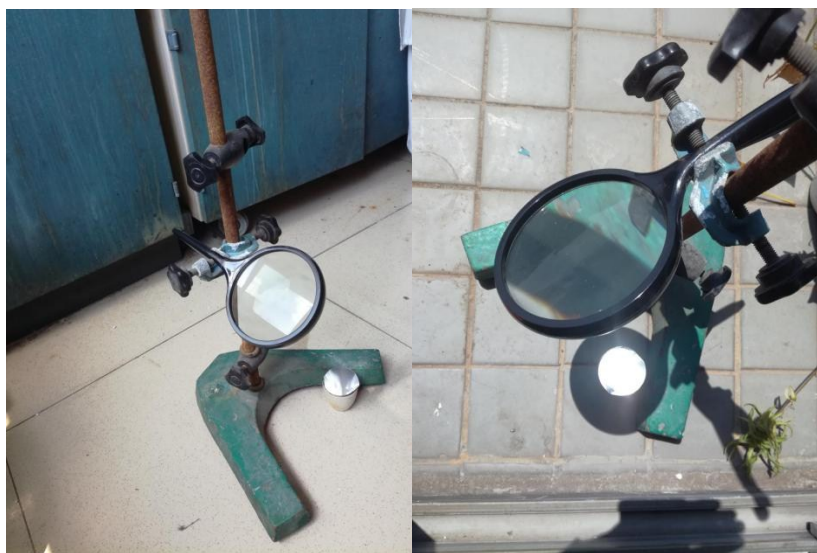
Figure S2 Experimental set-up for concentration solar radiation reaction.
