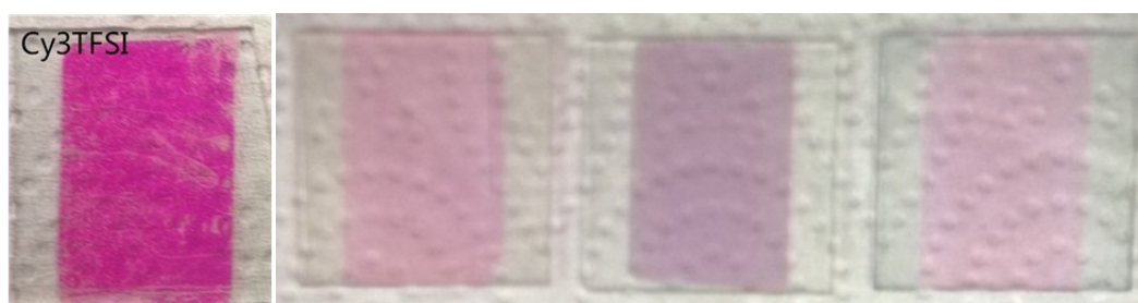
Figure S2. Visual results of the evaporated Cy3TFSI films on glass, ITO/TiO 2 , ITO/MoO 3 and ITO/PEDOT:PSS substrates (left to right).
