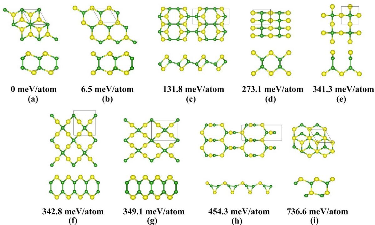
**Figure S1.**  $(\text{B}_2\text{S}_2)_x$  ( $x = 1$  and  $2$ ) monolayers with lower energy searched by the CALYPSO code. The relative energies with respect to the lowest one are calculated by PBE functional. The yellow and green balls represent sulphur and boron atoms, respectively. The black frames are boundaries of primitive cells.
