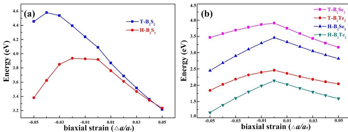
**Figure S4.** (a) Bandgaps as a function of biaxial strain obtained for T- (blue line) and H- $B_2S_2$  (red line) monolayers. (b) Bandgaps for T- $B_2Se_2$  (pink line), H- $B_2Se_2$  (blue line), T- $B_2Te_2$  (red line) and H- $B_2Te_2$  (dark green line) monolayers. All the results are calculated by HSE functional.
