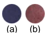
Fig. S6. The colorimetric response of PDA/CNC@chitosan films: (a) control and (b) after exposure to ammonia at -20°C for 3 h.
