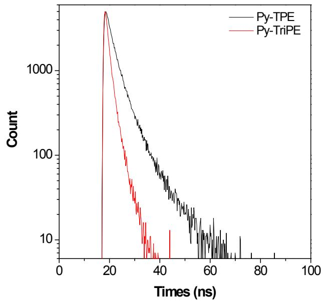
**Figure S13.**Fluorescence decays of **Py-TPE** and **Py-TriPE**in the solid state.
