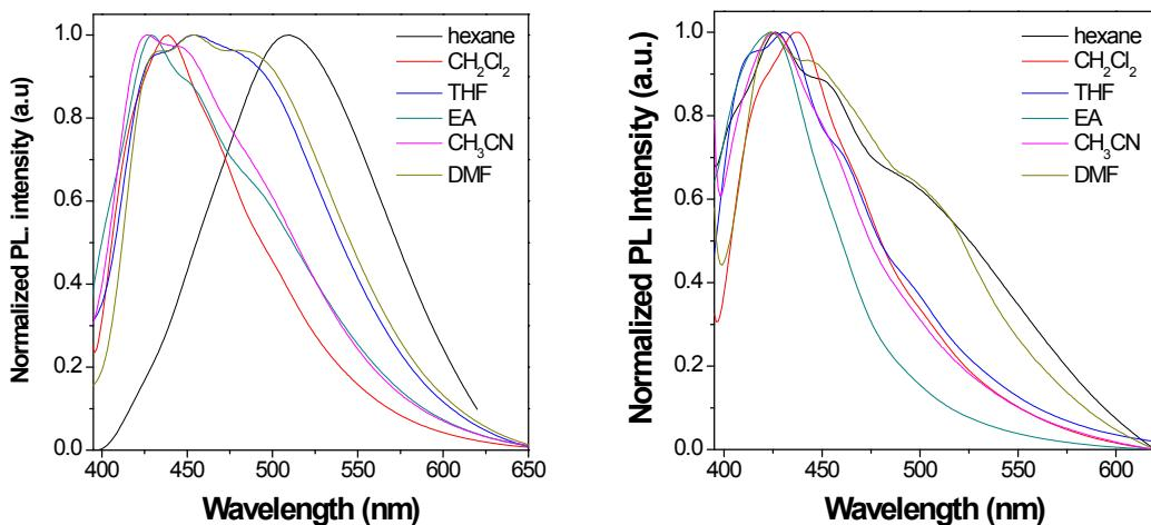
**Figure S12.** Fluorescence spectra of Py-TPE and Py-TriPE recorded in six different solvents (hexane, dichloromethane, tetrahydrofuran, ethyl acetate, acetonitrile and N,N-dimethylformamide) at  $\sim$ 10–5 M and 25 °C.
