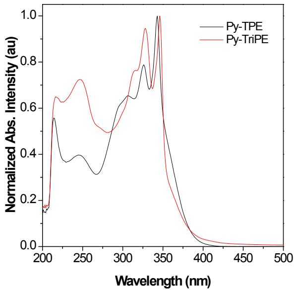
**Figure S7** Normalized UV-vis absorption spectra of **Py-TPE** and **Py-TriPE** recorded in THF solutions at  $\sim 10^{-5}$  M at 25 °C.
