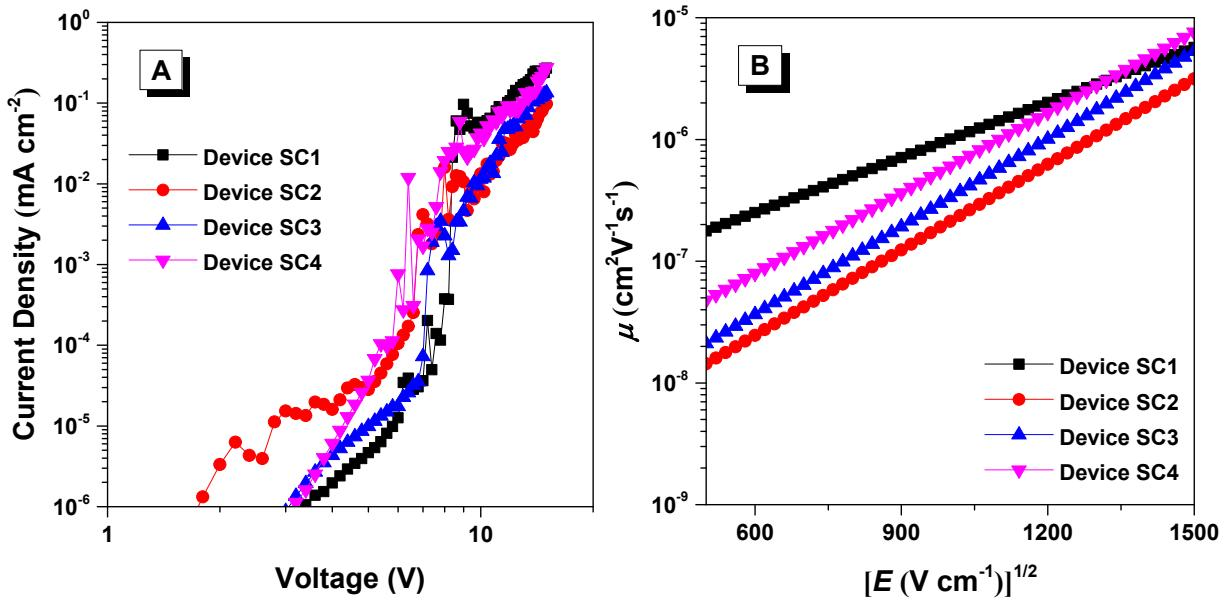
**Figure S19.(A)** Double logarithmic plots of current density ( $J$ ) vs applied voltage ( $V$ ) of device SC1-4. Configuration, device SC1: ITO/Py-TPE (80 nm)/TAPC (10 nm)/Al, device SC2: ITO/TmPyPB(10nm)/Py-TPE (80 nm)/LiF (1 nm)/Al, device SC3: ITO/Py-TriPE (80 nm)/TAPC (10 nm)/Al, device SC4: ITO/TmPyPB(10 nm)/Py-TriPE (80 nm)/LiF (1 nm)/Al.(B) Electric field-dependent hole and electron mobilities ( $\mu$ ) of Py-TPE and Py-TriPE.
