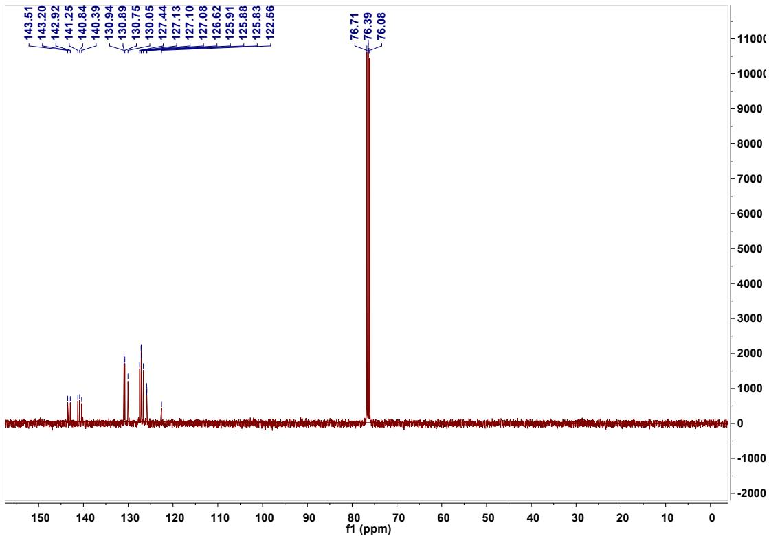
**Figure S4.** <sup>13</sup>C NMR spectrum of Py-TriPE (100 MHz, CDCl<sub>3</sub>, 293 K).
