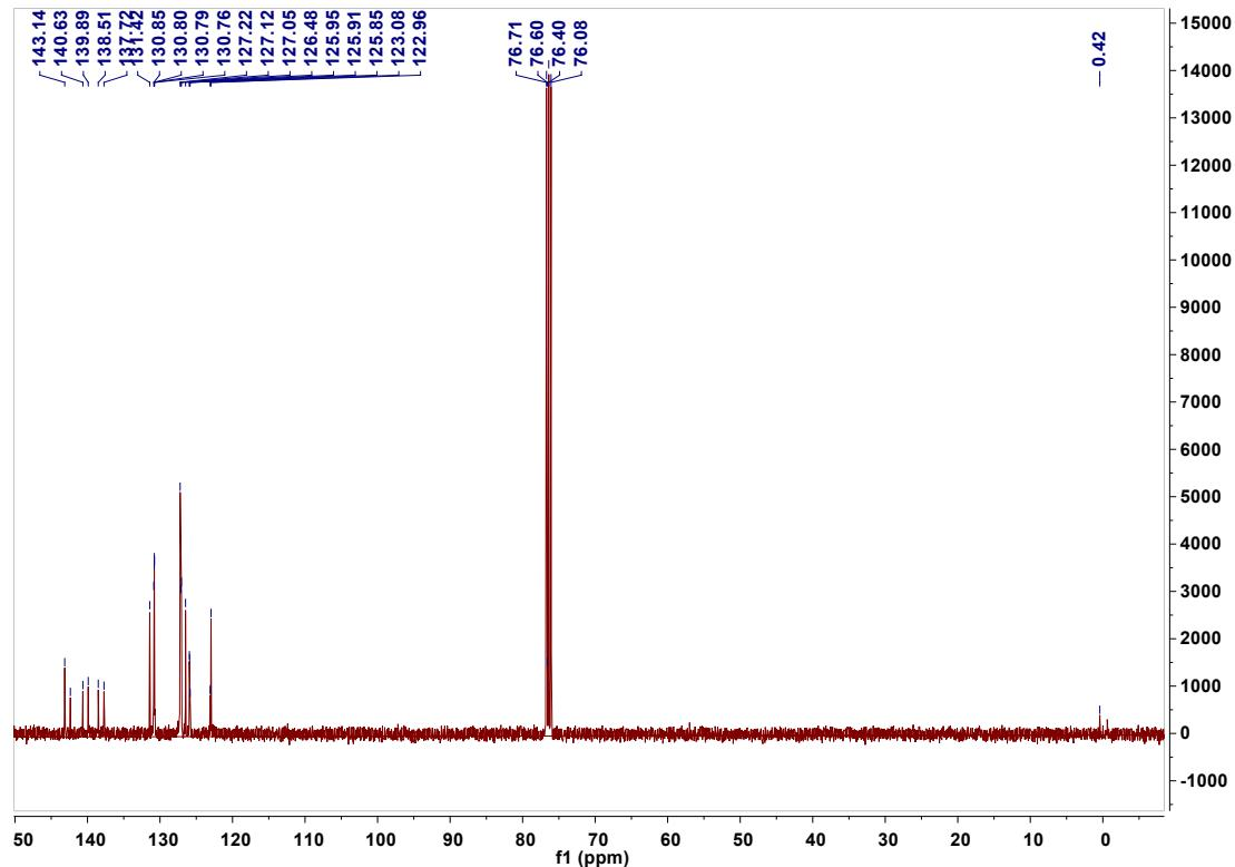
**Figure S2.** <sup>13</sup>C NMR spectrum of Py-TPE (100 MHz, CDCl<sub>3</sub>, 293 K).
