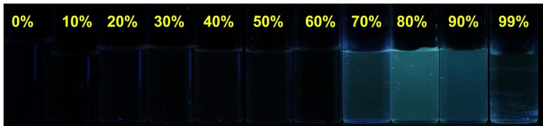
**Figure S10.** Fluorescent photographs of Py-TriPE in THF/water mixtures from  $f_w = 0$ , to 99% taken under UV illumination ( $\lambda_{ex} = 365$  nm).
