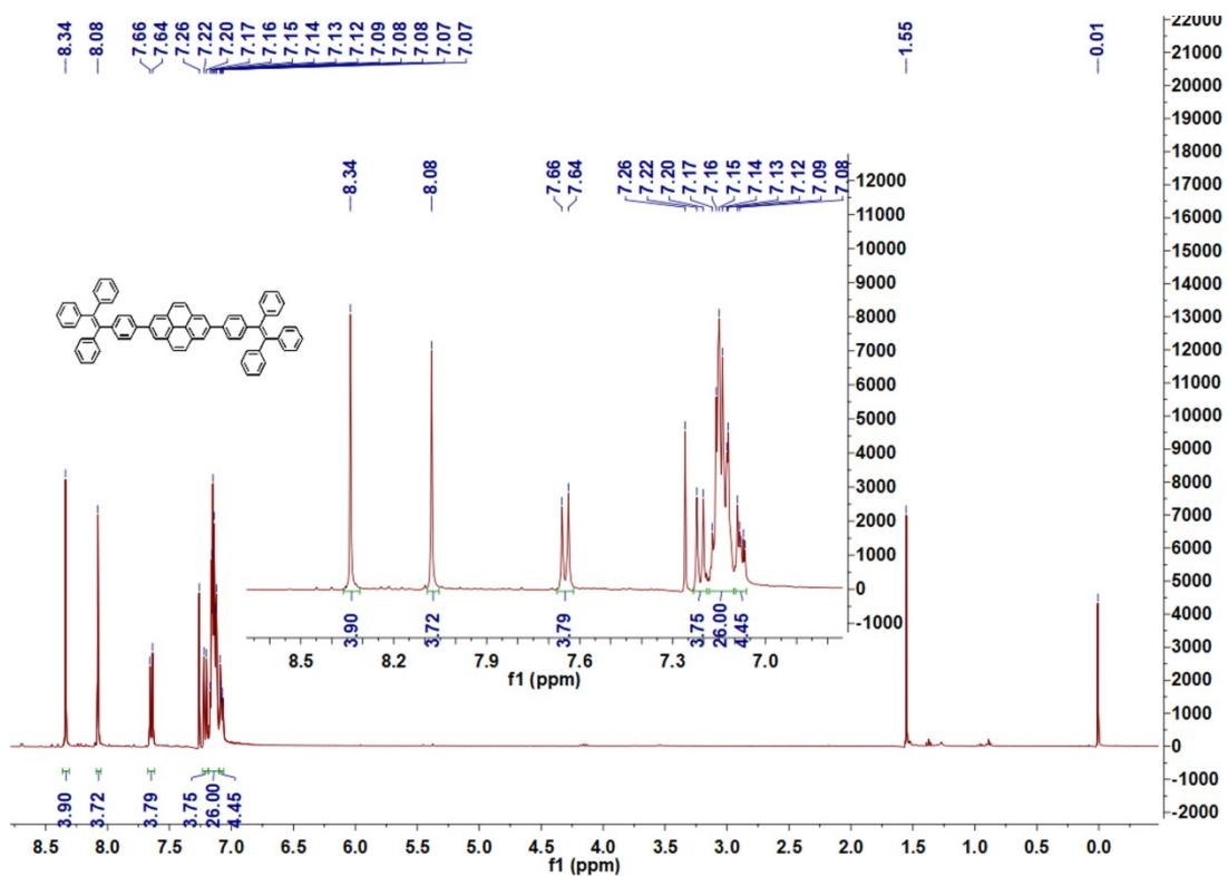
**Figure S1.** <sup>1</sup>H NMR spectrum of Py-TPE (400 MHz, CDCl<sub>3</sub>, 293 K).
