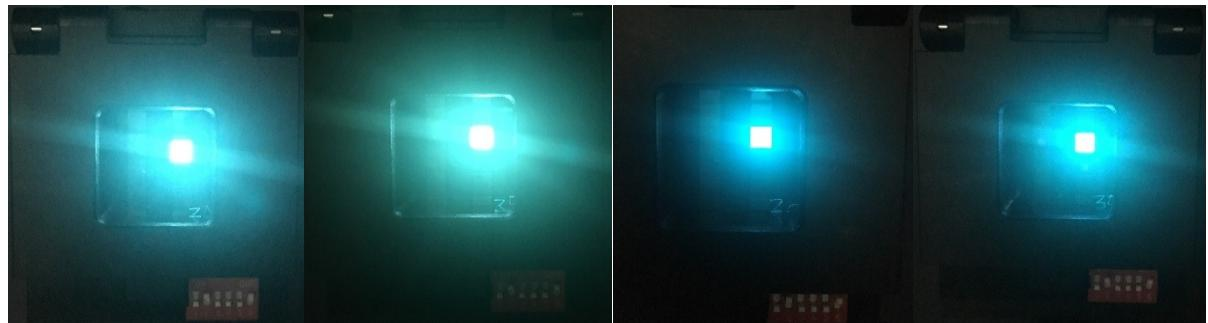
**Figure S16.** Photos of the OLED devices, using **Py-TPE** as host material in EL devices **1-2** and **Py-TriPE** as host material in EL devices **3-4**.
