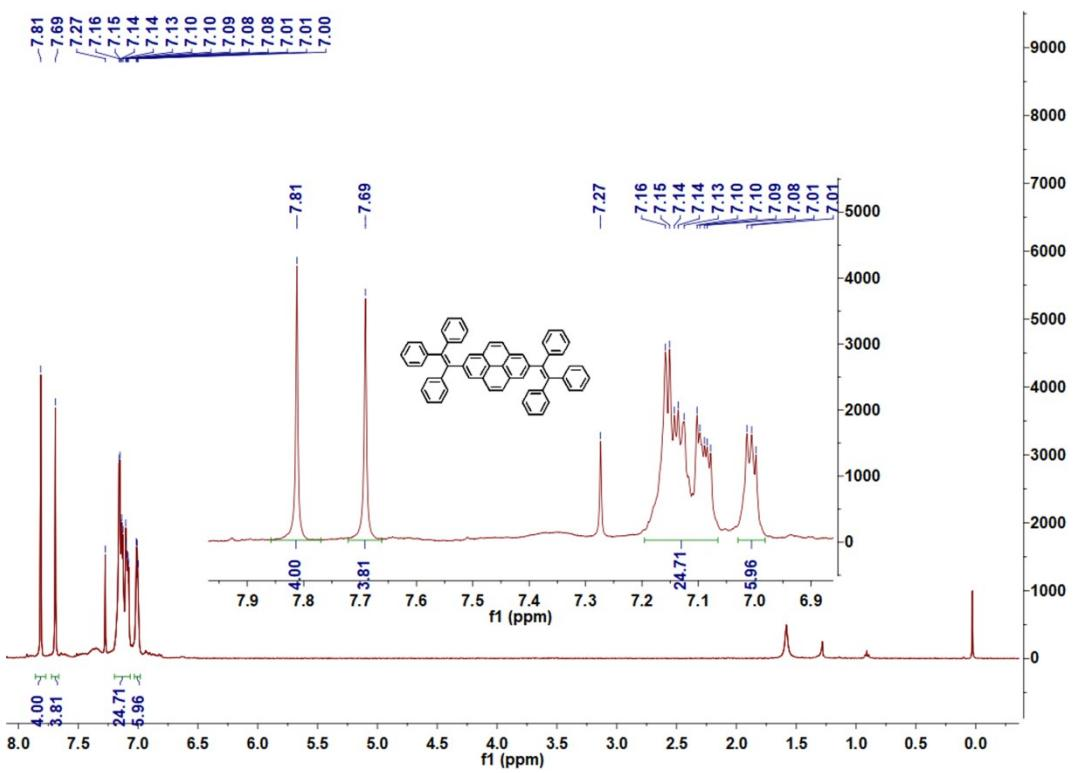
**Figure S3.** <sup>1</sup>H NMR spectrum of Py-TriPE (400 MHz, CDCl<sub>3</sub>, 293 K).
