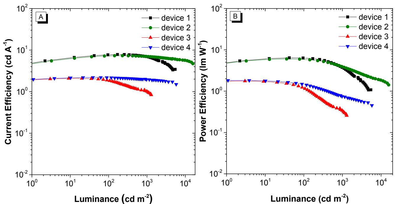
**Figure S17.** (A) Luminance–Current efficiency curves and (B) Luminance–power efficiency curves for non-doped OLED devices, using **Py-TPE** as host material in EL devices **1-2** and **Py-TriPE** as host material in EL devices **3-4**.
