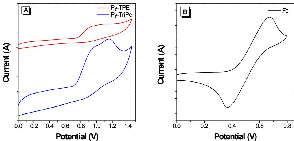
**Figure 14.** CV of (A) Py-TPE and Py-TriPE and (B) ferrocene recorded from a  $\text{CH}_2\text{Cl}_2$  solution on a platinum plate electrode at a scan rate of  $100 \text{ mV}\cdot\text{s}^{-1}$ .
