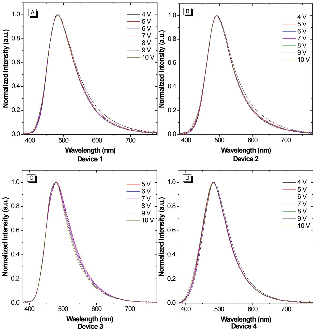
**Figure S18.** EL spectra of the device using Py-TPE and Py-TriPE as emitters at various voltages.
