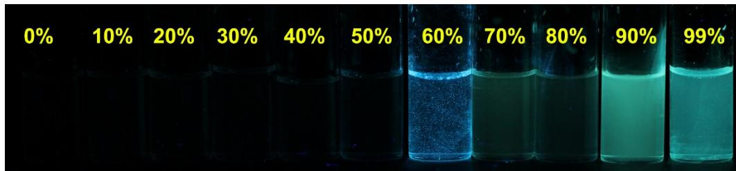
**Figure S9.** Fluorescent photographs of Py-TPE in THF/water mixtures from  $f_w = 0$ , to 99% taken under UV illumination ( $\lambda_{ex} = 365$  nm).
