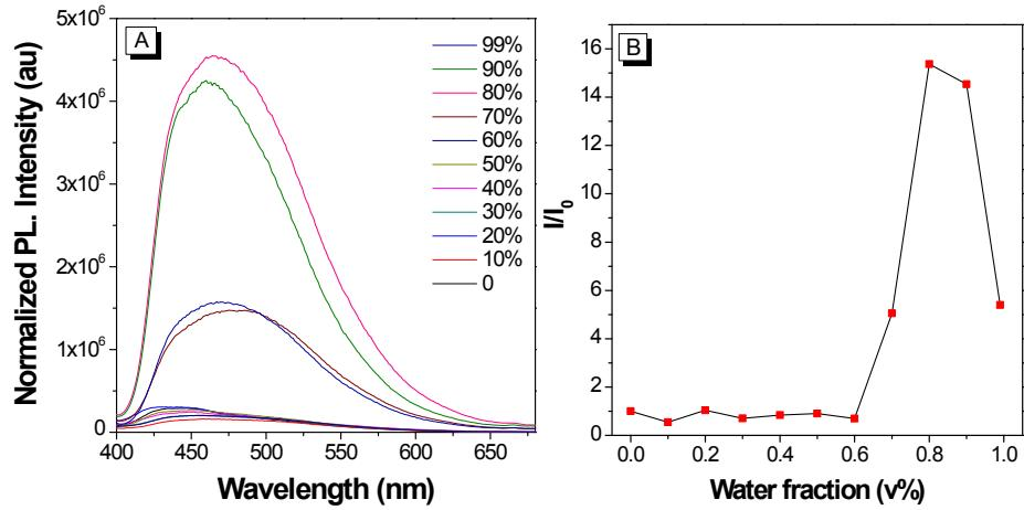
**Figure S8.** (A) PL spectra of **Py-TriPE** in THF/water mixture with different water fractions ( $f_w$ ). (B) Plot of  $I/I_0$  versus the composition of THF/water mixture of **Py-TriPE**, where  $I_0$  is the PL intensity in pure THF solution at 465 nm.
