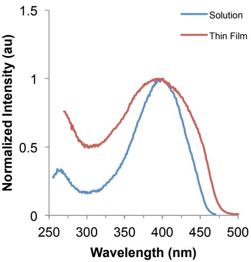
Absorbance (top left), emission (bottom left), and excitation (bottom right) of **4-BT-F5** in solution and as a drop cast thin film.
