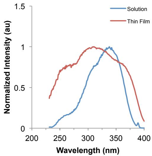
Absorbance (top left), emission (bottom left), and excitation (bottom right) of **4-BP-F5** in solution and as a drop cast thin film.
