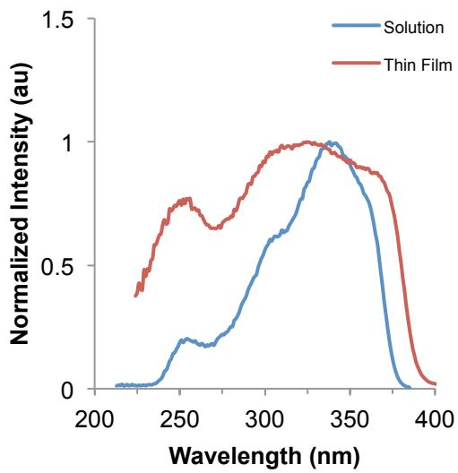
Absorbance (top left), emission (bottom left), and excitation (bottom right) of **3-PE-H5** in solution and as a drop cast thin film.
