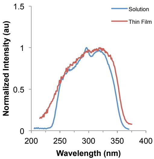
Absorbance (top left), emission (bottom left), and excitation (bottom right) of **4-TMBP-F5** in solution and as a drop cast thin film.
