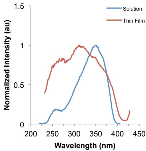
Absorbance (top left), emission (bottom left), and excitation (bottom right) of **4-PE-F5** in solution and as a drop cast thin film.
