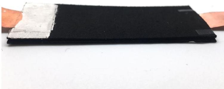
**Fig. S8.** Digital photo of sensory skin device comprised of two sensory skins (60 mm × 25 mm) placed face-to-face.
