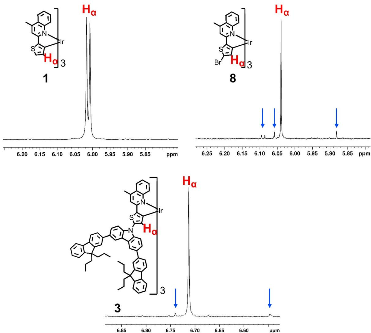
**Figure S3** <sup>1</sup>H NMR investigation of the regioisomers formed during the bromination of **1** and carry through to dendrimer **3**. The thiophenyl proton alpha to the Ir-C bond ( $H_\alpha$ ) was used as the diagnostic peak. The signals corresponding to the  $H_\alpha$  of the major isomer are labelled in red. The small signals corresponding to the minor regioisomer(s) are indicated by blue arrows.
