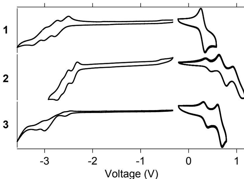
**Figure S6** Cyclic voltammograms of red-emitting iridium(III) complexes versus Fc/Fc<sup>+</sup> redox couple. Oxidations were performed in anhydrous dichloromethane while reductions were in anhydrous tetrahydrofuran. Tetrabutylammonium perchlorate was utilized as the electrolyte with a glassy carbon working electrode, platinum counter electrode and silver/silver(I) nitrate in acetonitrile reference electrode.
