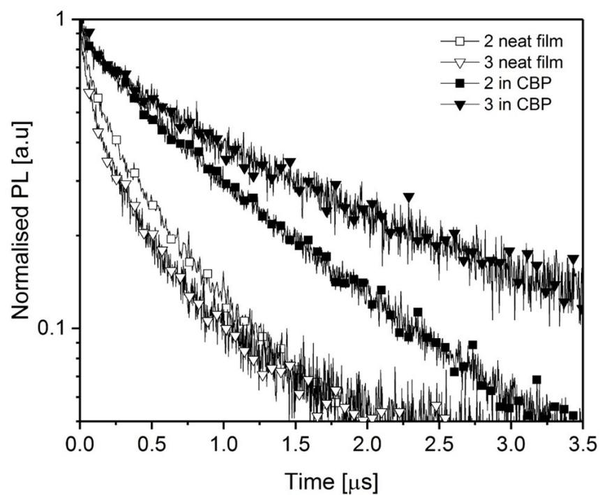
**Figure S7** TCSPC decays of a) **1** (at 589 nm), **2** and **3** (both at 609 nm) in toluene and as neat films, and b) at 610 nm for the neat **2** and **3**, and 10 wt% dendrimer:CBP blend films. Excitation wavelength = 372 nm.
