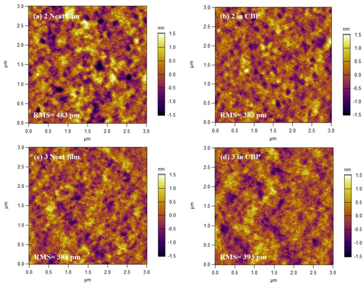
**Figure S5** AFM images showing the surface topology of the films. Neat and blend film of **2** [(a) and (b), respectively] and neat and blend of **3** [(a) and (b), respectively].
