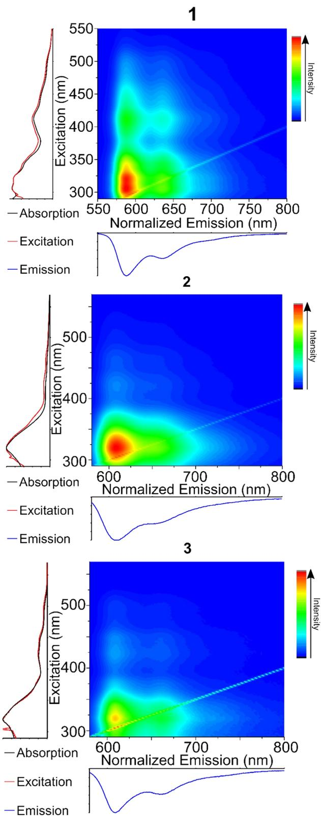
**Figure S8** Emission versus excitation contour plots of **1**, **2**, and **3** in solution (toluene). One-dimensional emission, excitation and adsorption spectra are shown as axis projections for comparison.
