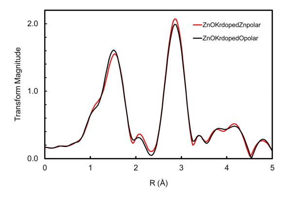
S1 Fig. 1 X-ray absorption spectra and transform magnitude for Zn in the most heavily implanted polar ZnO films.
