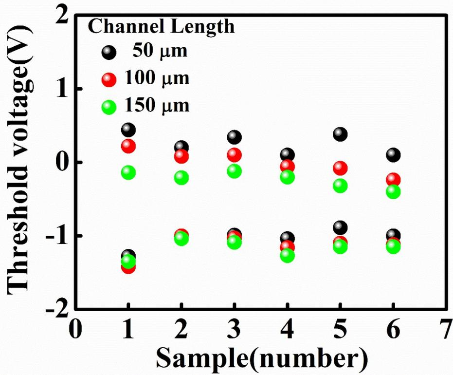
**Fig. S5.**  $V_{th}$  for various samples with different channel lengths after the +6 V, 100  $\mu\text{s}$  program, -4 V, 100  $\mu\text{s}$  erase. Each device has an  $\text{Al}_2\text{O}_3$  (20 nm)/ PaMS (10 nm) gate stack.
