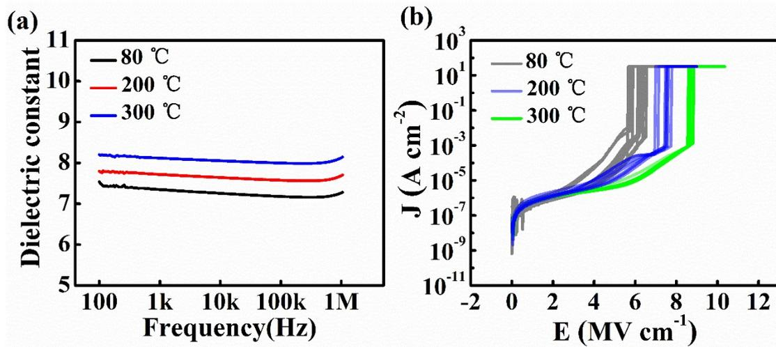
**Fig. S7.** Electrical properties of Al<sub>2</sub>O<sub>3</sub> films fabricated at various temperatures. (a) Dielectric constant as a function of frequency. (b) Leakage current as a function of electric field.
