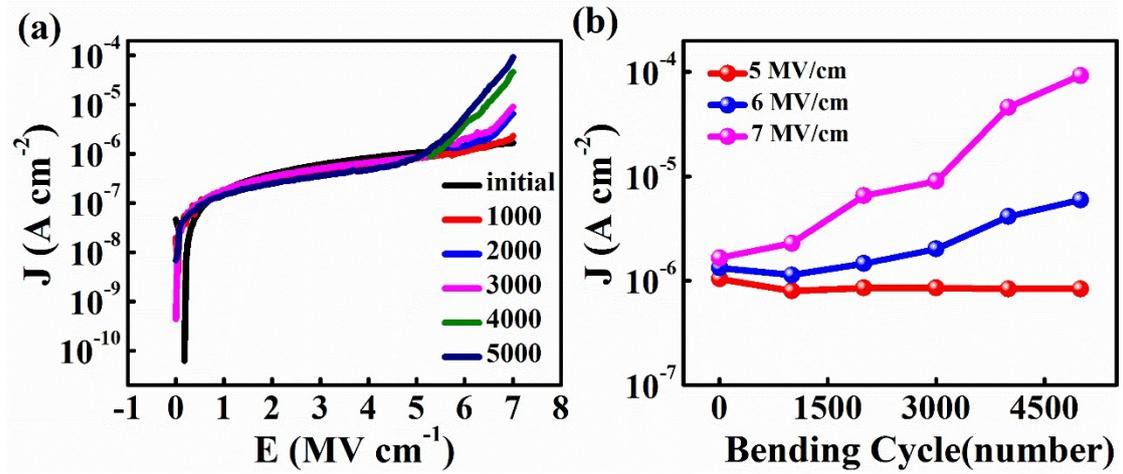
**Fig. S11.** Mechanical-bending properties of ALD-grown 20 nm  $\text{Al}_2\text{O}_3$  film. (a) Leakage current as a function of electric field for Au/ $\text{Al}_2\text{O}_3$ /Au after various numbers of bending cycles at a fixed bending radius of 10 mm. (b) Leakage current density as a function of number of bending cycles with a bending radius of 10 mm and for various electric fields.
