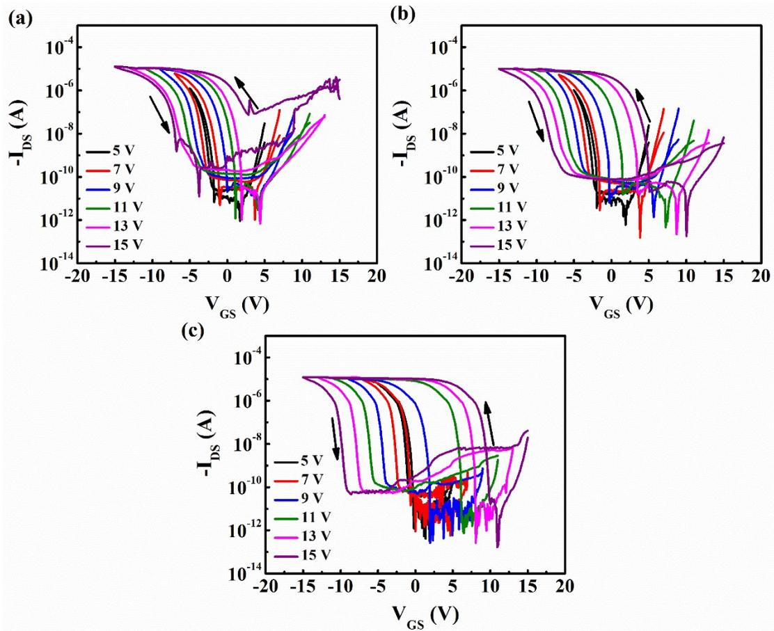
**Fig. S9.**  $I_{DS}$ - $V_{GS}$  hysteresis characteristics of OFET memory devices with  $Al_2O_3$  films fabricated at various temperatures: (a) 80 °C; (b) 200 °C; (c) 300 °C. The memory performance is lower for  $Al_2O_3$  devices deposited at lower temperatures.
