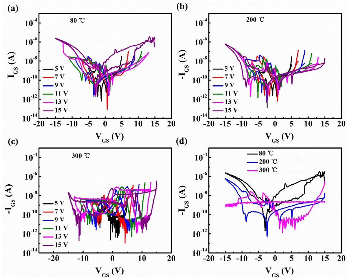
**Fig. S10.** Characteristics of gate leakage current of OFET memory devices with Al<sub>2</sub>O<sub>3</sub> films fabricated at various temperatures: (a) 80 °C; (b) 200 °C; (c) 300 °C. (d) Comparison of gate leakage current during voltage scans between  $\pm 15$  V. A higher gate leakage current occurs for Al<sub>2</sub>O<sub>3</sub> devices deposited at lower temperatures.
