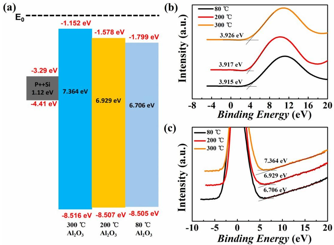
**Fig. S8.** (a) Band alignments of the Al<sub>2</sub>O<sub>3</sub> dielectric with different deposition temperatures from the XPS; (b) XPS valence band spectra of Al<sub>2</sub>O<sub>3</sub>/Si with different deposition temperatures; (c) XPS O 1s electron energy loss spectra of Al<sub>2</sub>O<sub>3</sub>/Si with different deposition temperatures
