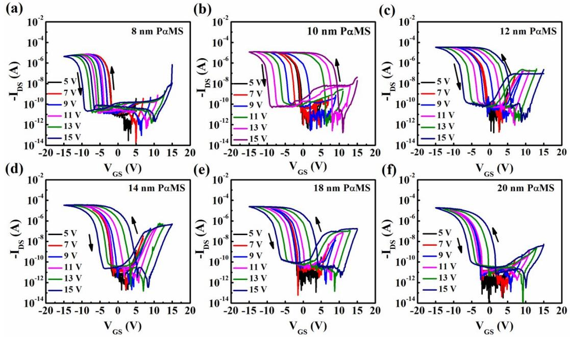
**Fig. S1.** Typical  $I_{DS}$ - $V_{GS}$  characteristics for various  $V_{GS}$  sweeping ranges for OFET memory devices with various PaMS thicknesses: (a) 8 nm; (b) 10 nm; (c) 12 nm; (d) 14 nm; (e) 18 nm; (f) 20 nm. The  $Al_2O_3$  is 20 nm thick and  $V_{DS} = -3$  V.
