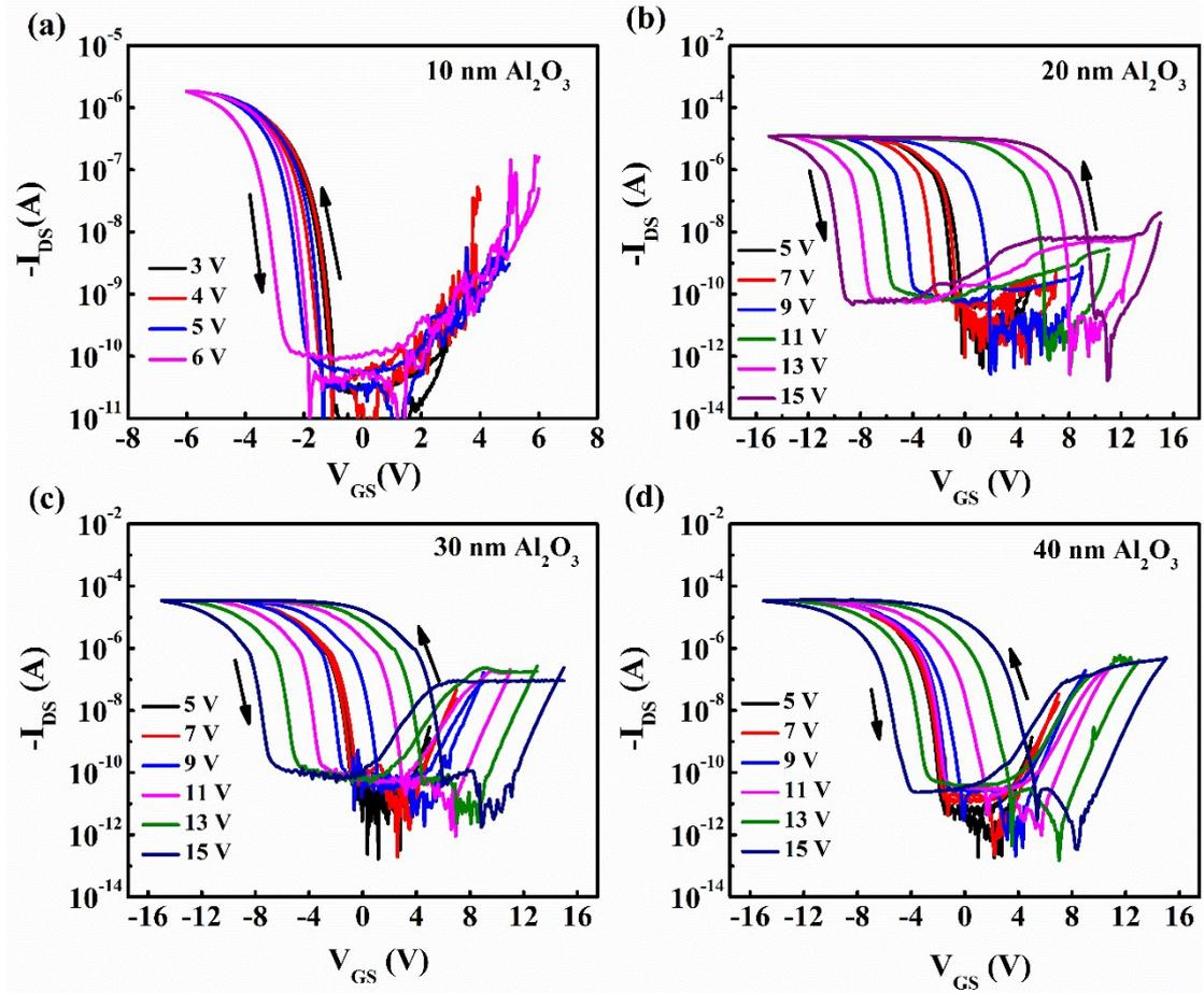
**Fig. S2.** Typical  $I_{DS}$ - $V_{GS}$  characteristics at different  $V_{GS}$  sweeping ranges for OFET memory devices with various  $Al_2O_3$  thicknesses: (a) 10 nm; (b) 20 nm; (c) 30 nm; (d) 40 nm. P $\alpha$ MS is 10 nm thick and  $V_{DS} = -3$  V.
