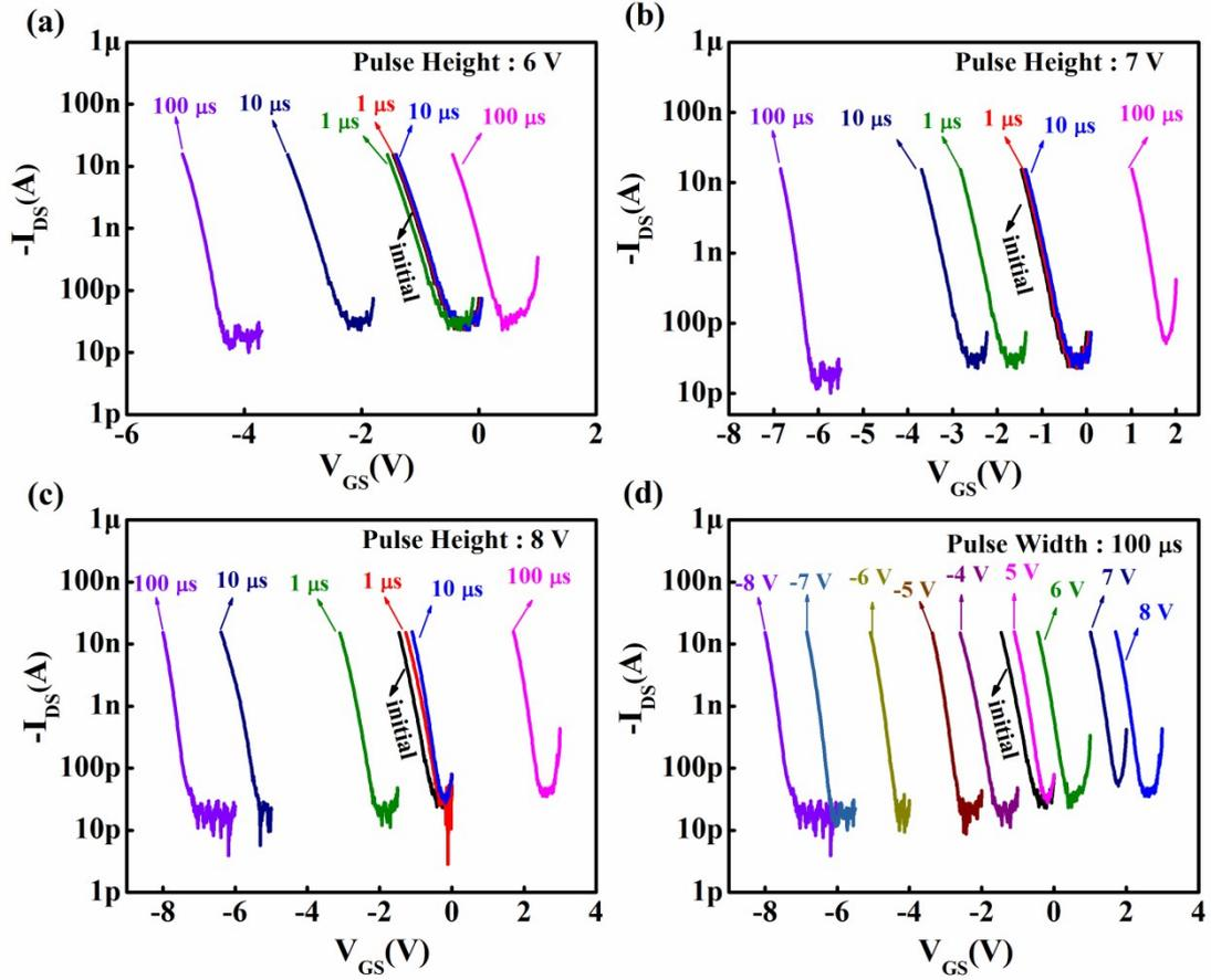
**Fig. S4.** Typical  $I_{DS}$ - $V_{GS}$  curves for reading out  $V_{th}$  values for OFET memory with  $Al_2O_3(20\text{ nm})/PaMS(10\text{ nm})$  gate stack: (a) pulse height is 6 V; (b) pulse height is 7 V; (c) pulse height is 8 V; (d) pulse width is 100  $\mu s$ .  $V_{DS} = -3\text{ V}$  for all measurements.
