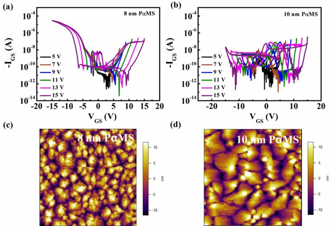
**Fig. S3.** Gate leakage current Characteristics of OFET memory devices with different thickness PαMS films: (a) 8 nm, (b) 10 nm. AFM surface topographies of pentacene film on different thickness PαMS films: (c) 8 nm, (d) 10 nm.
