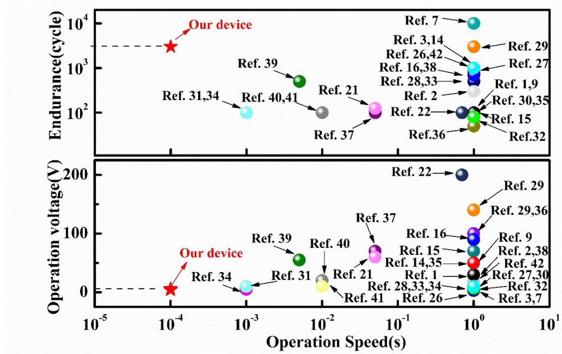
**Fig. S6.** Comprehensive comparison of operating voltage, operating speed, and endurance of proposed device with that of the representative flexible flash-type OTFT memory devices reported in recent years. The references here are from the main text.
