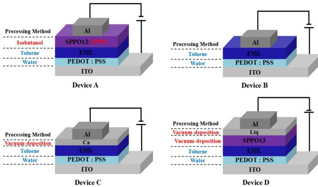
**Fig. S7.** Configuration and processing method of different blue devices: device A: solution-processed SPPO13:TPPO (8: 2, w/w) is used as EIL; device B: without EIL; device C: vacuum-deposited Ca is used as EIL; device D: vacuum-deposited SPPO13/Liq are used as ETL/EIL.
