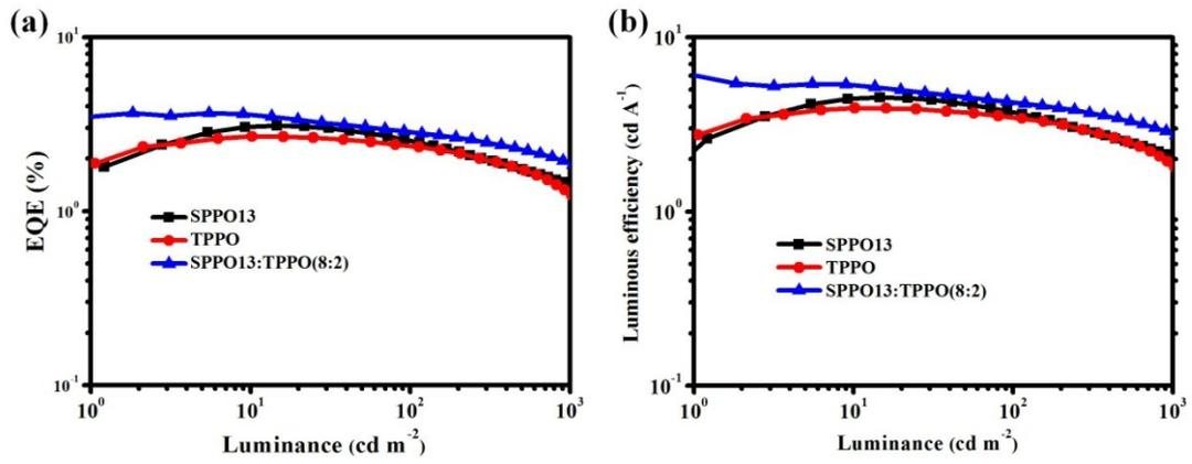
**Fig. S5.** Performance of blue devices with different electron injection layers (SPPO13, TPPO, and SPPO13: TPPO (8: 2, w/w)) (a) EQE as a function of luminance; (b) luminous efficiency as a function of luminance.
