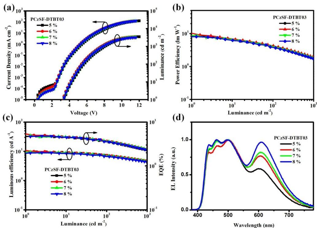
**Fig. S11.** Concentration tuning of red polymer PCzSF-DTBT03 (green and red polymers are doped into blue polymer as the EML, and the concentration of green polymer is 7 wt. %): (a) current density–voltage–luminance ( $J$ - $V$ - $L$ ) characteristics; (b) power efficiency as a function of luminance; (c) luminous efficiency and EQE as a function of luminance; (d) EL spectra.
