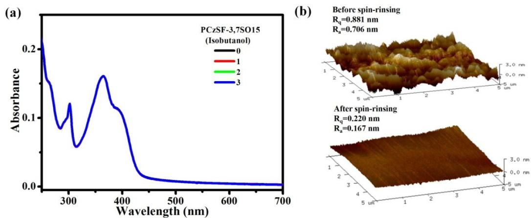
**Fig. S1.** UV-Vis absorption spectra for PCzSF-3,7SO15 film after different spin-rinsing time with isobutanol (a), and AFM images of PCzSF-3,7SO15 films before and after spin-rinsing with isobutanol (b).
