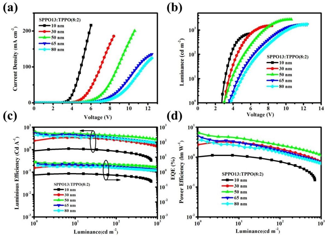
**Fig. S3.** Performance of blue devices with varying thickness of mixed EIL SPPO13:TPPO (8:2): (a) current density-voltage ( $J$ - $V$ ) characteristics; (b) luminance-voltage ( $L$ - $V$ ) characteristics; (c) luminous efficiency and EQE as a function of luminance; (d) power efficiency as a function of luminance.
