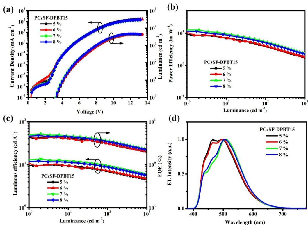
**Fig. S10.** Concentration tuning of green polymer PCzSF-DPBT15 (green polymer doped into blue polymer as the EML): (a) current density–voltage–luminance ( $J$ - $V$ - $L$ ) characteristics; (b) power efficiency as a function of luminance; (c) luminous efficiency and EQE as a function of luminance; (d) EL spectra.
