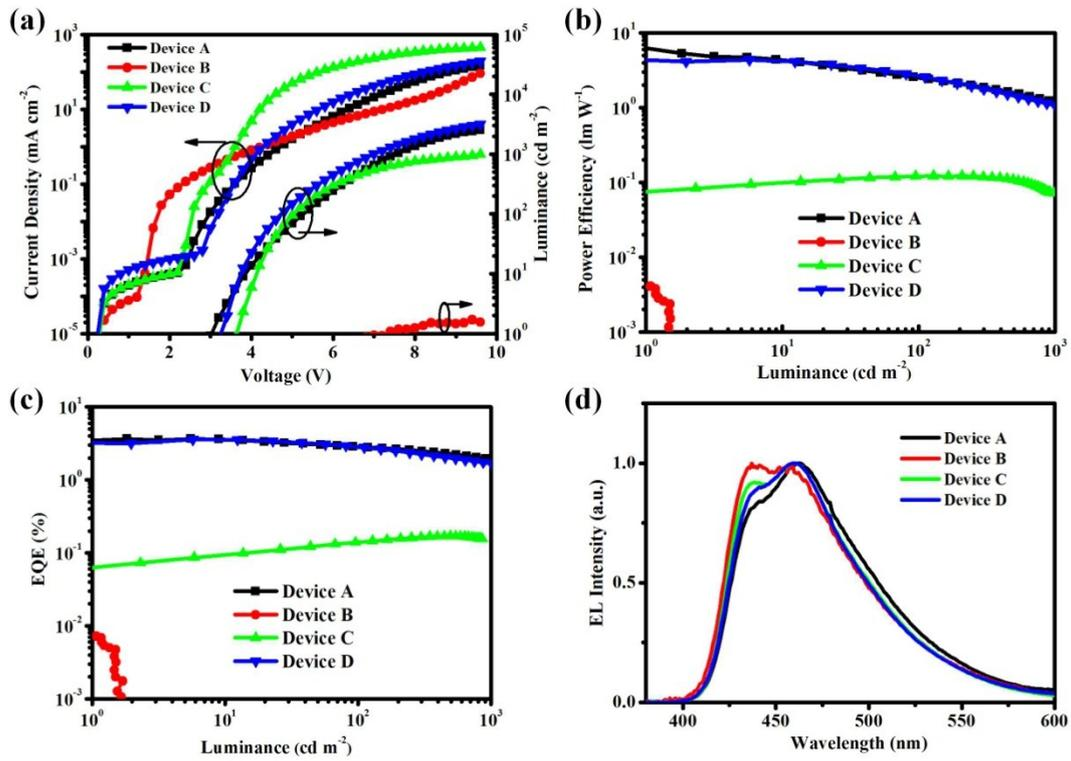
**Fig. S8.** Performance comparison of device A (SPPO13:TPPO (8: 2, w/w)), device B, device C and device D: (a) current density-voltage-luminance ( $J-V-L$ ) characteristics; (b) power efficiency as a function of luminance; (c) EQE as a function of luminance; (d) EL spectra.
