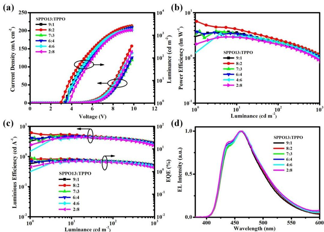
**Fig. S2.** Performance of blue devices with varying ratio between SPPO13 and TPPO
