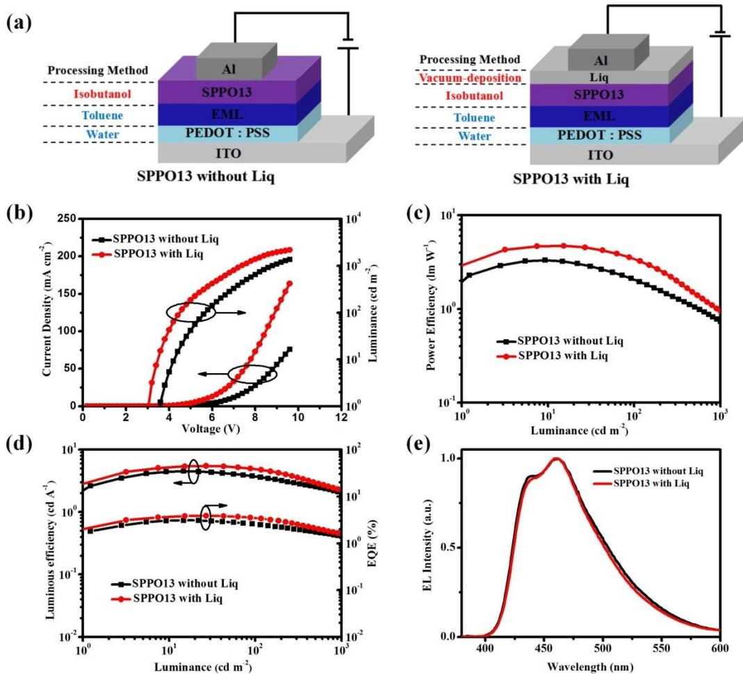
**Fig. S6.** Comparison between devices without Liq and with Liq: (a) device configuration of devices without Liq and with Liq; (b) current density–voltage–luminance ( $J-V-L$ ) characteristics; (c) power efficiency as a function of luminance; (d) luminous efficiency and EQE as a function of luminance; (e) EL spectra.
