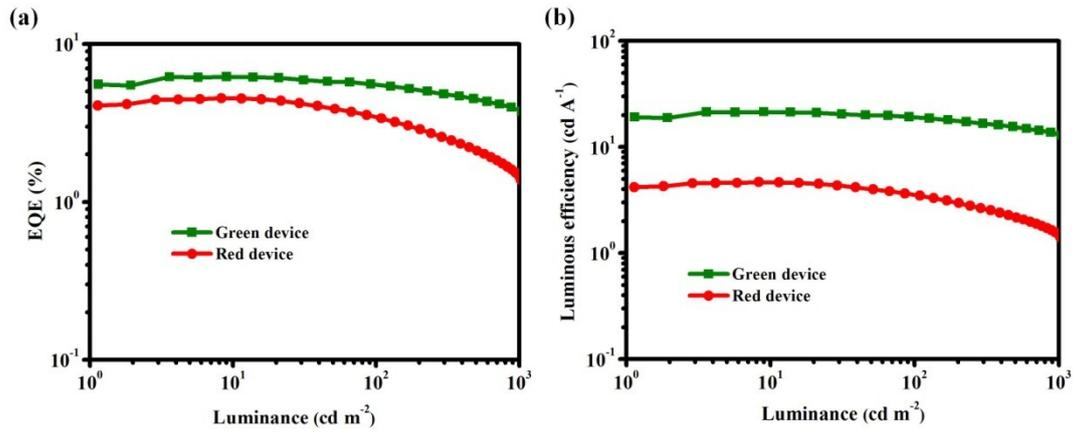
**Fig. S9.** EQE (a) and luminous efficiency (b) as a function of luminance for green and red devices with SPPO13: TPPO (8: 2, w/w) as electron injection layer.
