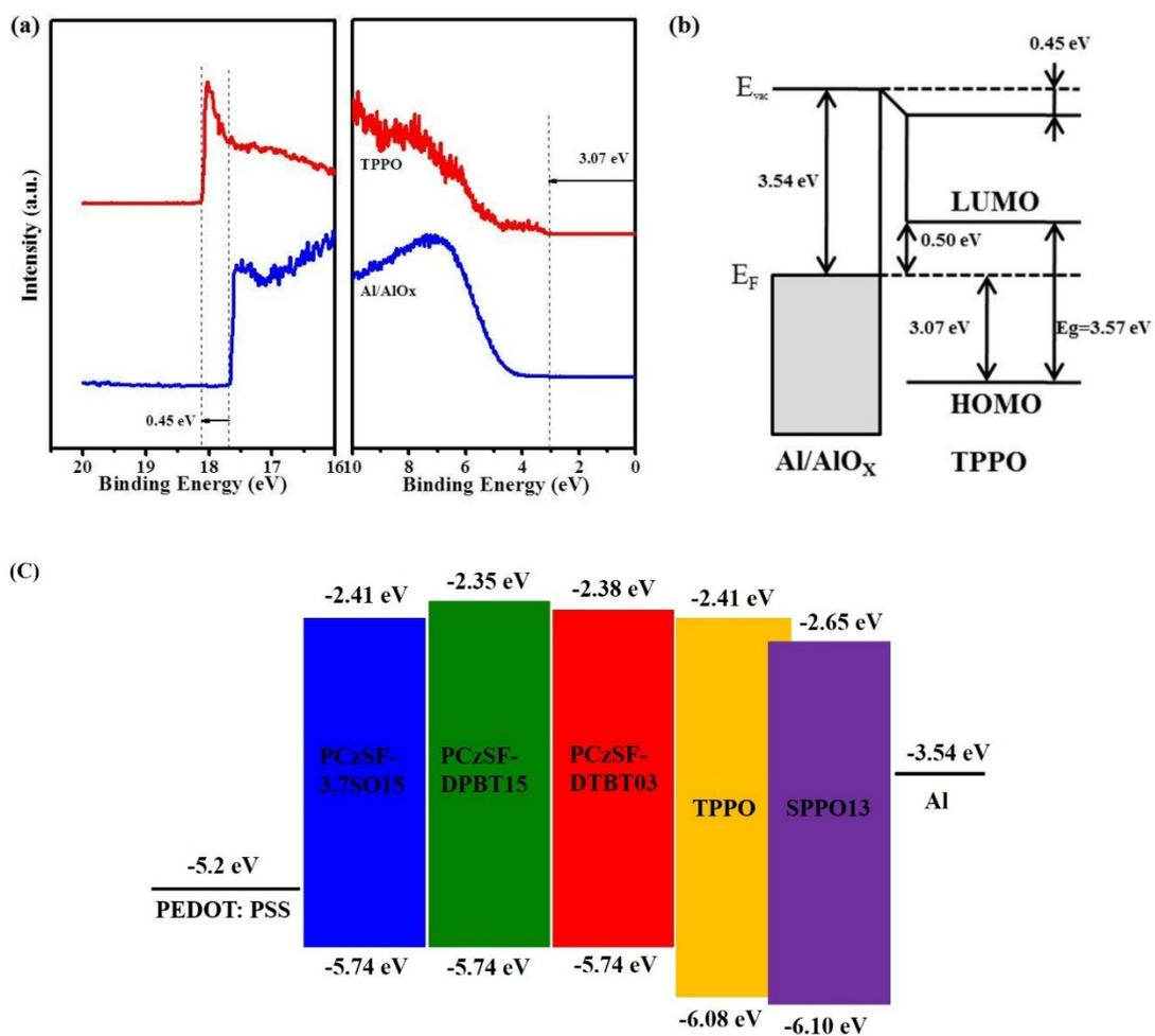
**Fig. S4.** UPS spectra of Al/TPPO (a); The corresponding energy diagram at the interfaces (b); Energy level alignment of the multi-layer PLEDs (c).
