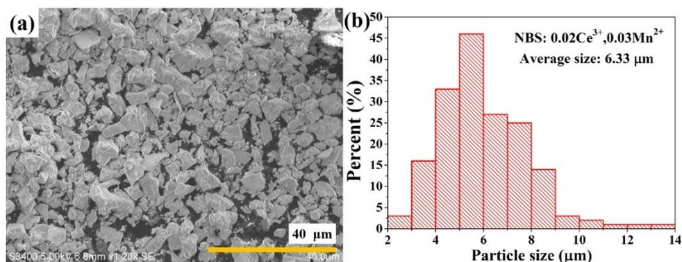
**Figure S2.** (a) SEM micrograph and (b) the particle size distribution of NBS:0.02Ce<sup>3+</sup>,0.03Mn<sup>2+</sup>.
