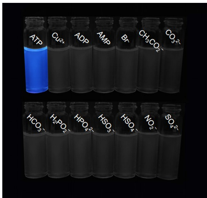
Fig. S9. Photos of TPE-COOH/Cu 2+ upon addition of various ions in HEPES buffer. [TPE-COOH/Cu 2+ ] = 1.0×10 -5 mol/L; [anion] = 2.0×10 -5 mol/L; \lambda_{\text{exc}} = 365 nm.
