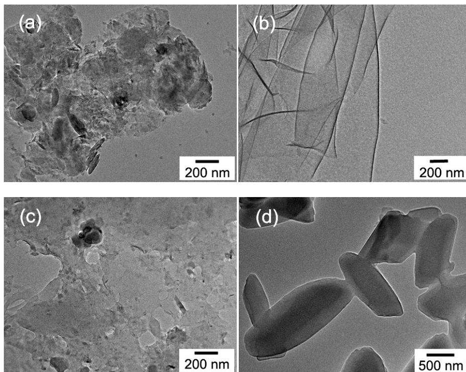
**Fig. S2** TEM images of samples obtained by dissolving PPs in water with different polymer concentrations ( $\text{mg mL}^{-1}$ ), where PPs were prepared with CA/LCy molar ratio being 2:1 at  $160\text{ }^{\circ}\text{C}$  for 1 h: (a) 0.005; (b) 2; (c) 16; (d) 32.
