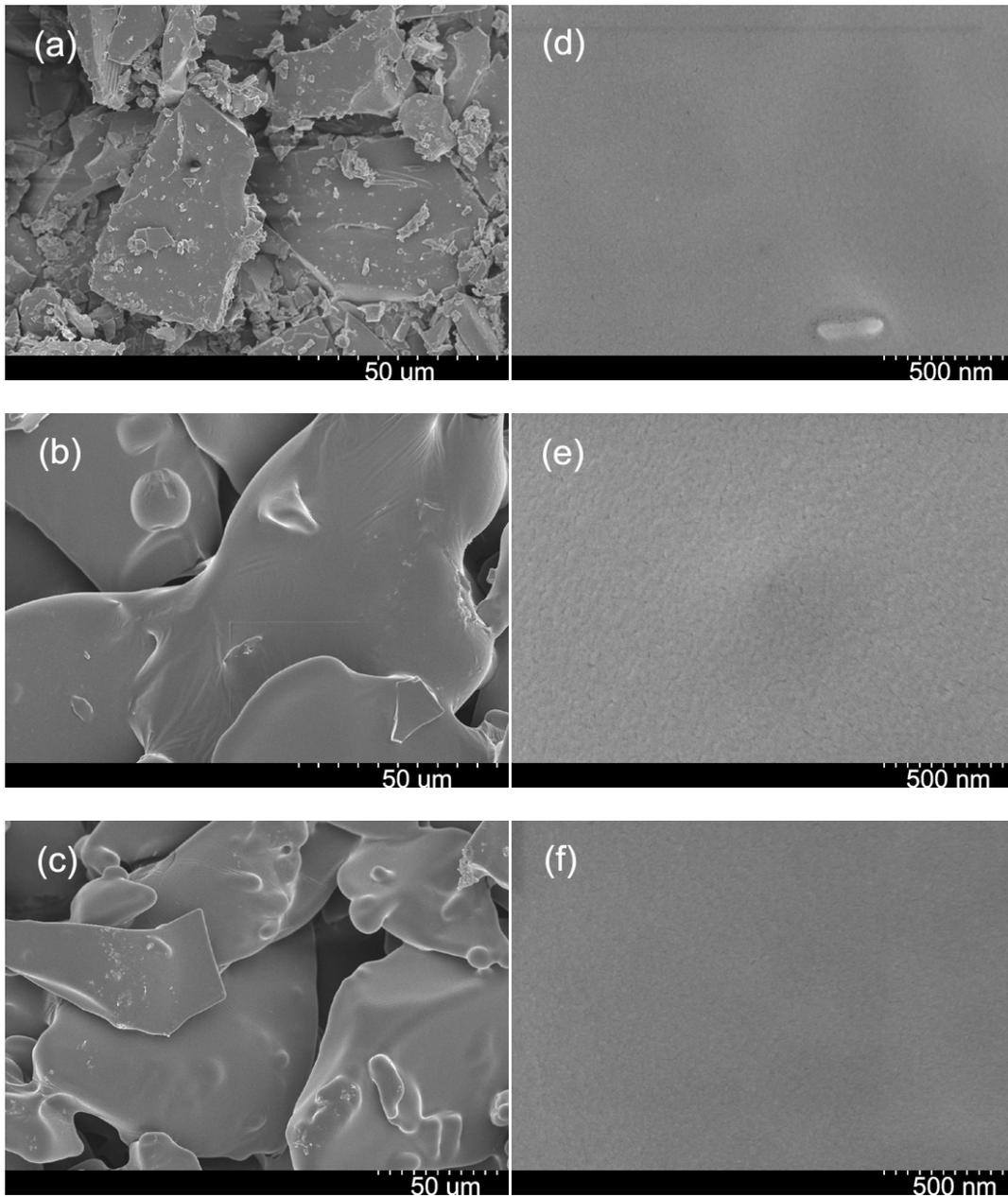
**Fig. S1** SEM images of PPs prepared with different CA/LCy molar ratios at 160 °C for 1 h: (a,d) 1:1; (b,e) 2:1; (c,f)
