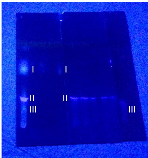
**Fig. S8** Photograph of the chromatoplate; I, II, and III marked in the figure denote three types of oligomers, respectively; where PPs used for column chromatography were prepared with CA/LCy molar ratio of 2:1 at 160 °C for 1 h.
