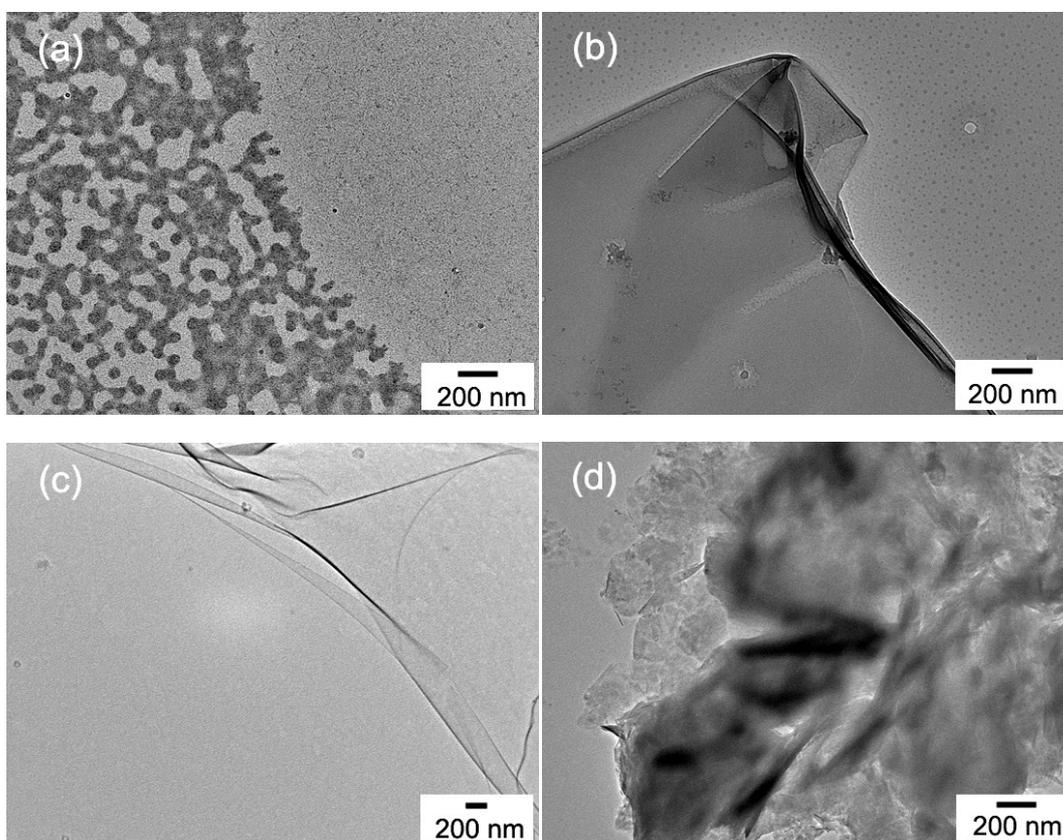
**Fig. S4** TEM images of samples obtained by dissolving PPs in water with polymer concentration of  $1 \text{ mg mL}^{-1}$ , where PPs were prepared with CA/LCy molar ratio being 2:1 at different temperatures for 1 h: (a)  $140 \text{ }^\circ\text{C}$ ; (b)  $150 \text{ }^\circ\text{C}$ ; (c)  $170 \text{ }^\circ\text{C}$ ; (d)  $180 \text{ }^\circ\text{C}$ .
