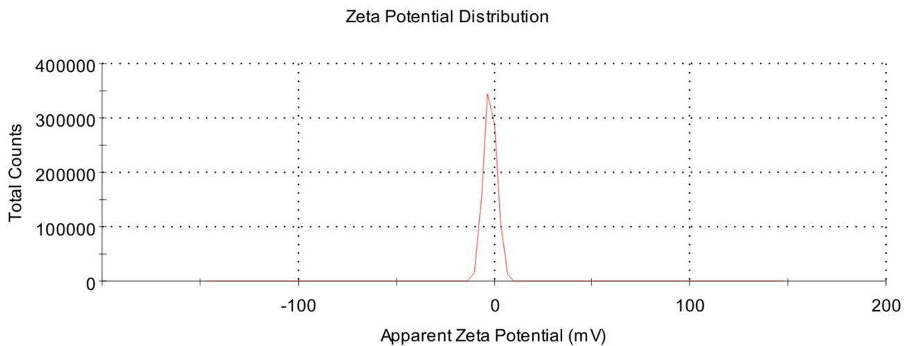
**Fig. S11**  $\zeta$ -Potential plot of PNF aqueous solution with PNF concentration of  $1 \text{ mg mL}^{-1}$ , where PPs were prepared with CA/LCy molar ratio of 2:1 at  $160 \text{ }^\circ\text{C}$  for 1 h.
