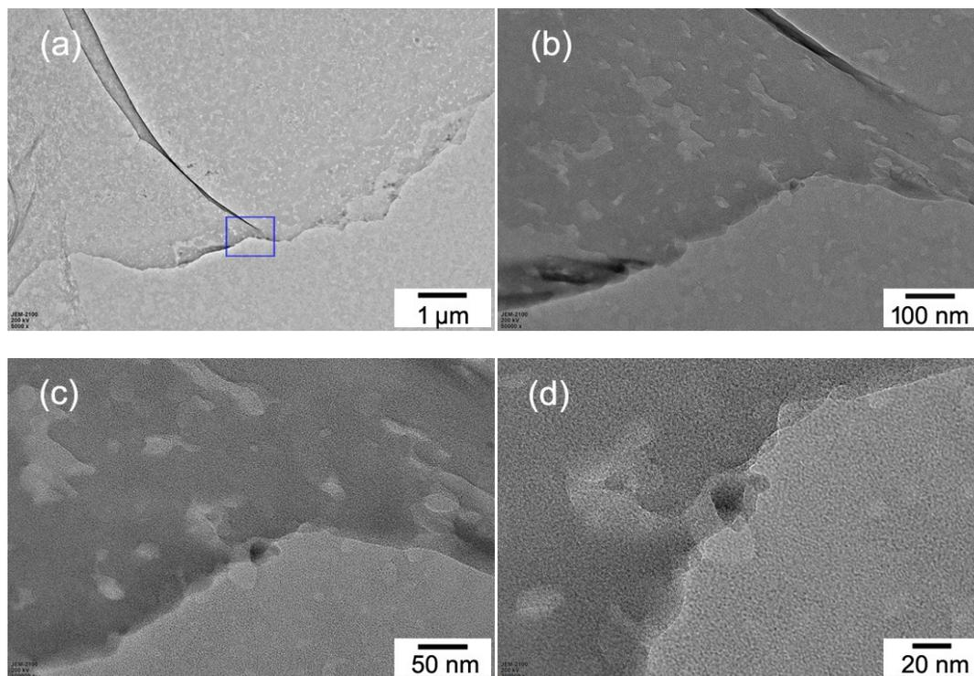
**Fig. S10** TEM images of the sample prepared with CA/LCy molar ratio of 1:1 at 150 °C for 2 h; for TEM observations, the concentration of sample aqueous solution was 1 mg mL<sup>-1</sup>.
