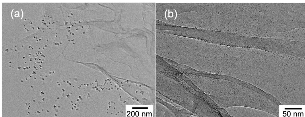
**Fig. S7** TEM images of samples obtained by dissolving PPs in water with polymer concentration of  $1 \text{ mg mL}^{-1}$  but without ultrasonication, where PPs were prepared with CA/LCy molar ratio of 2:1 at  $160 \text{ }^\circ\text{C}$  for 1 h: (a) polymer nanoplates coexist with PNs; (b) CDs residing on PNs.
