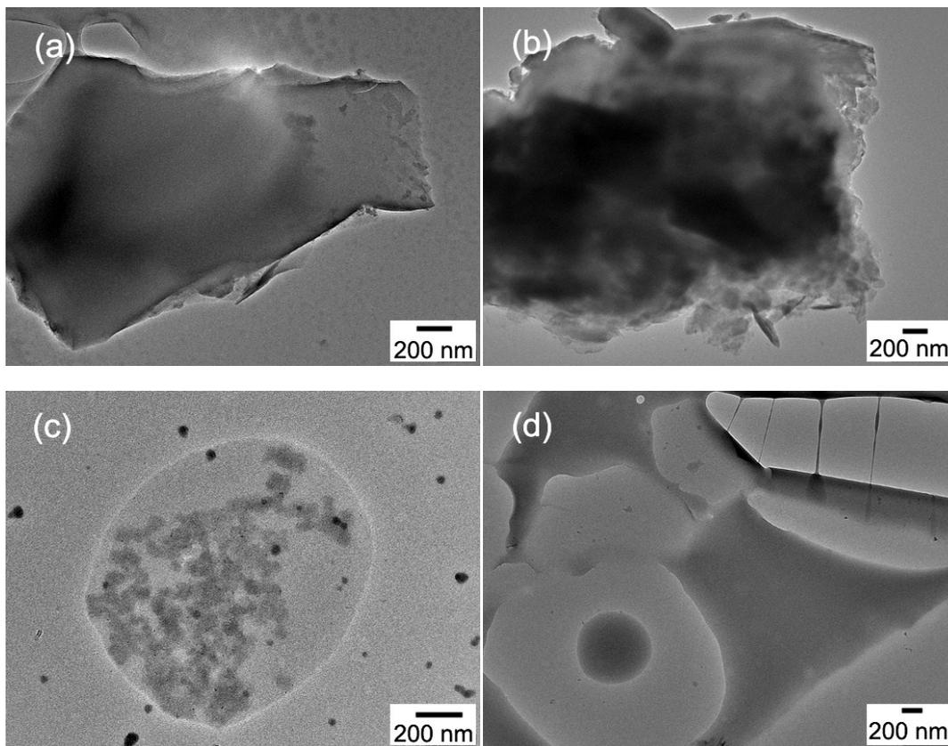
**Fig. S6** TEM images of samples obtained by dissolving PPs in different solvents with polymer concentration of  $1 \text{ mg mL}^{-1}$ , where PPs were prepared with CA/LCy molar ratio of 2:1 at  $160 \text{ }^\circ\text{C}$  for 1 h: (a) absolute ethanol; (b) acetone; (c) tetrahydrofuran; (d) ethyl acetate.
