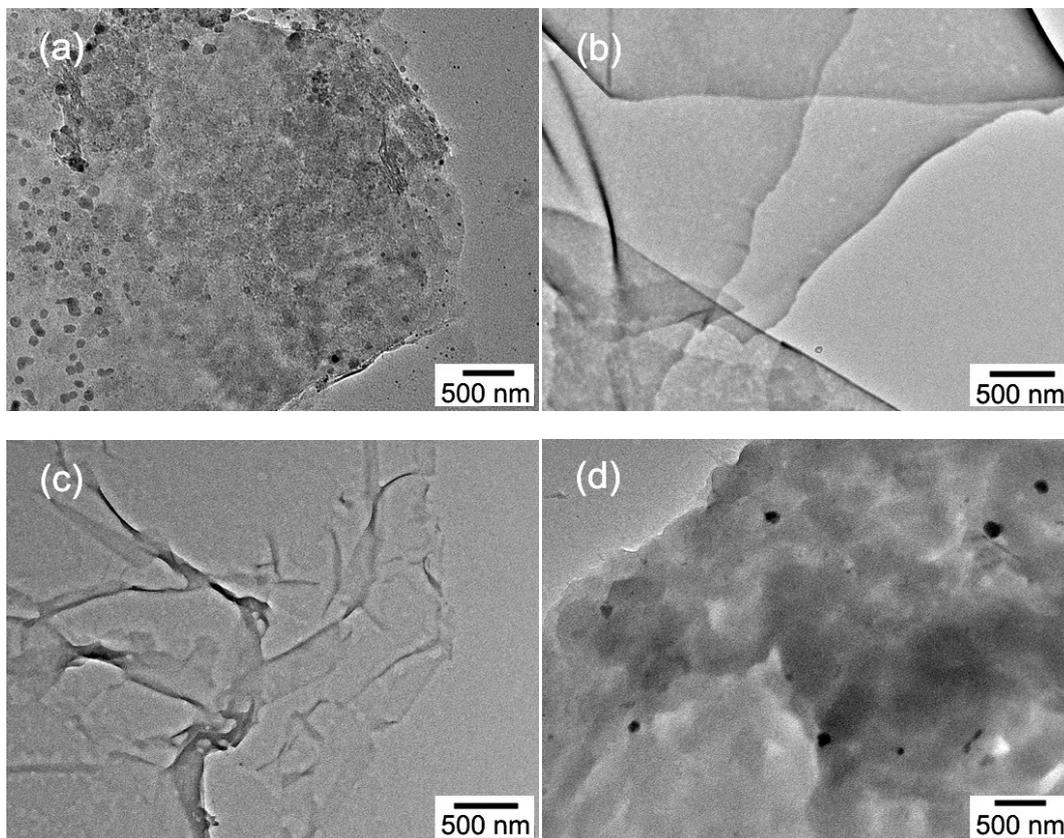
**Fig. S5** TEM images of samples obtained by dissolving PPs in water with polymer concentration of  $1 \text{ mg mL}^{-1}$ , where PPs were prepared with CA/LCy molar ratio being 2:1 at  $160 \text{ }^\circ\text{C}$  for: (a) 0.5 h; (b) 2 h; (c) 4 h; (d) 6 h.
