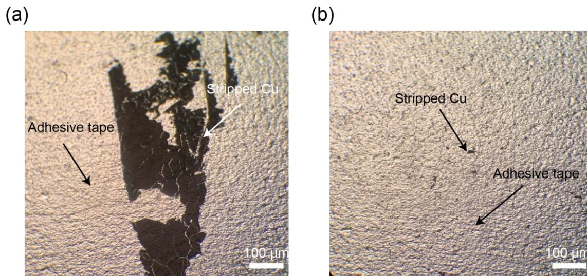
**Figure S7.** Optical microscopy characterizations of the stripped Cu from electroless deposited 'HK' word pattern fabricated on (a) photolithographically patterned conditioned PET substrate with directly deposited PdNPs, and (b) PET substrate with embedded PdNPs through the presented method.
