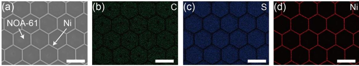
**Figure S2.** Scanning electron microscopy (SEM) and energy-dispersive X-ray spectroscopy (EDS) analysis for a Ni mold before SACN process. (a) The SEM image with corresponding elemental mappings for (b) carbon, (c) sulfur, and (d) nickel. The scale bars represent 50  $\mu\text{m}$ .
