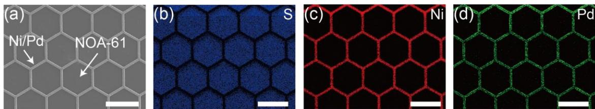
**Figure S3.** SEM and EDS analysis for a SACN-mold. (a) The SEM image with corresponding elemental mappings for (b) sulfur, (c) nickel, and (d) palladium. The scale bars represent 50  $\mu\text{m}$ .
