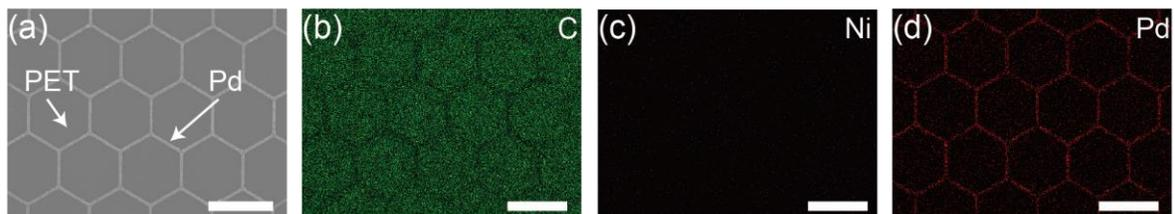
**Figure S5.** SEM and EDS analysis for the typical imprint-transferred PdNPs on a polyethylene terephthalate (PET) film. (a) The SEM image with corresponding elemental mappings for (b) carbon, (c) nickel and (d) palladium. The scale bars represent 50  $\mu\text{m}$ .
