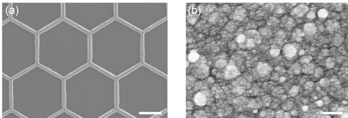
**Figure S4.** (a) SEM images of a SACN-mold and (b) zoom-in image showing the morphology of the adsorbed PdNPs. The scale bars represent 20  $\mu\text{m}$  in (a) and 100 nm in (b).
