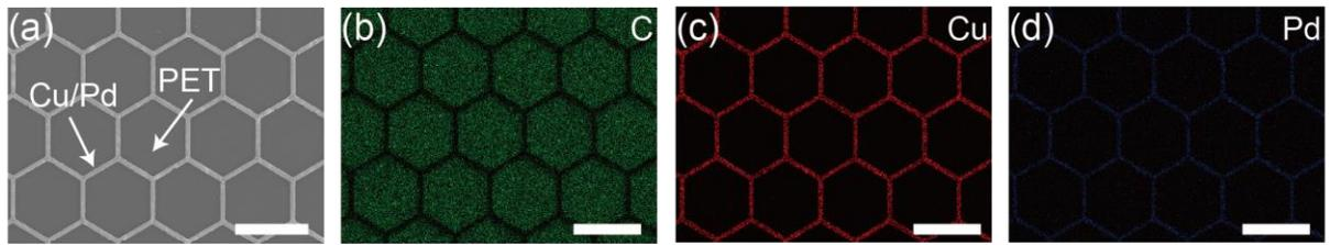
**Figure S6.** SEM and EDS analysis for a Cu TE. (a) The SEM image with corresponding elemental mappings for (b) carbon, (c) copper, and (d) palladium. The scale bars represent 50  $\mu\text{m}$ .
