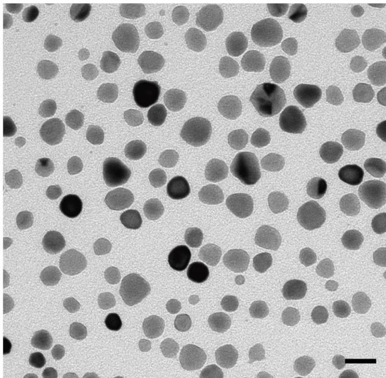
**Figure S1.** Tunneling electron microscopy (TEM) image of the catalytic palladium nanoparticles (PdNPs). The scale bar represents 20 nm. Reproduced with permission.<sup>1</sup> Copyright 2018, American Chemical Society.
