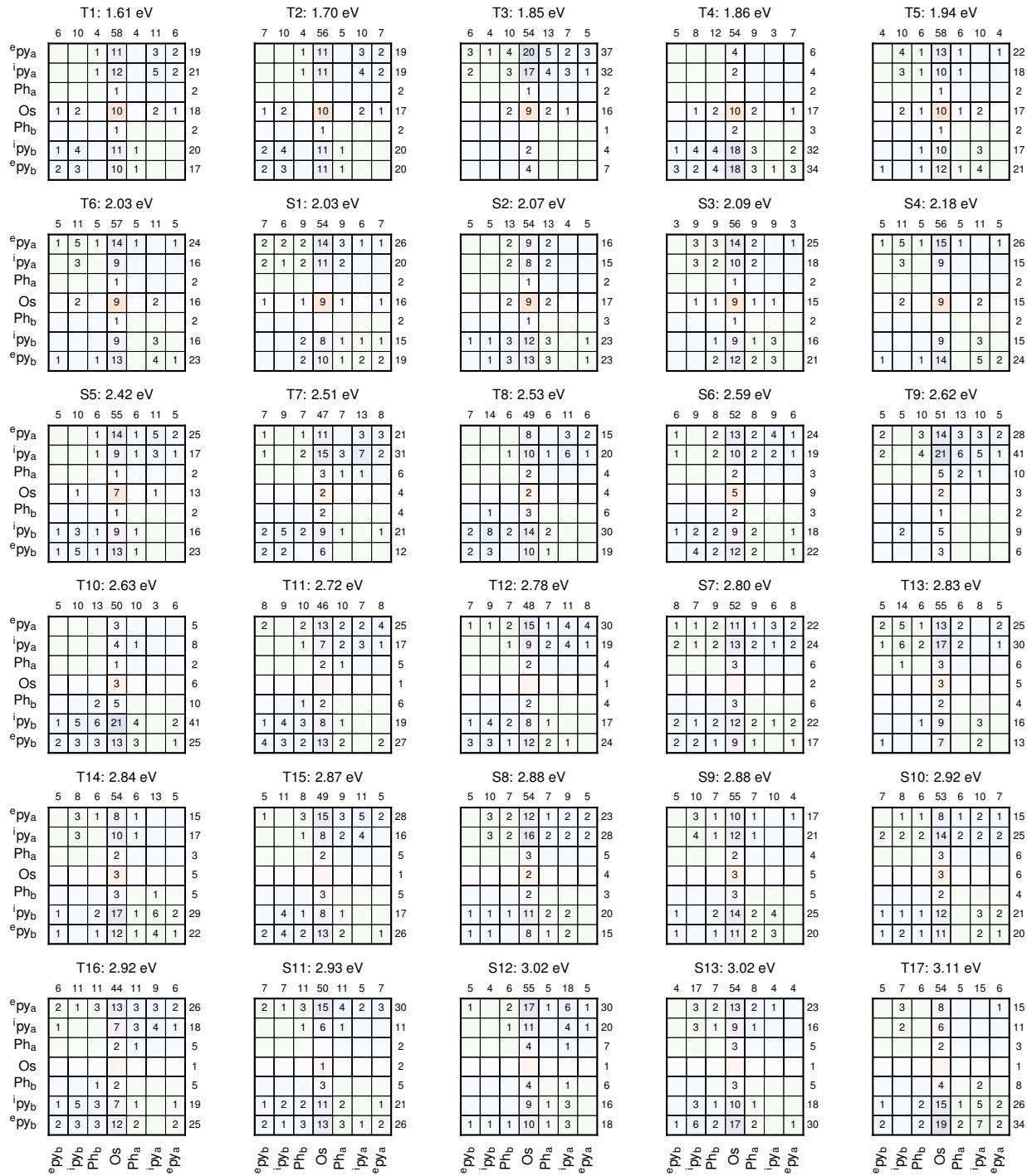
**Figure 5: Electron-hole correlation plots for the first 30 excited states of 1-Os calculated with LR-TDDFT/1C-X2C-PBE0/x2c-SV(P)all/COSMO(CH<sub>2</sub>Cl<sub>2</sub>). See text for a detailed explanation of how to read the diagrams.**
