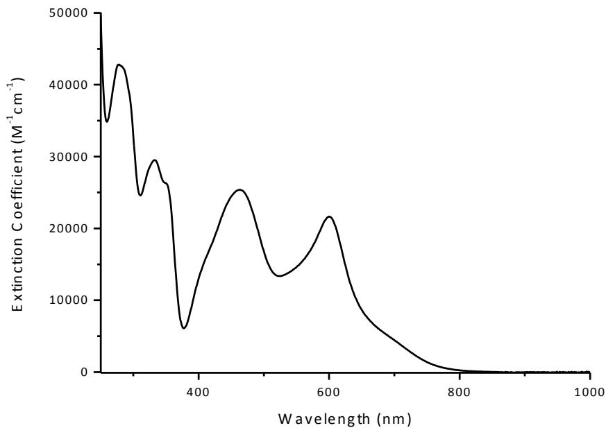
**Figure 1:** Absorption spectrum of 1-Ru recorded in  $\text{CH}_2\text{Cl}_2$  at rt.
