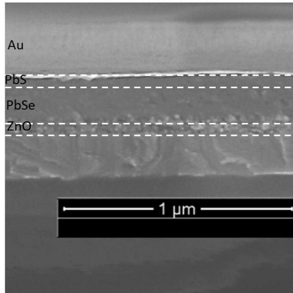
Figure S1. Scanning electron microscopy image of complete device of 5% PbSe mixing solar cell
