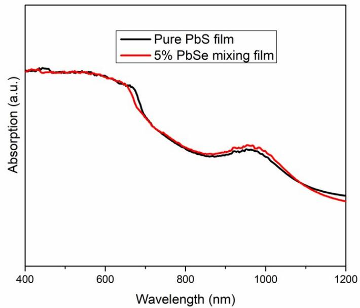
Figure S2. The UV-VIS absorption curves of pure PbS and 5% PbSe mixed films.
