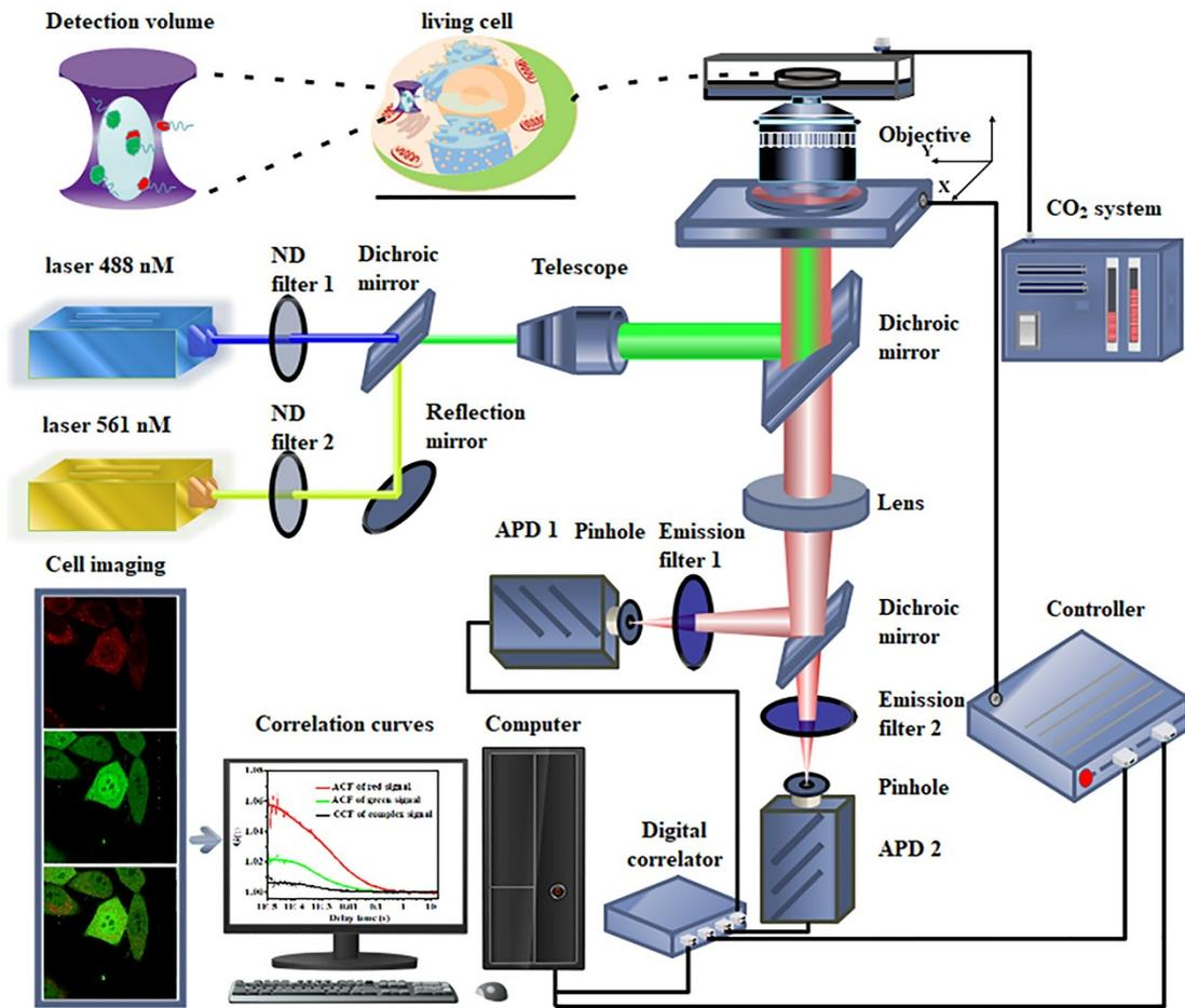
**FigureS1.** Schematic diagram of FCS and FCCS setup.
